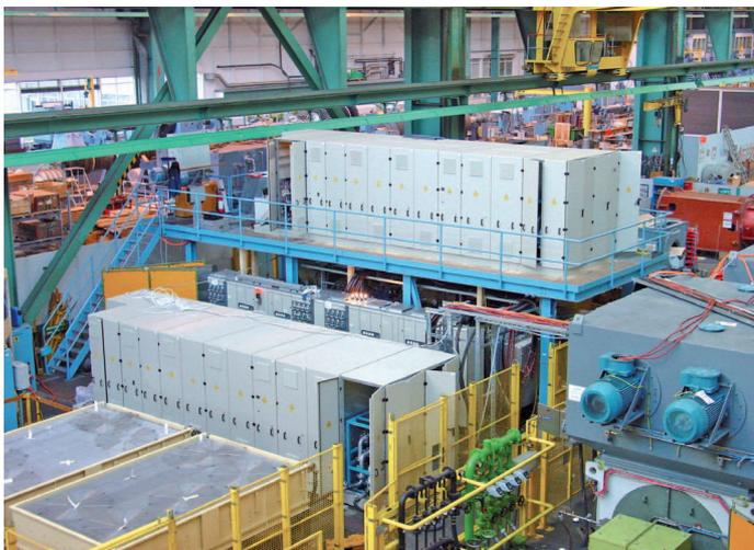
Back-to-back test 8 MW / 3,600 rpm
