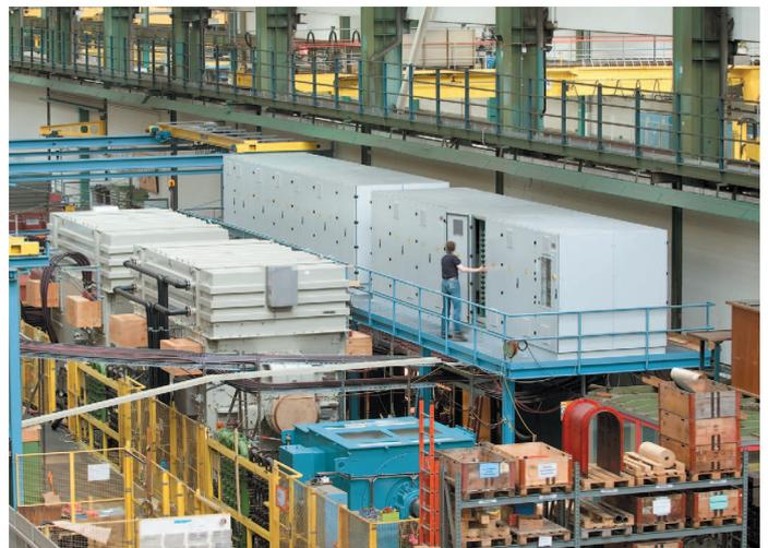
Back-to-back test 48 MW / 3,500 rpm
