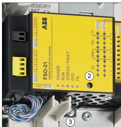
4. Make sure that the FSO data cable (terminal X110) is connected to the drive. Use only the cable delivered with the module.
