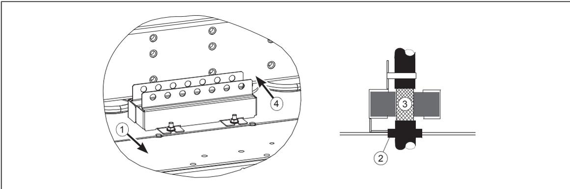
**Note 1:** Keep the shields continuous as close to the connection terminals as possible. Secure the cables mechanically at the entry strain relief.
