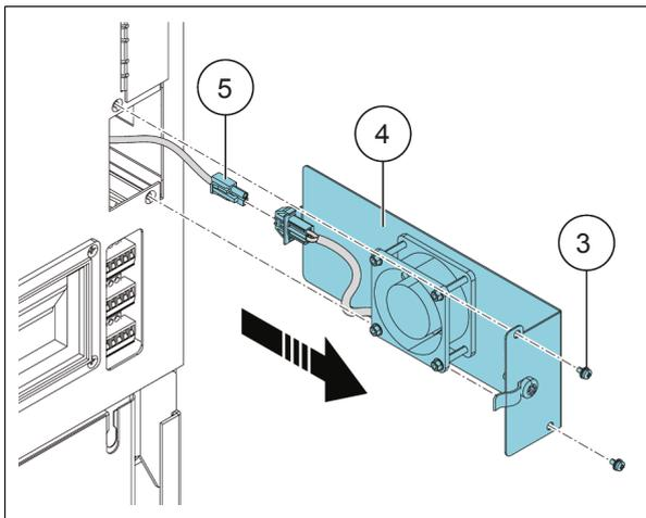
6. Remove the four M3 (5.5 mm) nuts which hold the fan.
