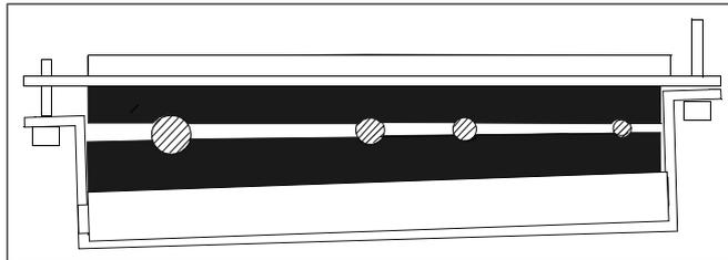
6. If more than one cable go through a grommet, seal the grommet by applying Loctite 5221 (catalogue number 25551) inside the grommet.
