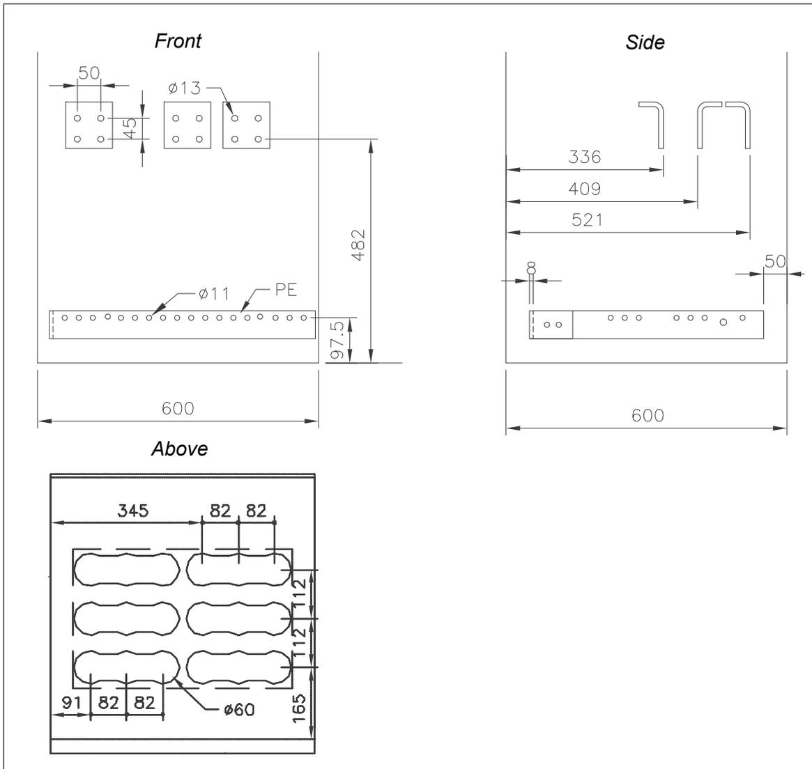
■ **600 mm incoming cubicle – main breaker (+F255), bottom cable entry, 12-pulse (+A004)**
