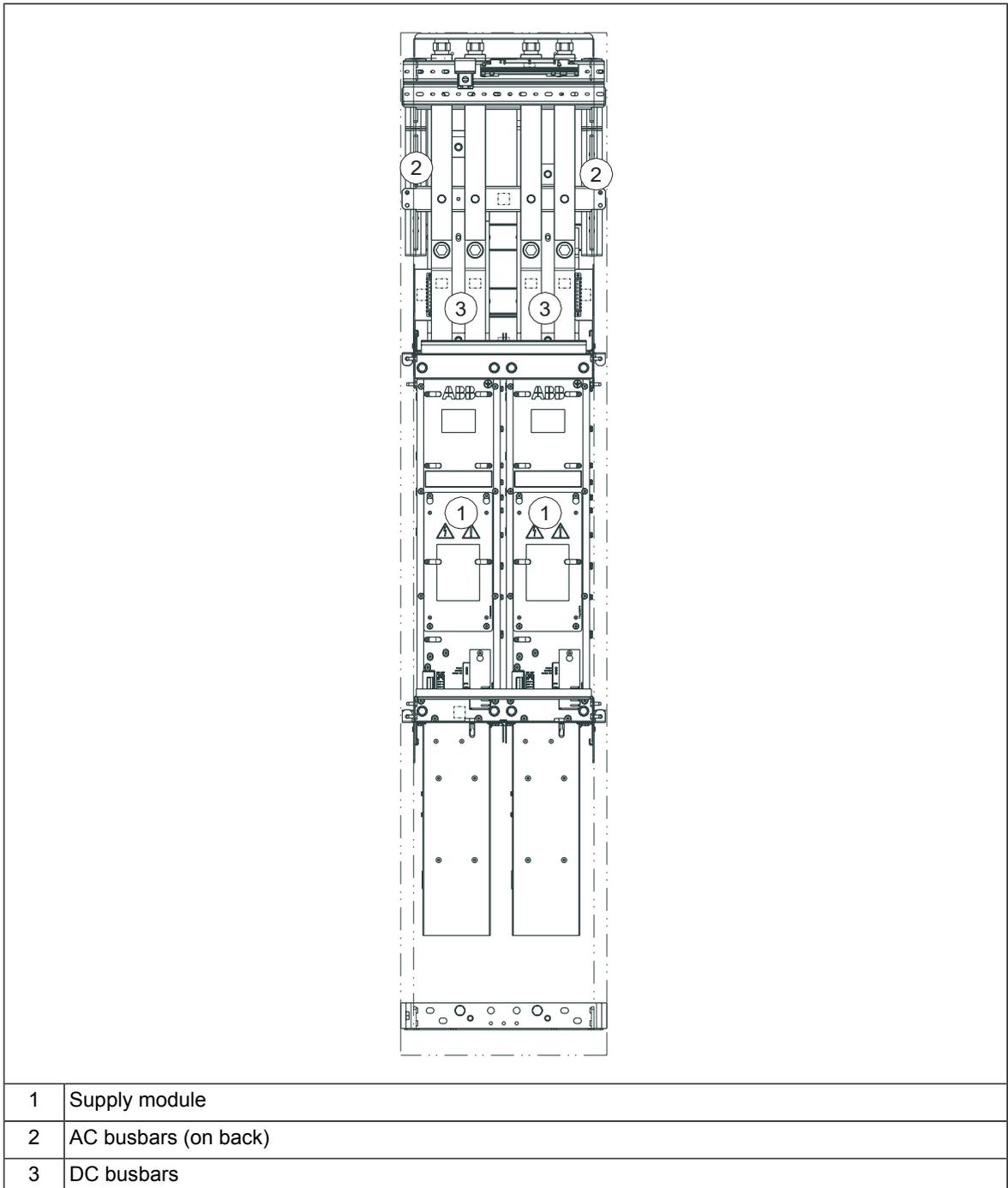
■ **Layout drawing of a supply module cubicle 1×D8T**
