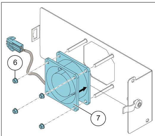
8. Put the fan onto the threaded studs on the fan holder with the airflow direction arrow pointing towards the fan holder.
