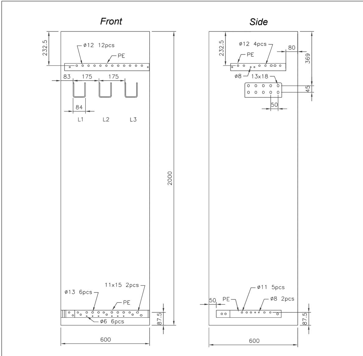
■ **1000 mm incoming cubicle – main breaker (+F255), bottom cable entry**
