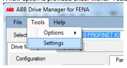
If user is trying to connect to Siemens PLC via VPN connection and the FENA adapter version is 3.03 or later then this option has to be selected.
