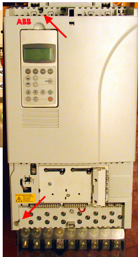
Figure 7.3: RFI earthing screws in the frame R6.
