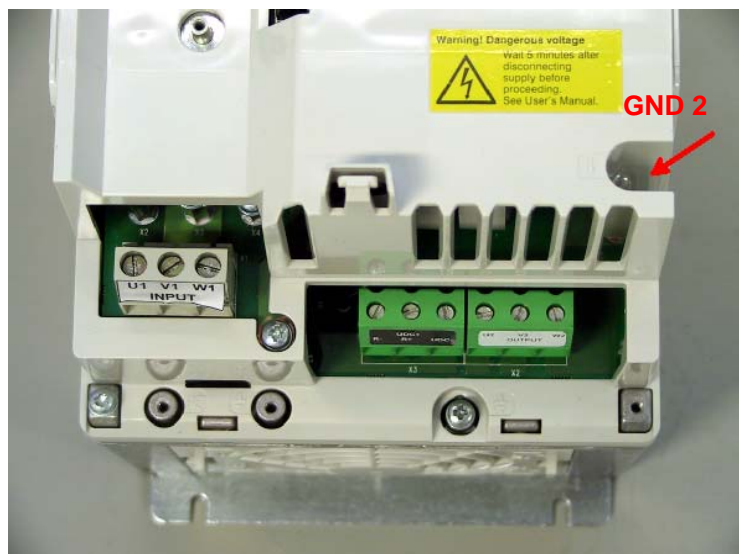
Figure 4.3: Earthing screw GND2 of the EMC capacitors in ACS800-01 frame size R3.
