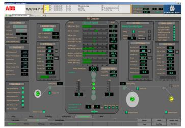
All automation panels and all control cables were reused reducing shutdown time and cost for the customer. ABB also offered a DCS800 rebuild kit solution to upgrade existing drives and reused all electrical components, including drives power and control cables. A special adapter plate was also prepared to replace the force motor valve with moog servo valve. This arrangement enabled the replacement of valves with minimal changes in the hydraulic system.
