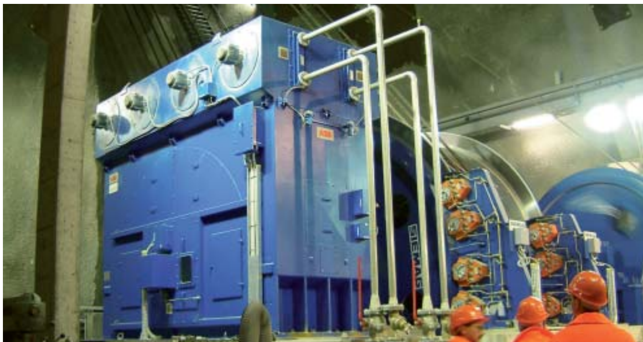
The 4,176 kW synchronous motor for the cage hoist
