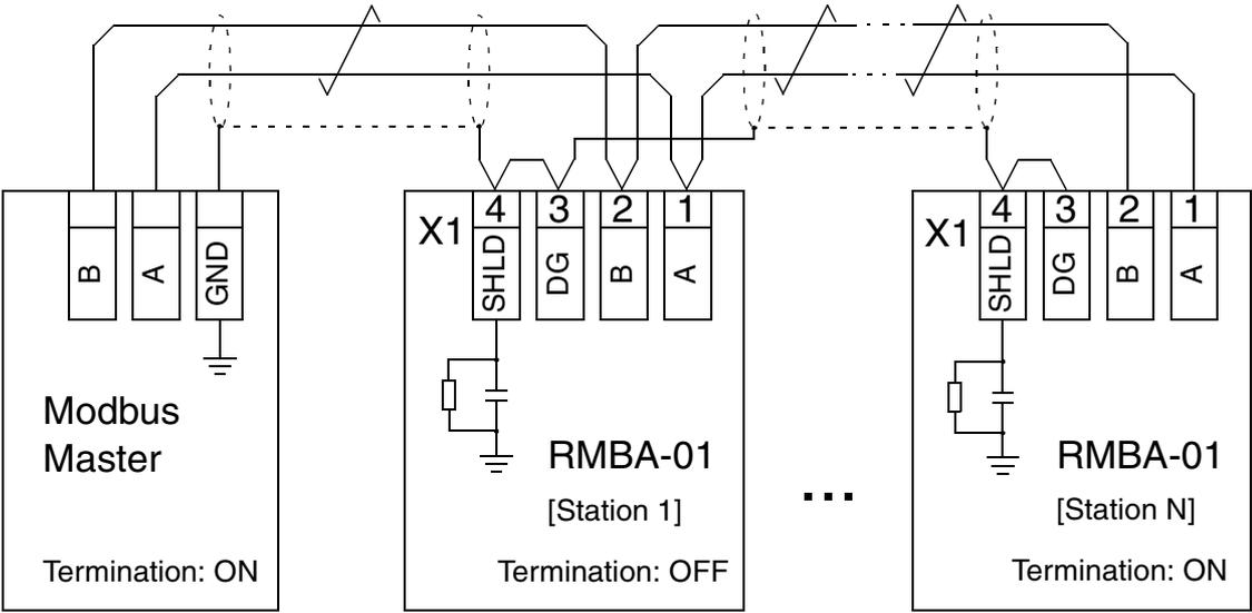
Figure 3-2 Two-wire connection
