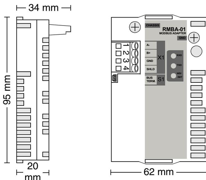
**Mounting:** Into an option slot of the RMIO board of the drive or onto external I/O Module Adapter (AIMA-01).
