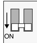
Figure 3-4 Bus termination switch (S1)
