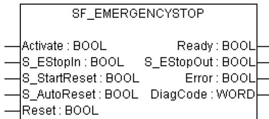
This function block is a safety-related function block for monitoring an emergency stop button. This FB can be used for emergency switch off functionality (stop category 0), or – with additional peripheral support – as emergency stop (stop category 1 or 2).
