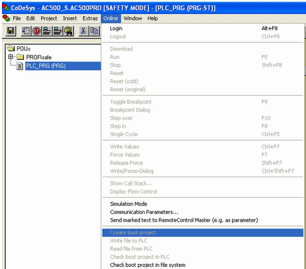
Fig. 95: Create boot project for SM560-S Safety CPU
