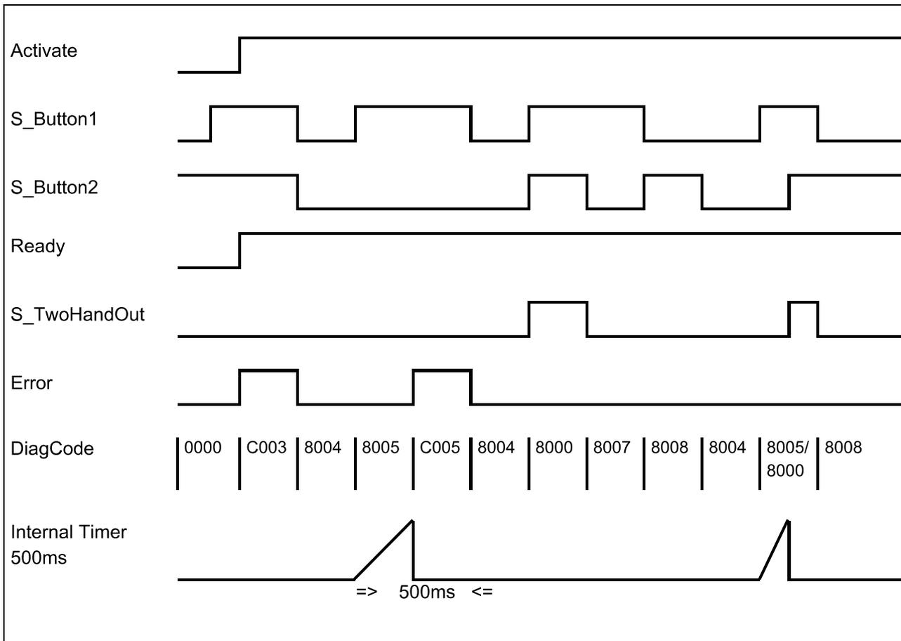
Fig. 111: Timing diagram for SF\_TwoHandControlTypeIII
