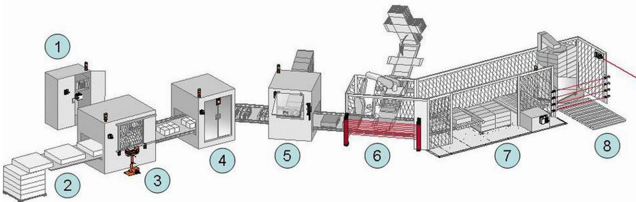
Fig. 133: Example of safety functionalities in a production line
