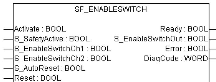
The SF\_EnableSwitch FB evaluates the signals of an enable switch with three positions.
