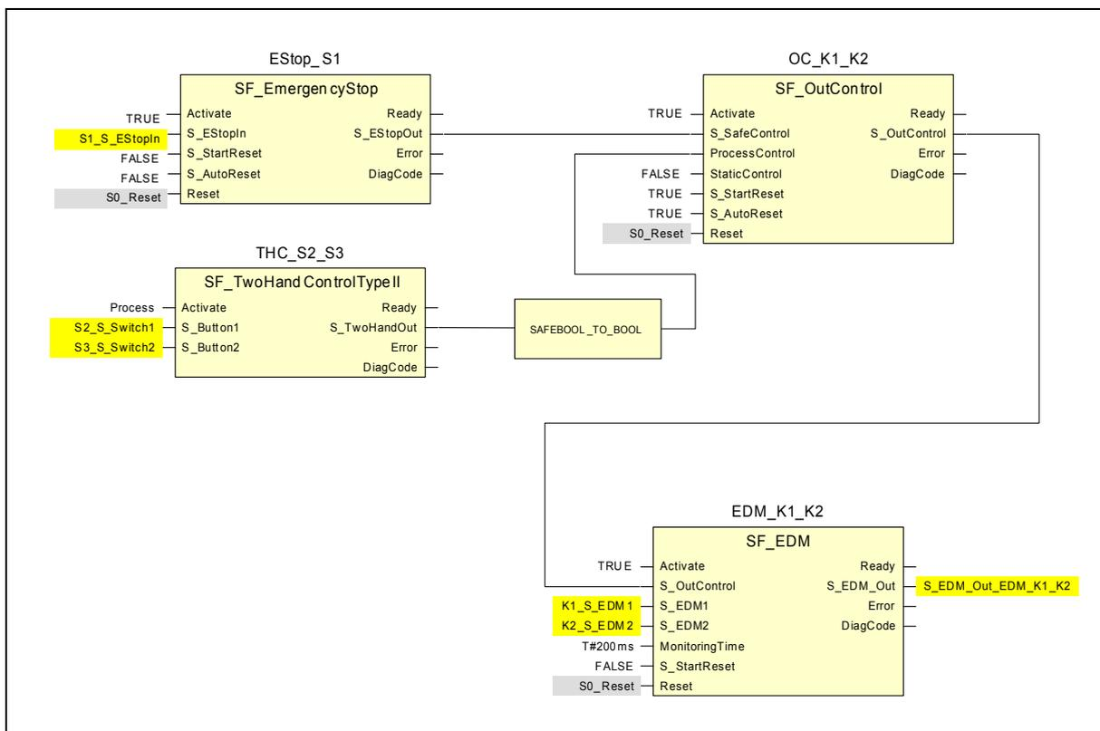
Fig. 140: Application Program TwoHand Control with EDM
