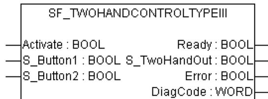
This function block provides the two-hand control functionality (see EN 574, Section 4 Type III. Fixed specified time difference is 500 ms).
