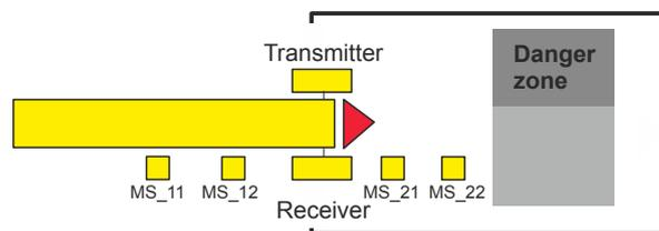
Muting mode remains active as long as MutingSwitch11 (MS\_11) and MutingSwitch12 (MS\_12) are activated by the product. The product may pass through the light curtain without causing a machine stop.
