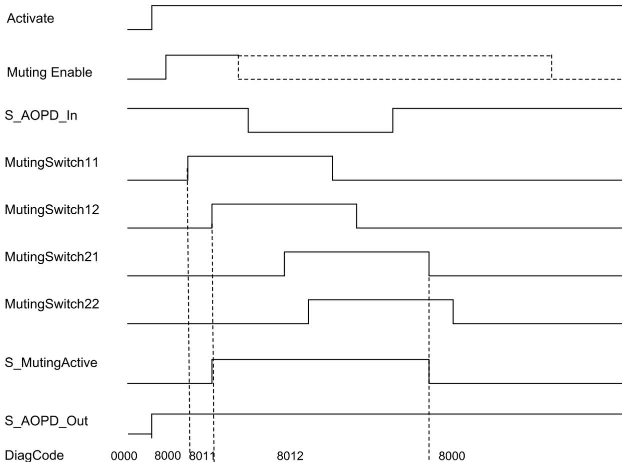
Fig. 114: Timing diagram for SF\_MutingSeq with S\_StartReset = TRUE
