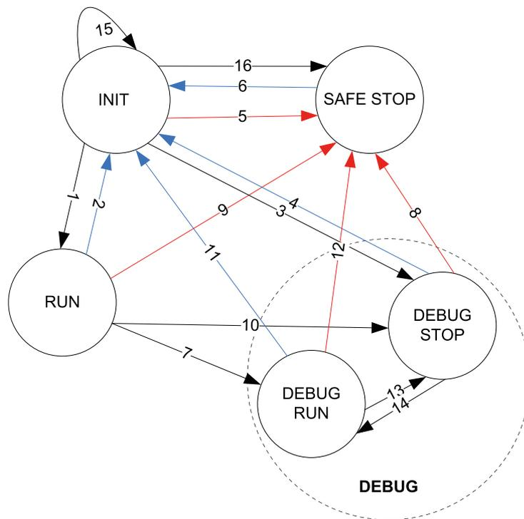
Fig. 11: SM560-S Safety CPU module states and transitions
