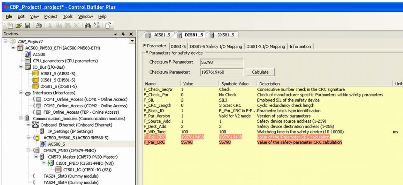
The screenshot shows the 'F-Parameter' configuration window in Control Builder Plus. The window is titled 'F-Parameter' and has tabs for 'DI581-S', 'DI581-S Safety I/O Mapping', 'DI581-S I/O Mapping', and 'Information'. The 'Information' tab is active, showing a table of F-Parameters for a safety device. The table has columns for Name, Value, Symbolic-Value, Description, and Unit. The values for 'F\_Par\_CRC' and 'F\_Par\_CRC' are highlighted in red.
