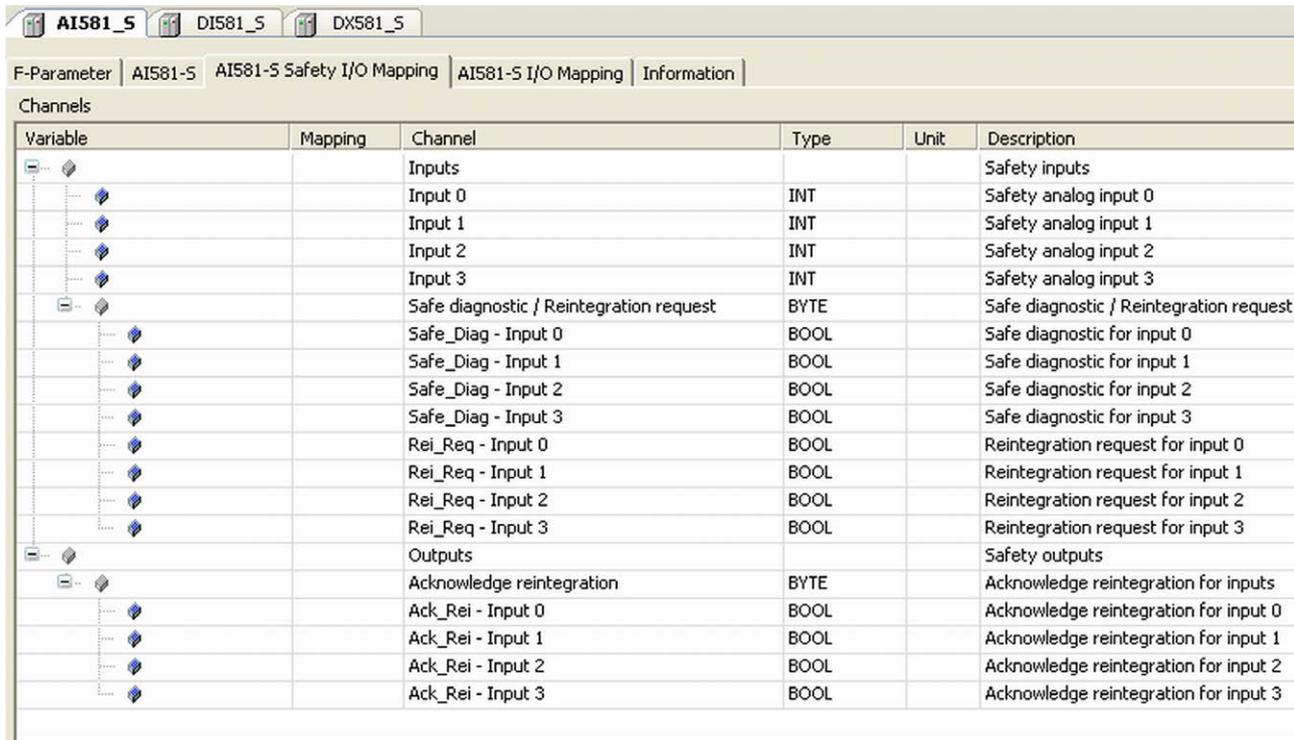
The screenshot shows the configuration interface for the AI581-S module. The 'Channels' section is expanded, displaying a table of variable mappings. The table has columns for Variable, Mapping, Channel, Type, Unit, and Description. The variables are grouped into Inputs, Safe diagnostic / Reintegration request, and Outputs.
