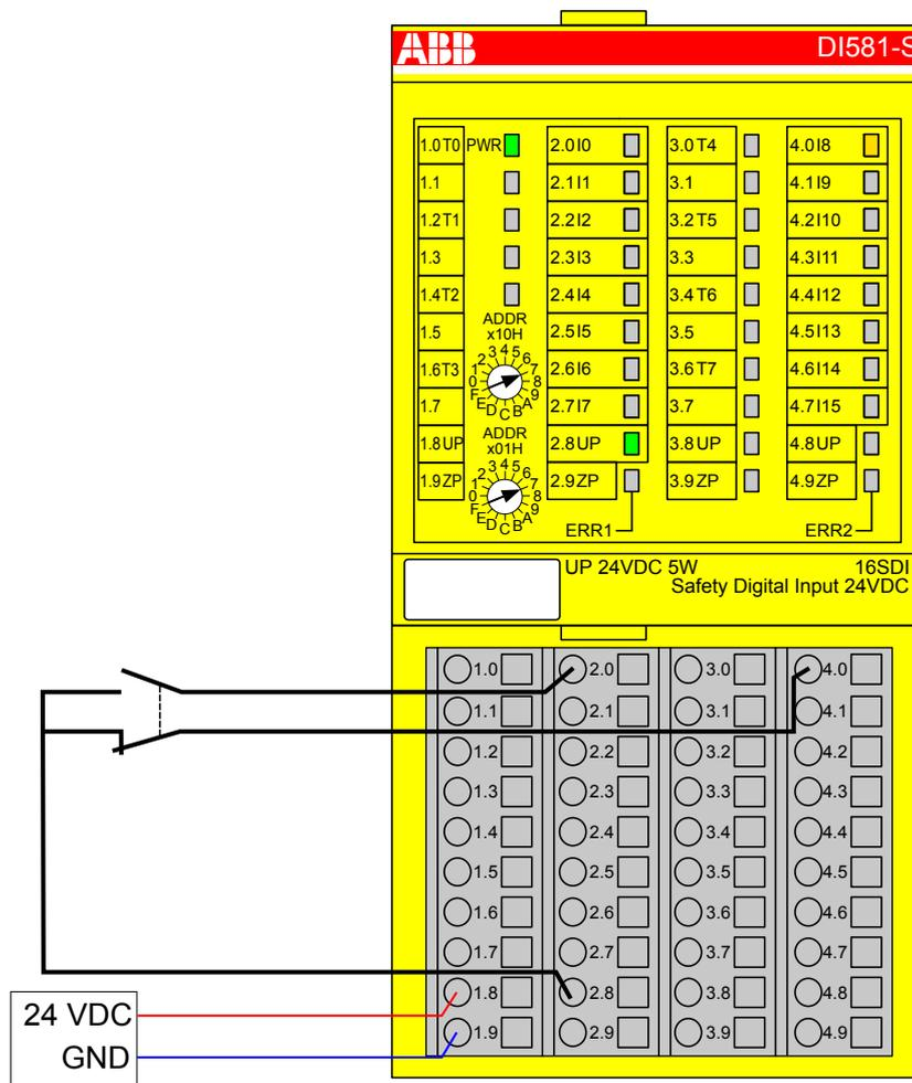
Fig. 27: Circuit example DI581-S, 2-channel sensor (antivalent), 24 V DC
