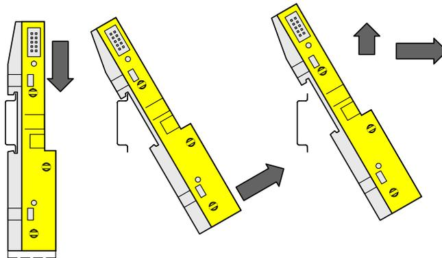
2. ➤ Pull down the Terminal Unit and remove it.
