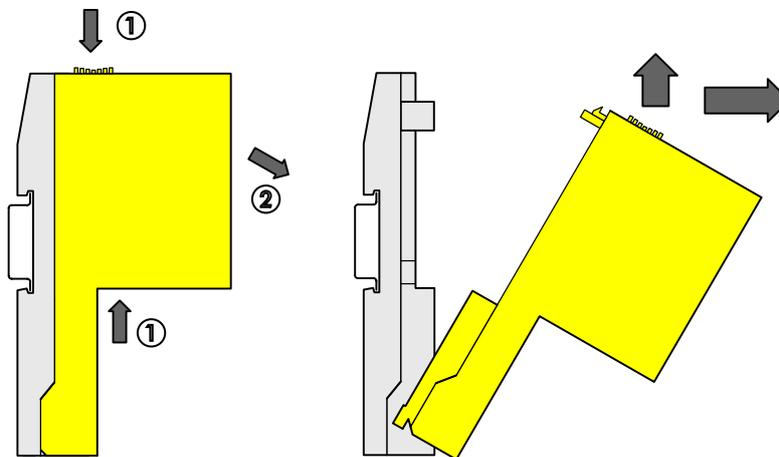
Fig. 7: Disassembly instructions
