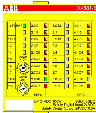
Safety binary input/output module DX581-S with 8 safety output channels (up to SIL3 or PL e) and 8 safety input channels (up to SIL2 or PL d) or 4 safety input channels (up to SIL3 or PL e) with 4 test pulse output channels.
