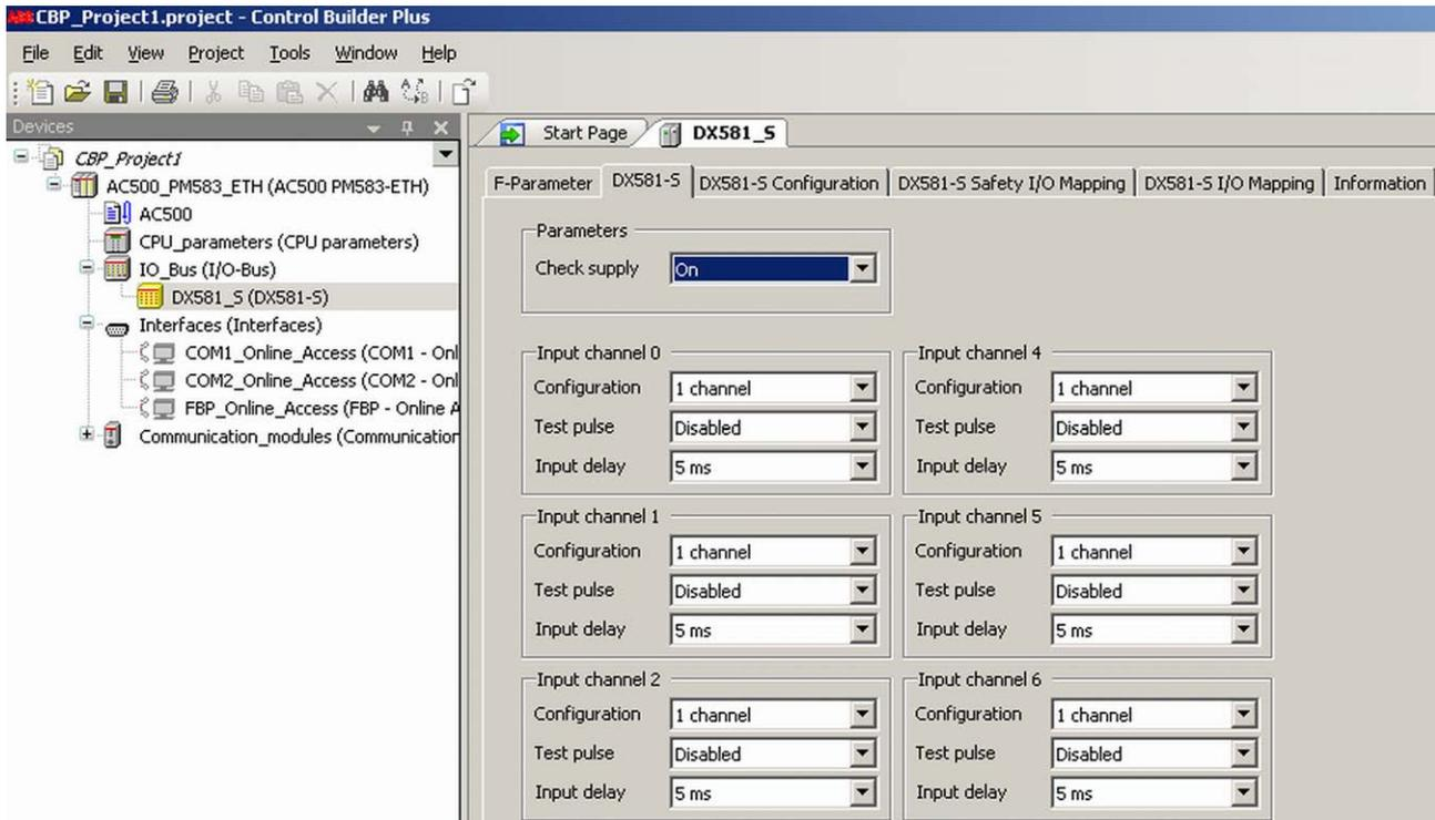
3. Verify against your safety application technical specification that all iParameters for all Safety I/O channels are set correctly.
