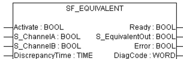
This function block converts two equivalent BOOL inputs (both NO or NC) to one BOOL output, including discrepancy time monitoring. This FB should not be used stand-alone since it has no restart interlock. It is required to connect the output to other safety related functionalities.
