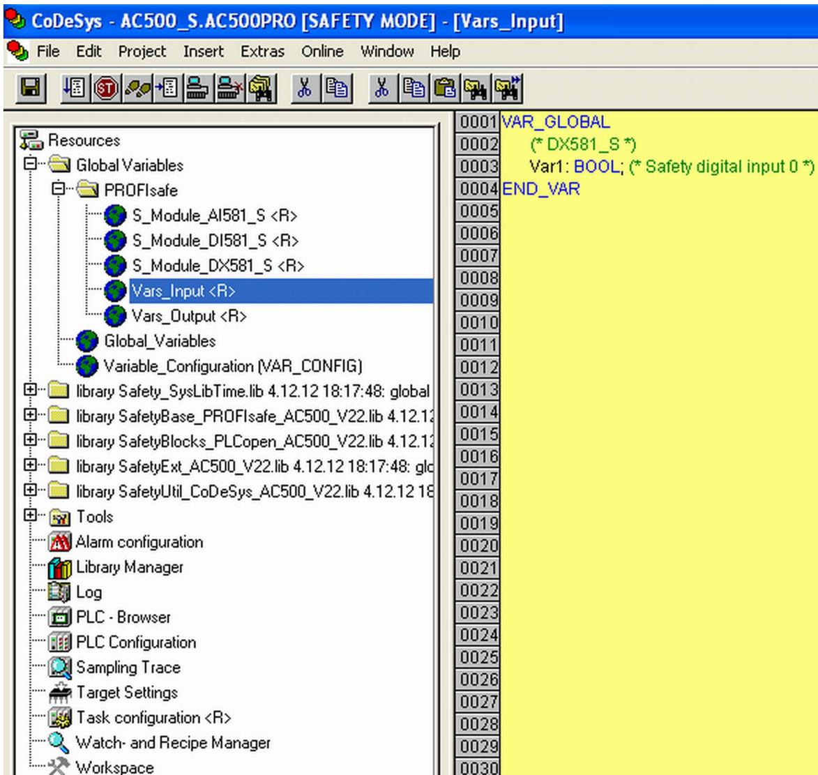
Fig. 88: Global variable list in CoDeSys Safety V2.3
