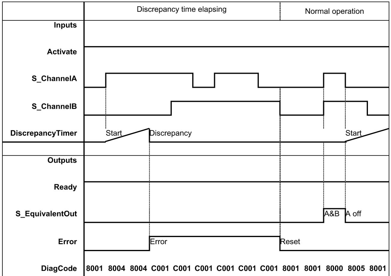
Fig. 98: Typical Timing Diagram for SF\_Equivalent
