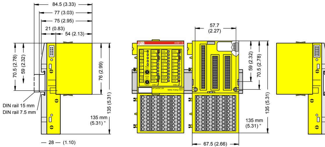
Fig. 52: Dimensions of AI581-S Safety I/O module
