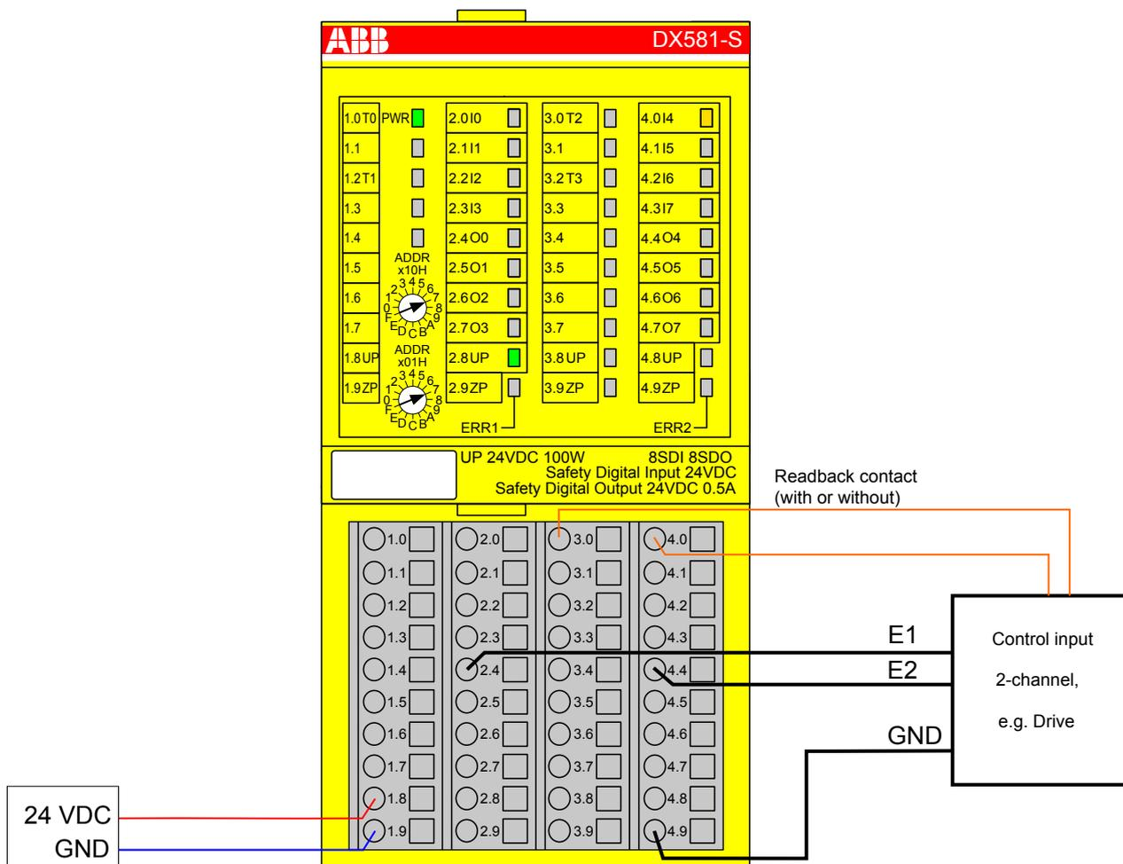
Fig. 47: Circuit example DX581-S, Transistor input (2-channel)
