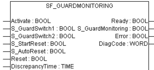
This function block monitors the relevant safety guard. There are two independent input parameters for two switches at the safety guard coupled with a time difference (MonitoringTime) for closing the guard.
