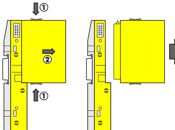
Fig. 40: Disassembly instructions
