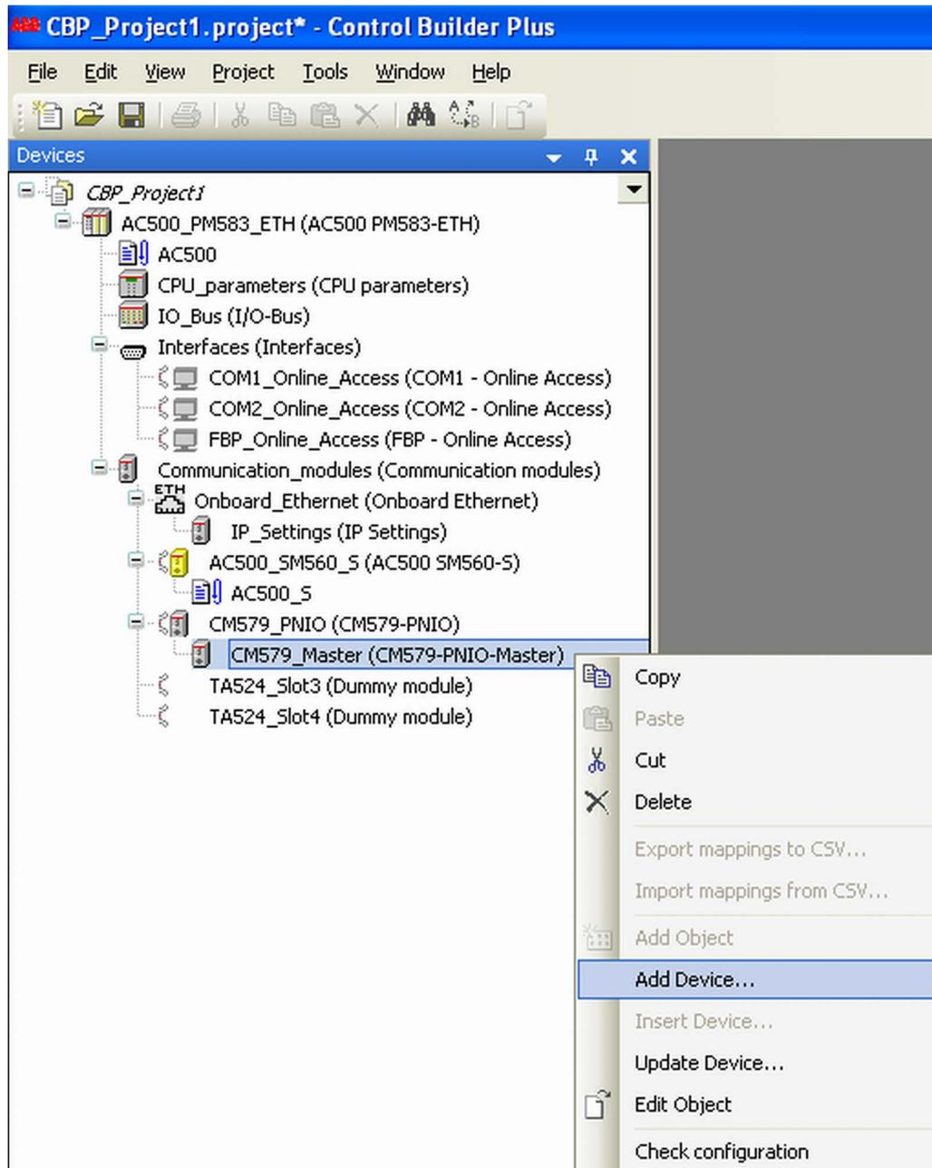
Fig. 77: Select module and open “Add Device menu ...”
