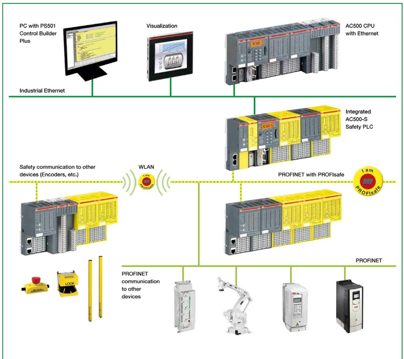
Fig. 4: AC500-S system setup with PROFINET / PROFIsafe
