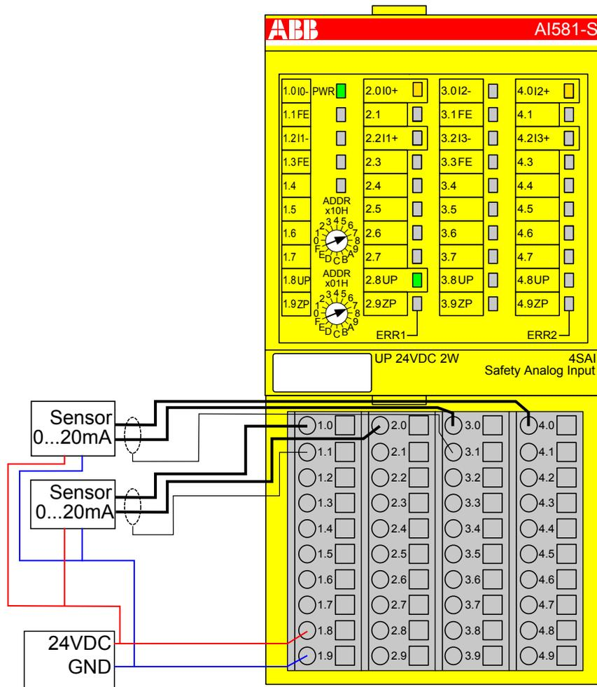
Fig. 56: Circuit example AI581-S, 2 analog sensors (0 ... 20 mA)
