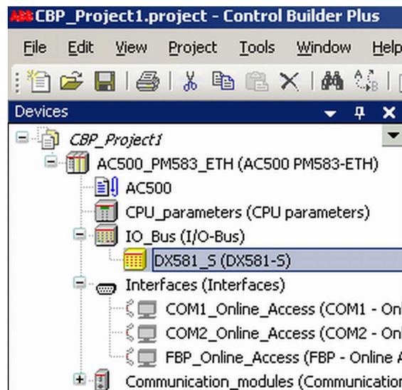
2. → Go to the iParameter setting tab (DX581-S, DI581-S or AI581-S respectively) for the given module and set appropriate iParameter values (e.g., "Test Pulse", "Input Delay", etc.).
