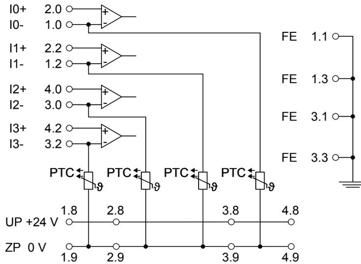
Fig. 53: Example of electrical connections with AI581-S
