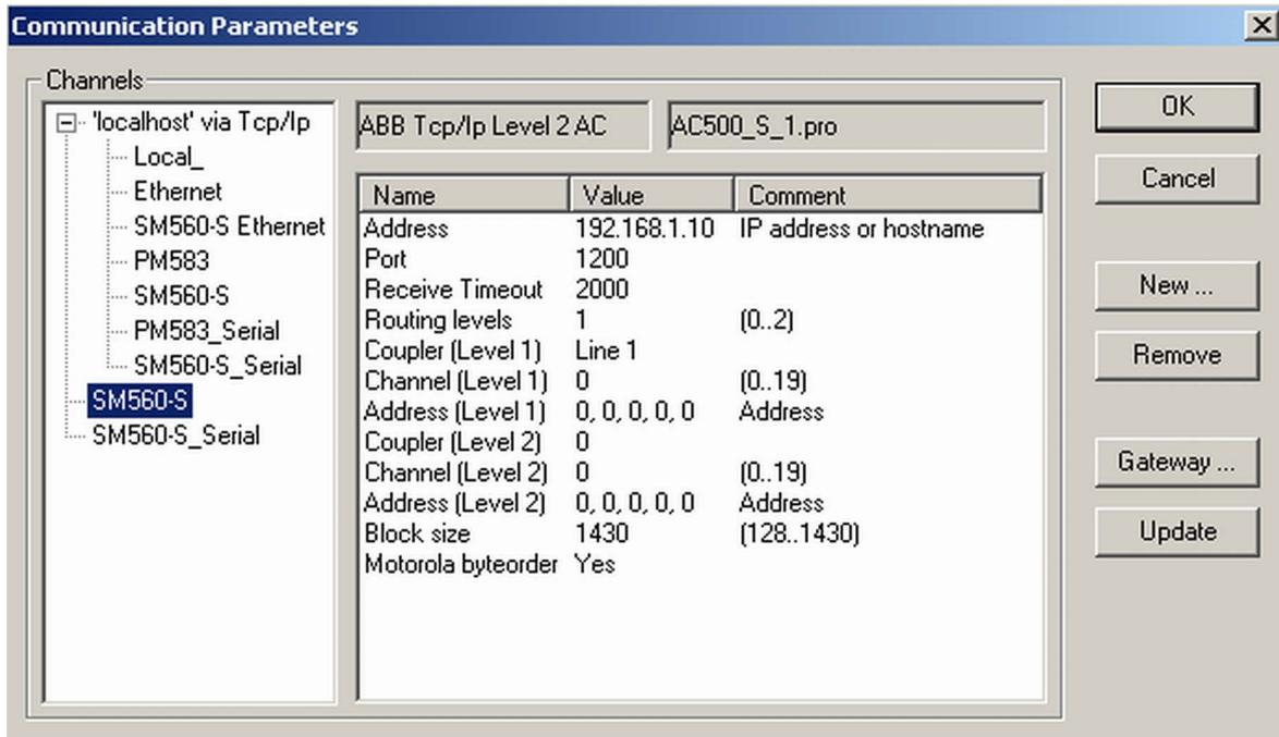
Fig. 93: Example with Ethernet connection
