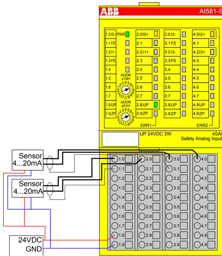
Fig. 58: Circuit example AI581-S, 2 analog sensors (4 ... 20 mA)
