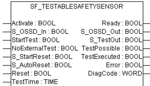
This function block detects, for example, the loss of the sensing unit detection capability, the response time exceeding that specified, and static ON signal in single-channel sensor systems. It can be used for external testable safety sensors (ESPE: Electro-sensitive protective equipment, such as a light beam).
