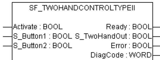
This function block provides the two-hand control functionality (☞ *EN 574, Section 4 Type II*).
