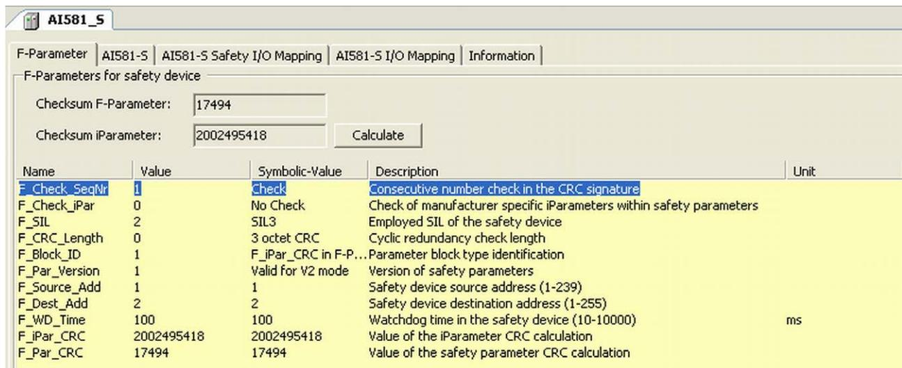
The screenshot shows the configuration window for AI581-S. It has tabs for 'F-Parameter', 'AI581-S', 'AI581-S Safety I/O Mapping', 'AI581-S I/O Mapping', and 'Information'. Under 'F-Parameters for safety device', there are input fields for 'Checksum F-Parameter' (17494) and 'Checksum iParameter' (2002495418), with a 'Calculate' button. Below is a table of parameters:
