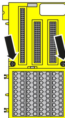
**2.** Fasten Terminal Unit with 2 M4 screws (max. 1.2 Nm).
