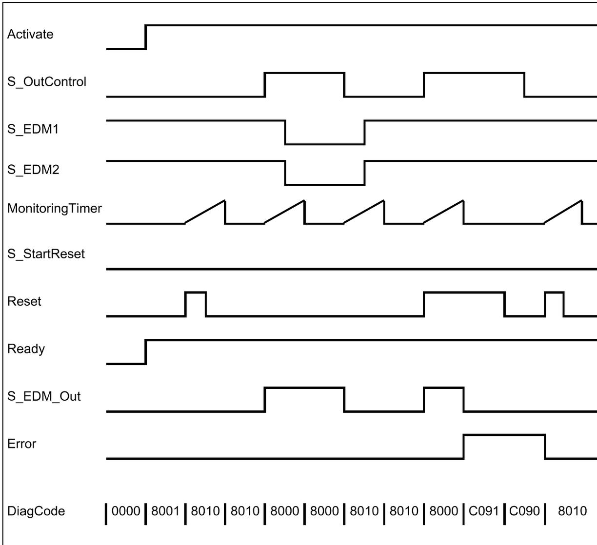
Fig. 124: Timing diagrams for SF\_EDM: S\_StartReset = FALSE
