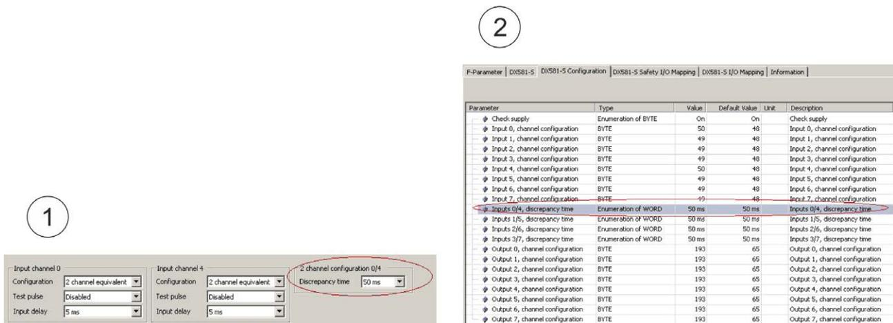
Fig. 132: Compare “DX581-S” tab and “DX581-S Configuration” tab
