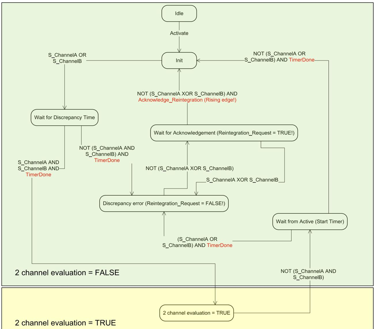
Fig. 17: 2 channel equivalent mode implemented in DI581-S
