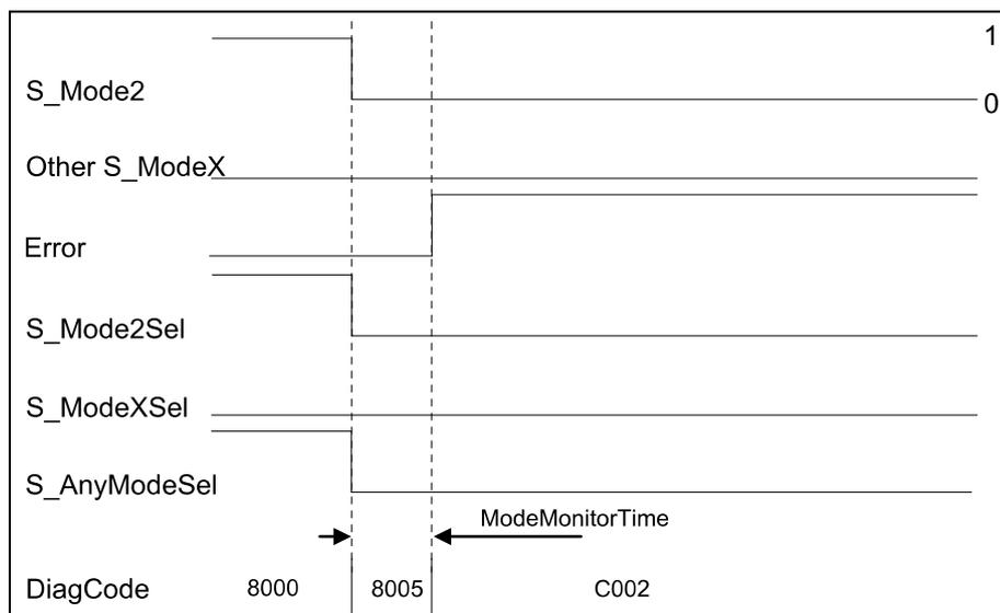
Fig. 101: Timing diagram for SF\_ModeSelector, error condition 2 at Mode inputs
