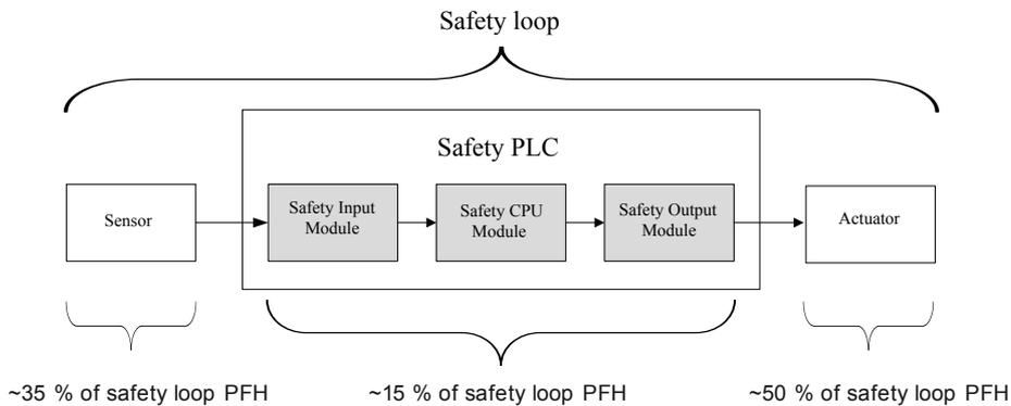
Fig. 3: Typical safety loop with AC500-S Safety PLC
