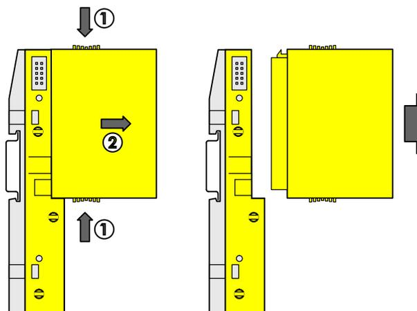
Fig. 51: Disassembly instructions
