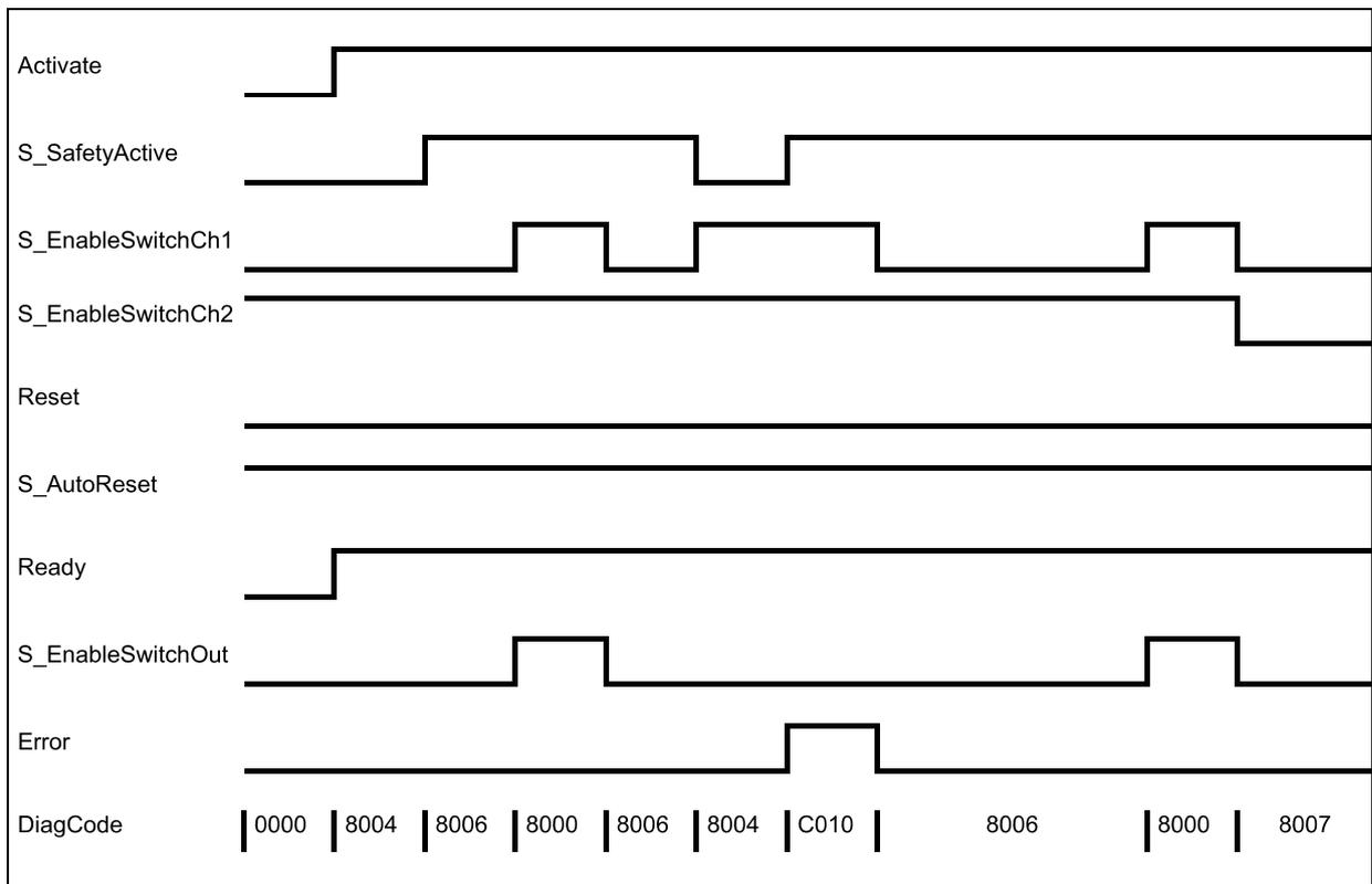
Fig. 119: Timing diagram for SF\_EnableSwitch: S\_AutoReset = TRUE
