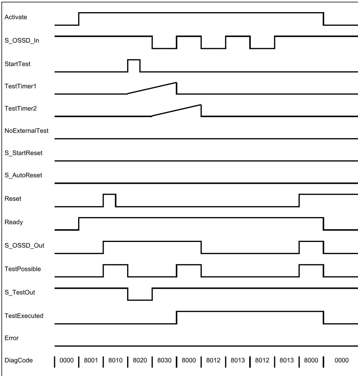
Fig. 113: Timing diagram for SF\_TestableSafetySensor
