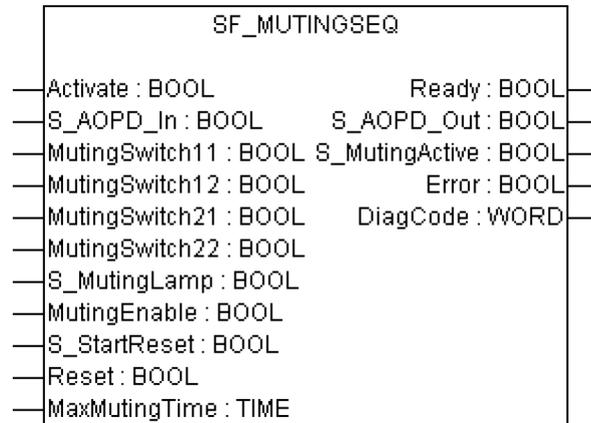
Muting is the intended suppression of the safety function (e.g., light barriers). In this FB, sequential muting with four muting sensors is specified.
