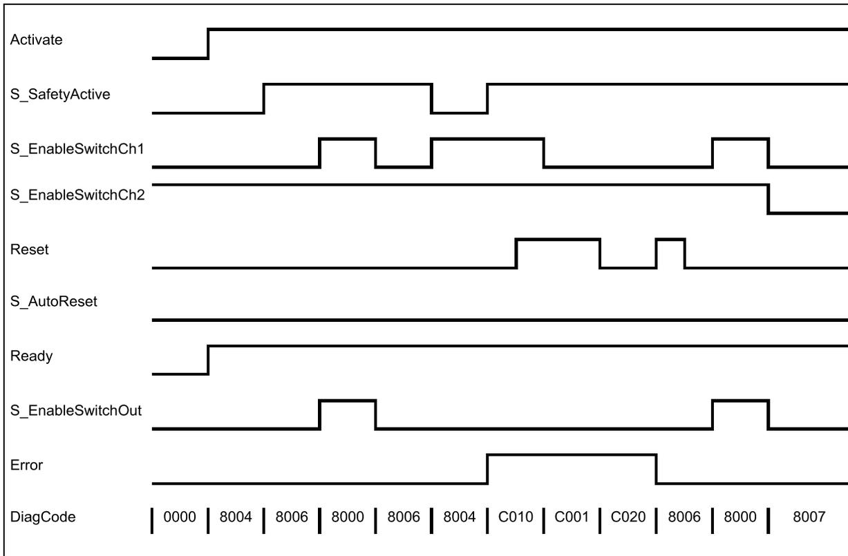
Fig. 118: Timing diagram for SF\_EnableSwitch: S\_AutoReset = FALSE
