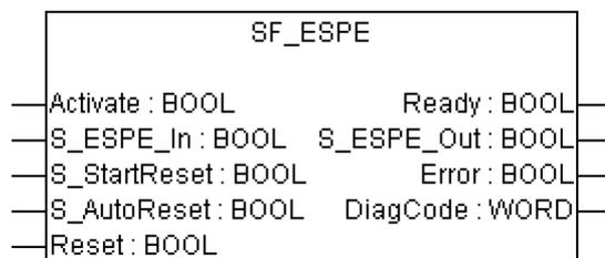
This function block is a safety-related function block for monitoring electro-sensitive protective equipment (ESPE). The function is identical to SF\_EmergencyStop. The S\_ESPE\_Out output signal is set to FALSE as soon as the S\_ESPE\_In input is set to FALSE. The S\_ESPE\_Out output signal is set to TRUE only if the S\_ESPE\_In input is set to TRUE and a reset occurs. The enable reset depends on the defined S\_StartReset, S\_AutoReset, and Reset inputs.
