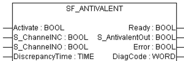
This function block converts two antivalent BOOL inputs (NO/NC pair) to one BOOL output with discrepancy time monitoring. This FB should not be used stand-alone since it has no restart interlock. It is required to connect the output to other safety related functionalities.
