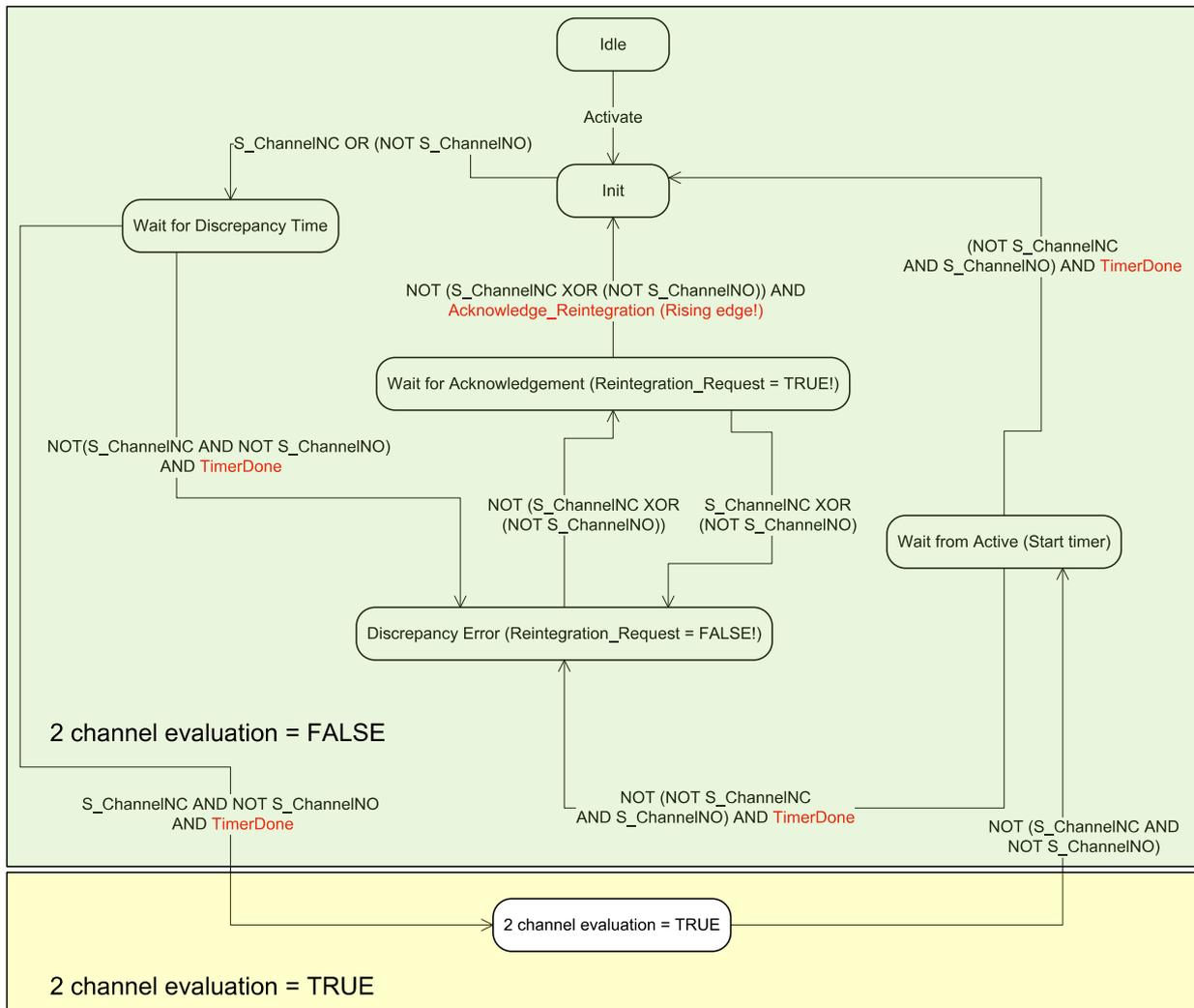
Fig. 38: 2 channel antivalent mode implemented in DX581-S
