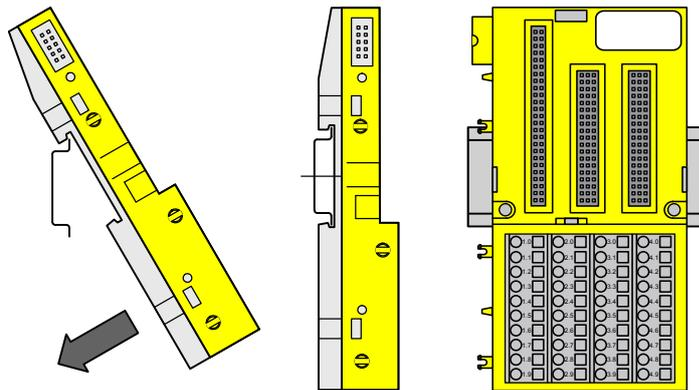
Fig. 60: Assembly instruction for mounting on a DIN rail
