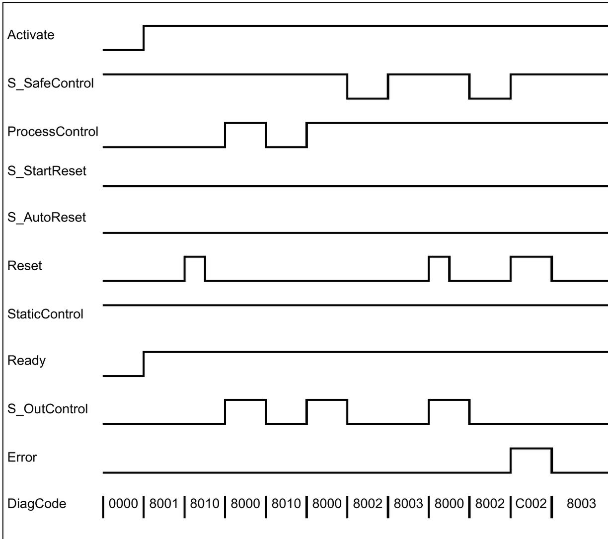
Fig. 122: Timing diagram for SF\_OutControl: S\_StartReset = FALSE
