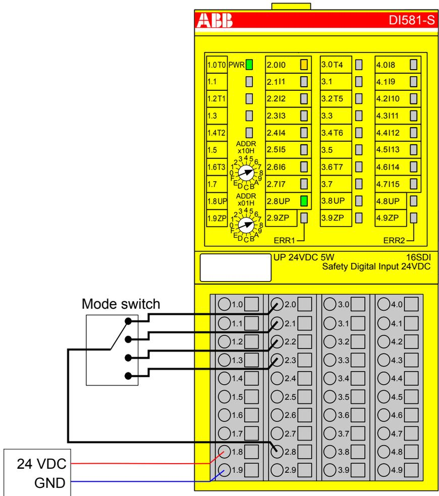
Fig. 35: Circuit example DI581-S, mode switch 1 from 4, 24 V DC
