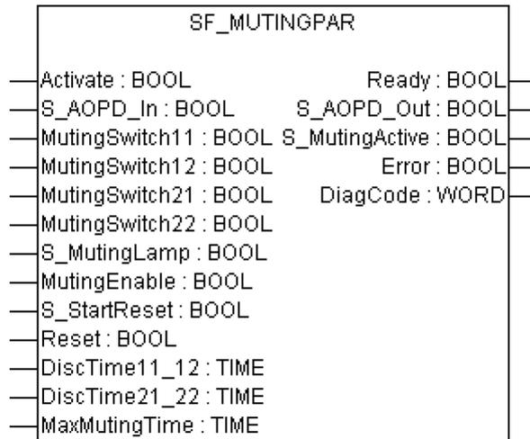
Muting is the intended suppression of the safety function. In this FB, parallel muting with four muting sensors is specified.
