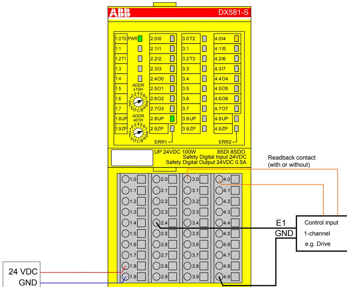
Fig. 46: Circuit example DX581-S, Transistor input (1-channel)
