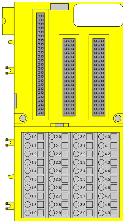
Spring-type terminal unit TU582-S for Safety I/O modules.
