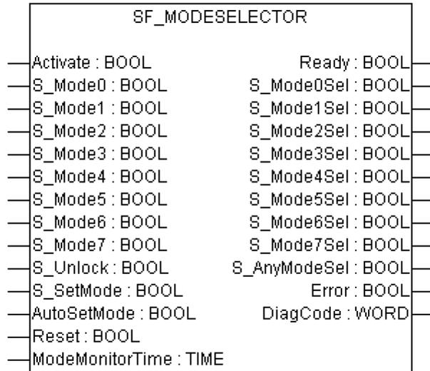
This function block selects the system operation mode, such as manual, automatic, semi-automatic, etc.
