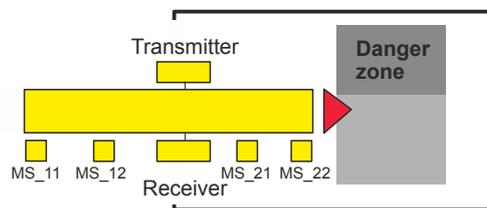
Before muting sensors MutingSwitch11 (MS\_11) and MutingSwitch12 (MS\_12) are disabled, muting sensors MutingSwitch21 (MS\_21) and MutingSwitch22 (MS\_22) must be activated. This ensures that muting mode remains active.
