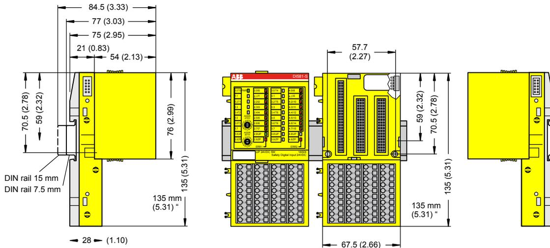
Fig. 21: Dimensions of DI581-S Safety I/O module
