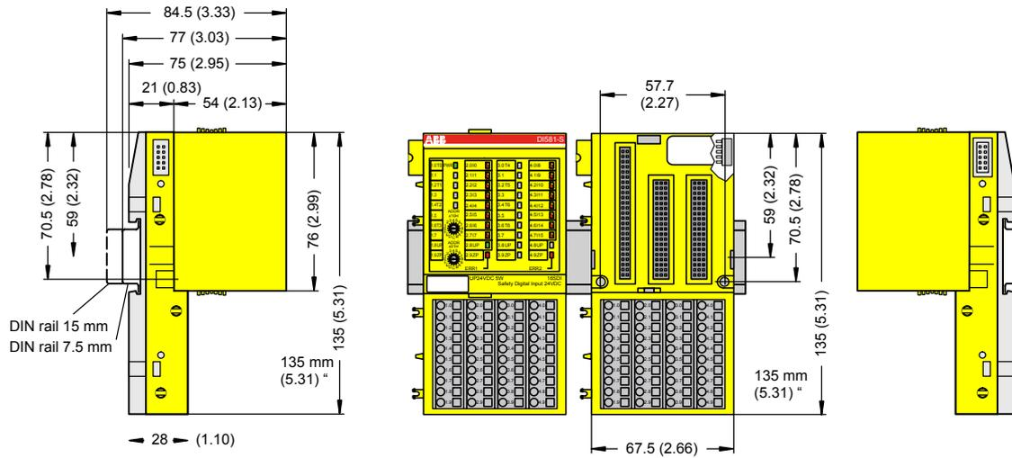
Fig. 61: Dimensions of TU582-S Safety I/O Terminal Unit
