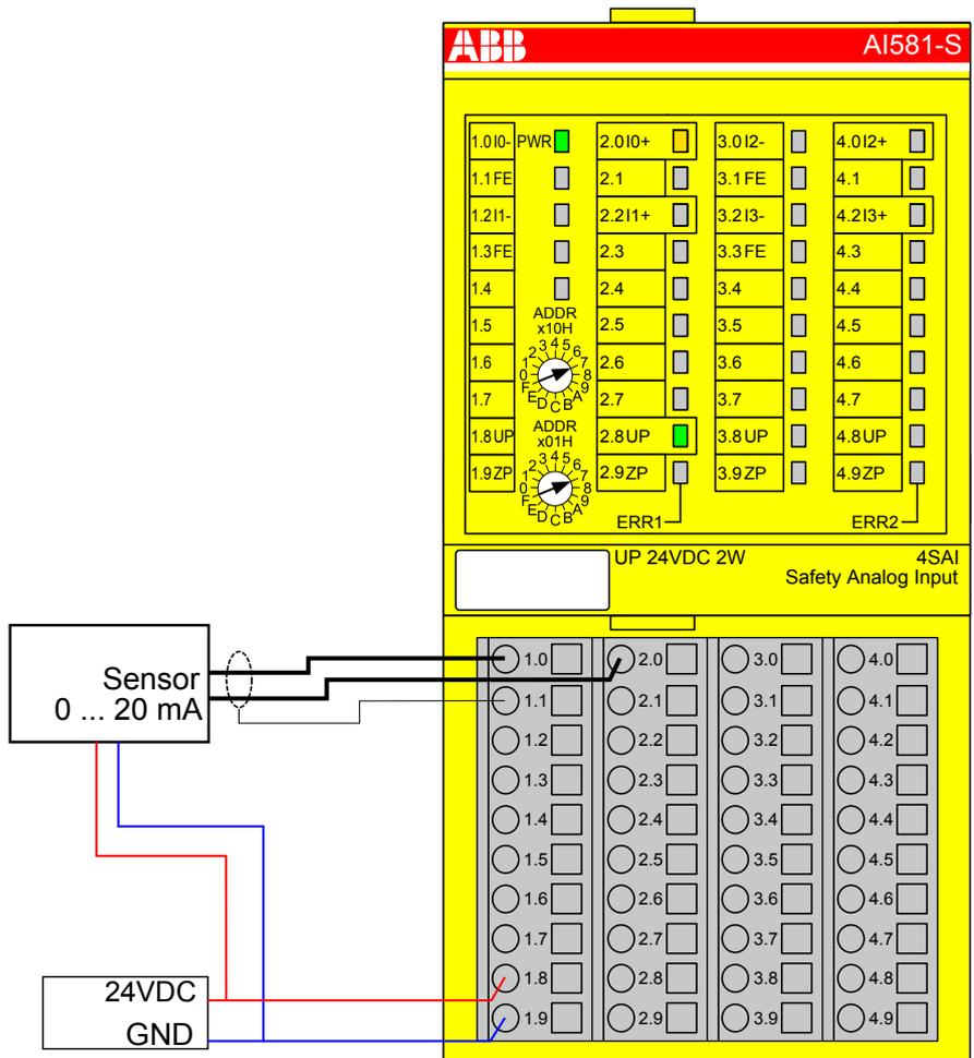
Fig. 55: Circuit example AI581-S, analog sensor (0 ... 20 mA)
