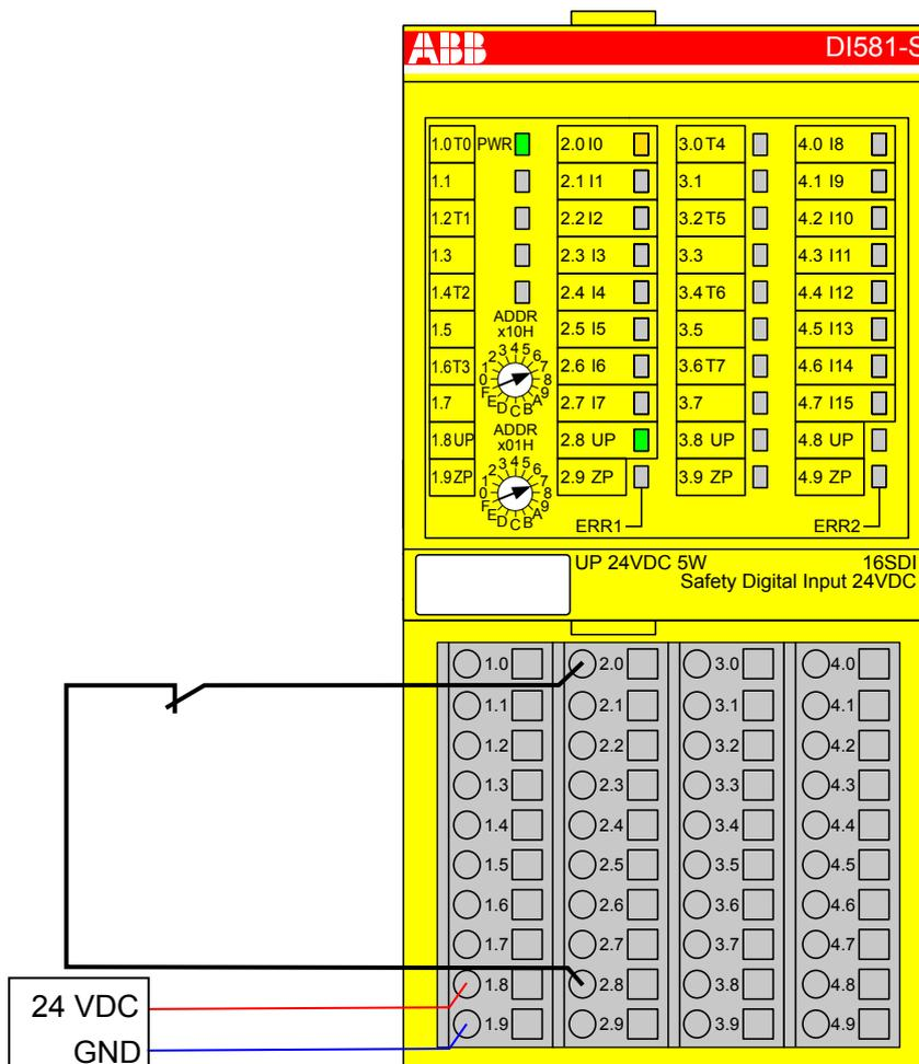
Fig. 24: Circuit example DI581-S, 1-channel sensor, 24 V DC
