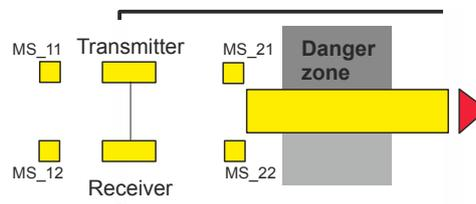
Muting mode is terminated if either muting sensor MutingSwitch21 (MS\_21) or MutingSwitch22 (MS\_22) is disabled by the product. The maximum time for muting mode to be active is the MaxMutingTime.
