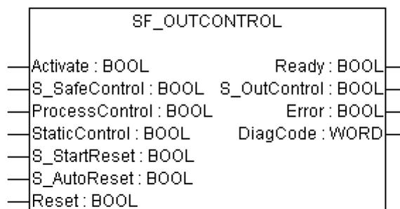
Control of a safety output with a signal from the functional application and a safety signal with optional startup inhibits.
