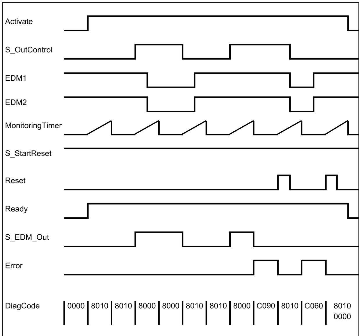
Fig. 125: Timing diagrams for SF\_EDM: S\_StartReset = TRUE
