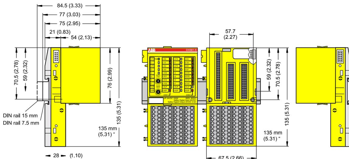
Fig. 41: Dimensions of DX581-S Safety I/O module
