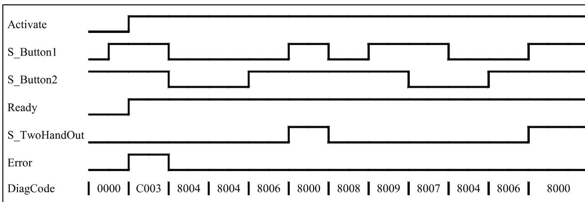
Fig. 110: Timing diagram for SF\_TwoHandControlTypell
