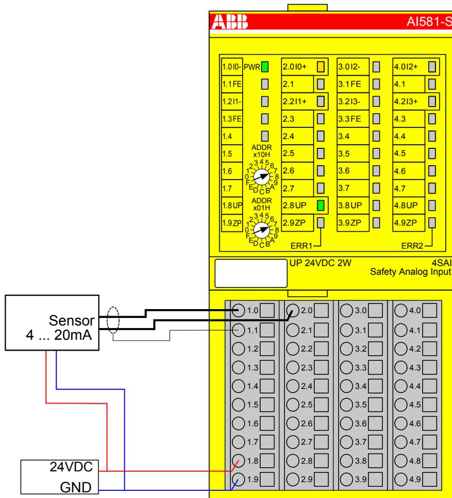
Fig. 57: Circuit example AI581-S, analog sensor (4 ... 20 mA)
