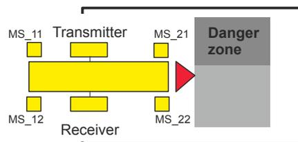
Before muting sensors MutingSwitch11 (MS\_11) and MutingSwitch12 (MS\_12) are disabled, muting sensors MutingSwitch21 (MS\_21) and MutingSwitch22 (MS\_22) must be activated. This ensures that muting mode remains active. The time discrepancy between switching of MutingSwitch21 and MutingSwitch22 is monitored by the time DiscTime21\_22.
