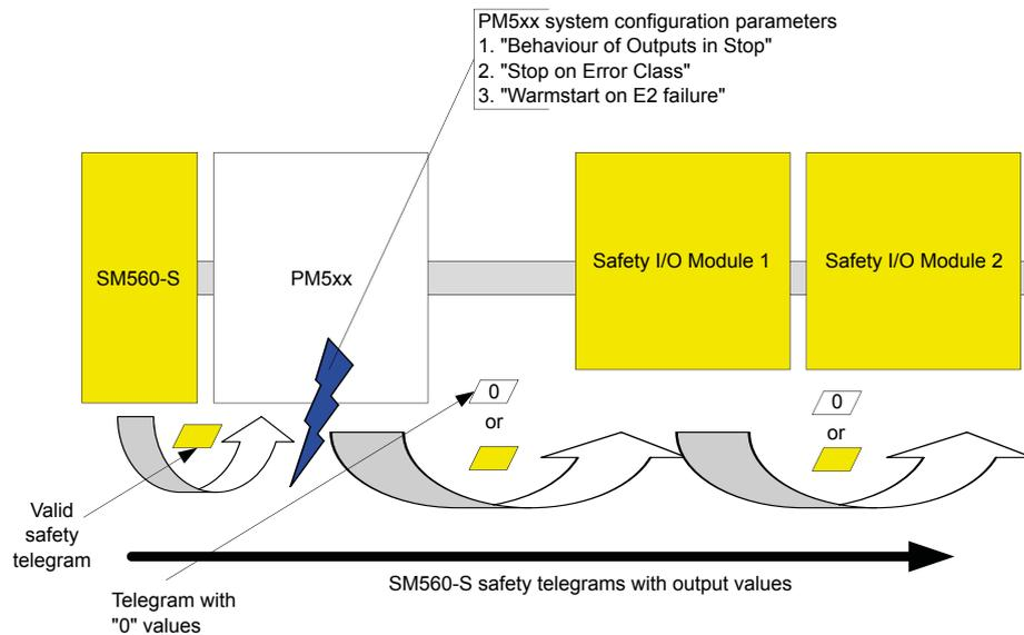
Fig. 12: Overview on how PM5xx system parameter setting influences SM560-S safety telegram flow
