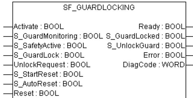
This FB controls an entrance to a hazardous area via an interlocking guard with guard locking ("four state interlocking").
