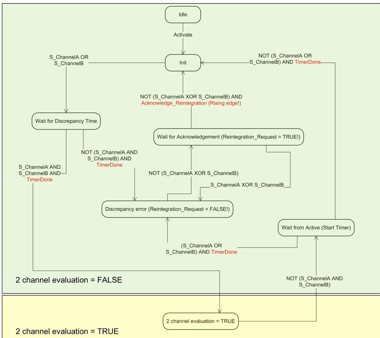
Fig. 37: 2 channel equivalent mode implemented in DX581-S
