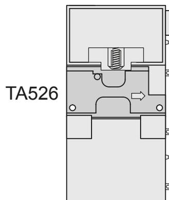
**1.** Snap TA526 on the rear side of the Terminal Unit like DIN rails.
