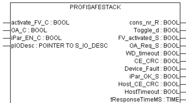
This function block represents PROFIsafe F-Device instance in the PROFIsafe F-Host to control and monitor the status of the given F-Device [3].
