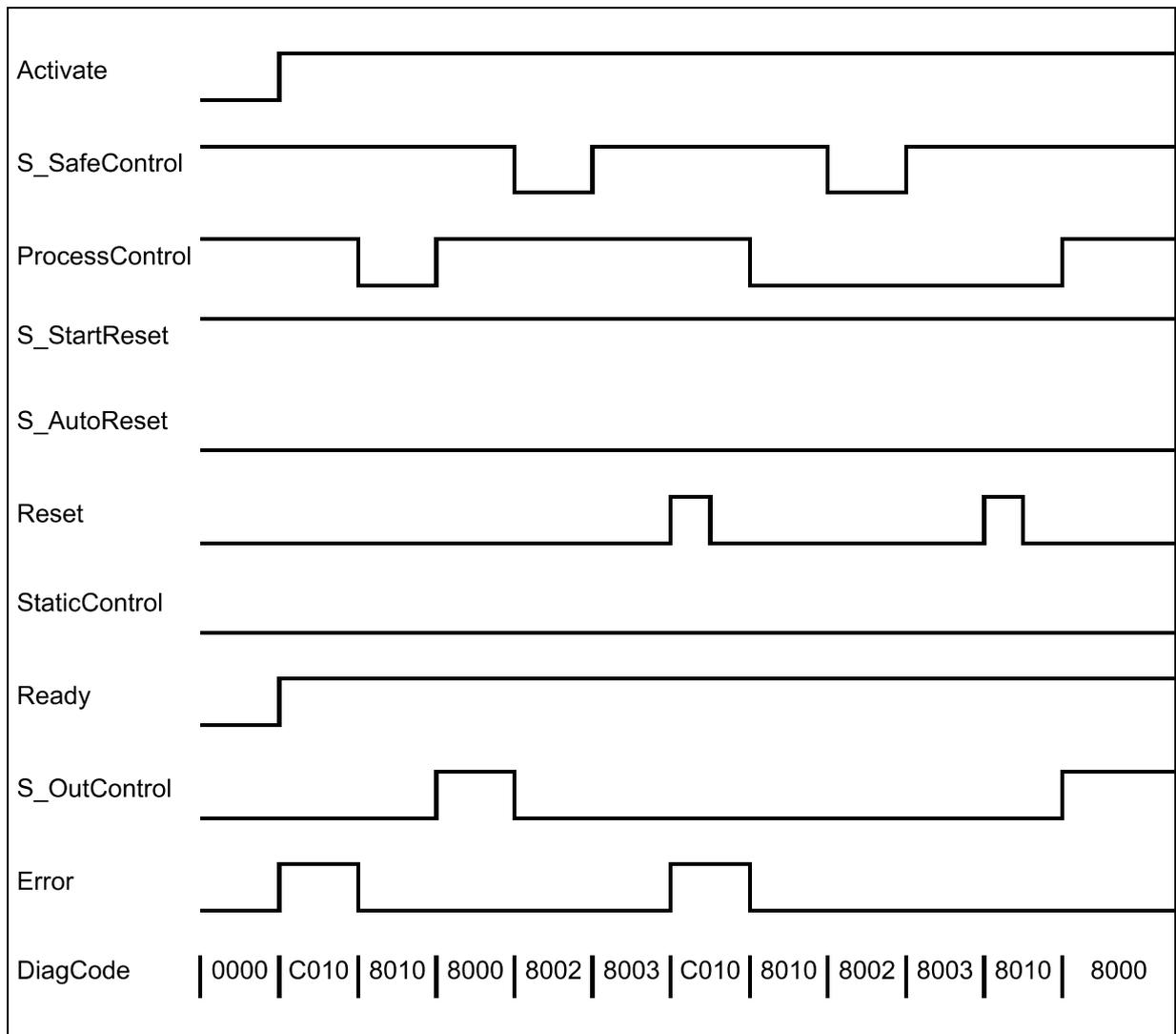
Fig. 123: Timing diagram for SF\_OutControl: S\_StartReset = TRUE
