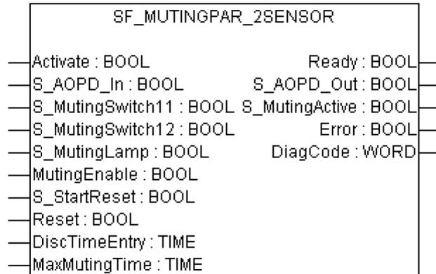
Muting is the intended suppression of the safety function. In this FB, parallel muting with two muting sensors is specified.
