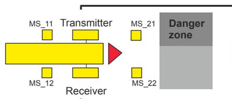
Muting mode remains active as long as MutingSwitch11 (MS\_11) and MutingSwitch12 (MS\_12) are activated by the product. The product may pass through the light curtain without causing a machine stop.
