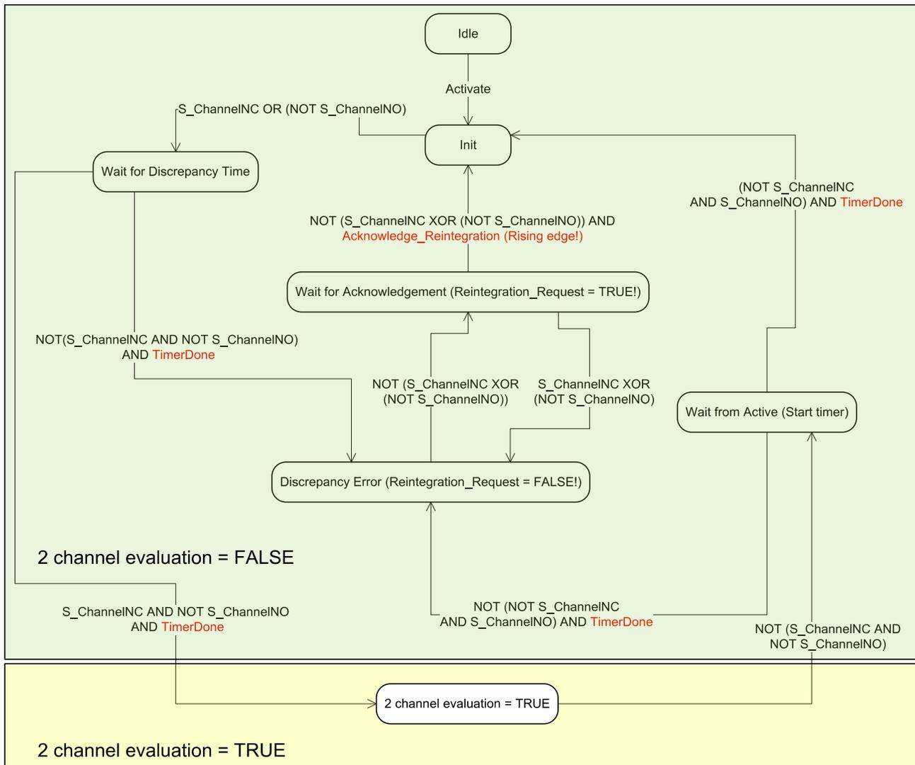
Fig. 18: 2 channel antivalent mode implemented in DI581-S
