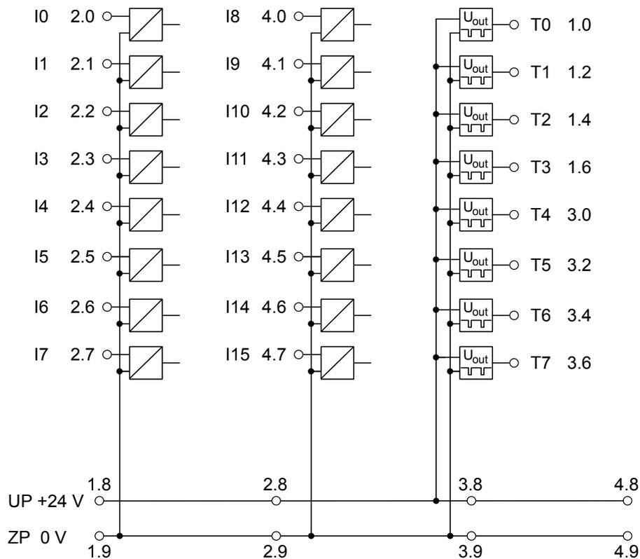
Fig. 22: Example of electrical connections with DI581-S
