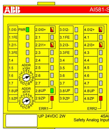
Safety analog input module AI581-S with 4 safety current input channels 0 ... 20 mA (up to SIL2 or PL d) or 2 safety current input channels (up to SIL3 or PL e).
