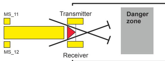
If reflection light barriers are used as muting sensors, they are generally arranged diagonally. In general, this arrangement of reflection light barriers as muting sensors requires only two light barriers, and only S\_MutingSwitch11 (MS\_11) and S\_MutingSwitch12 (MS\_12) are allocated.
