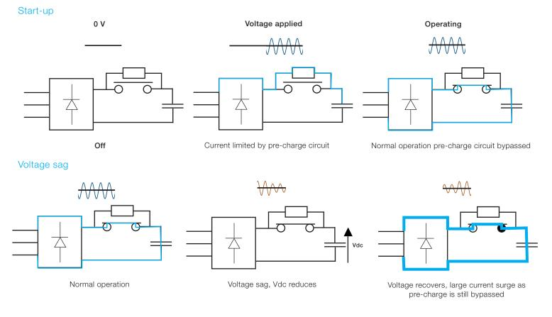
Figure one: Top normal controlled startup process. Bottom Inrush currents following a voltage sag
