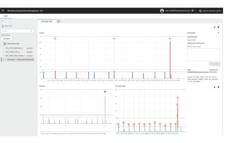
Statistical Process Control (SPC) is a quality method to supervise if a process is in state of control and whether it can produce units within given tolerances. The SPC application enables the user to define and monitor control cards. These control cards include visual diagrams that can track shop floor processes in real-time and help to continually improve the process and operational excellence.
