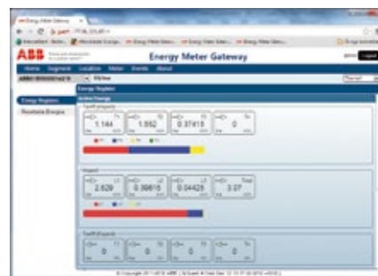
G13 provides easy management of system parameters through the many web pages pre-configured to manage energy consumption.
