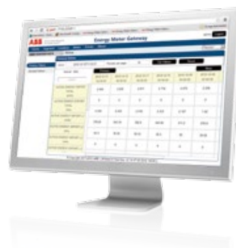
The web server function of the G13 gateway allows easy remote reading of the information collected from the system meters.
