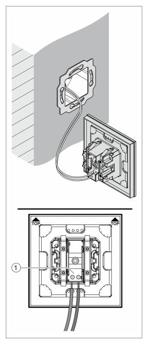
Fig. 15: Connection of the bus line
