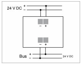
Fig. 18: Connection of bus coupler and display
