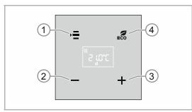
Fig. 25: RTC control elements
