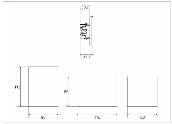
Fig. 5: Dimensions (all dimensions are in mm)
