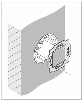
Fig. 14: Installation of the support ring
