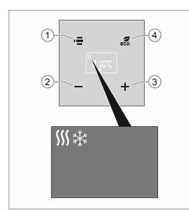
Fig. 28: Heating/cooling operating mode
