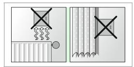
Fig. 9: Installation site – Position of RTC
