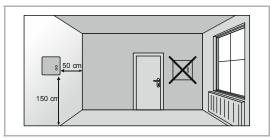
Fig. 6: Installation site - Distance
