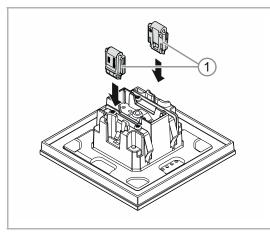
To install the device, perform the following steps:
