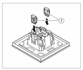
Fig. 6: Installation of the removal protection
