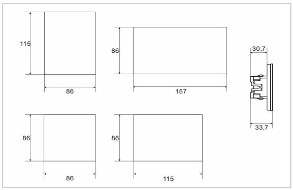
Fig. 5: Dimensions (all dimensions are in mm)
