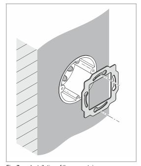
Fig. 7: Installation of the support ring
