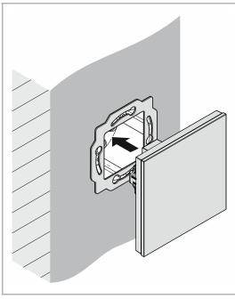
Fig. 10: Mounting devices
