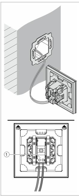
Fig. 8: Connection of the bus line
