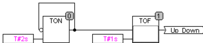
Image 2.11: A network in the continuous function chart editor
