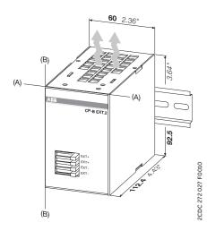
The device has to be mounted horizontally with the input terminals on the bottom. In order to ensure a sufficient convection, the minimum distance to the other modules must be not less than 40 mm (1.58 in) in vertical direction. Minimum distance in horizontal direction is not necessary.
