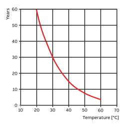
Capacitor's life span over temperature
