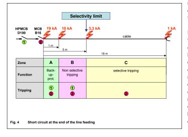
upstream high performance device is not really required in the case of short-circuit currents just above 3300 A. However, the protective function occurs automatically as the result of the selectivity limit.
