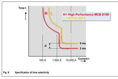
With regards to selectivity in the case of an overload it can be said that full selectivity can be expected due to the difference in rated current of the downstream High Performance Miniature Cicuit Breaker of 100 A. There are no points of intersection between the two thermal trip characteristics.
