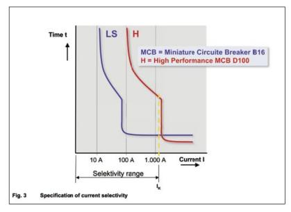
High Performance Miniature Circuit Breaker (HPMCB) and the final circuit's miniature circuit breaker are series connected as in the example in Fig. 1. Due to the difference of the rated currents of the two protective devices, i.e. 16 A to 100 A against the direction of energy flow, the full selectivity of both protective devices is assured in the overload area (curved zone of the trip characteristic curves), as the two curves neither touch nor intersect each other.
