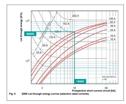
However, effective short-circuit protection is, in accordance with IEC 60364-4-43, only possible if the let through energy (l<sup>2</sup>t) in case of a short-circuit is less than the maximum allowable short-time energy ( $k^2S^2$ ) for the wire insulation to be protected:
