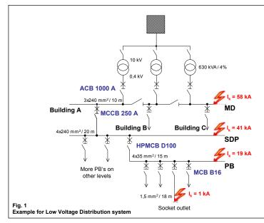
requirements concerning modern low voltage distribution systems which were outlined at the outset are taken into account, overcurrent protective devices with special features, the so-called High Performance Miniature Circuit Breakers (HPMCB, Table 1), should be selected.
