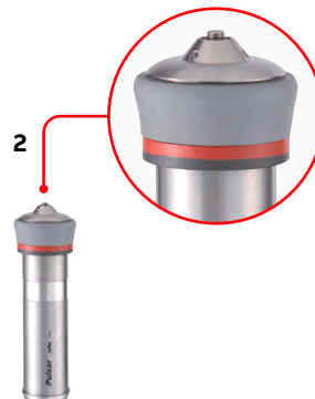
RodCheck after lightning stroke of few kA
