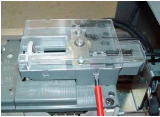
Figs. 1 and 2: Cover removal
