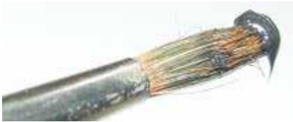
Fig. 3: Grease on the tip of brush
