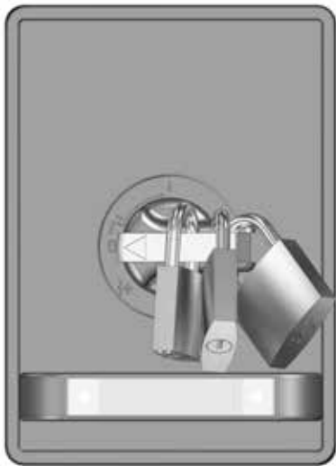
Fig. 40 Size 8E/4 withdrawable module with 3 padlocks
