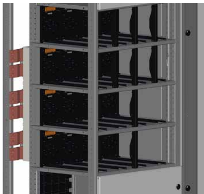
Fig. 53 Conversion to size 8E/4 and 8E/2 withdrawable module compartments
