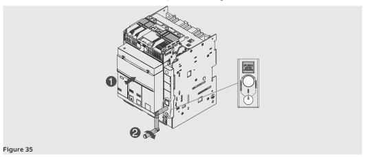
7. Press the lock button and then rotate the crank clockwise until the button comes out and the indicator shows that the circuit-breaker is in the **CONNECT** position. See Figure 36.
