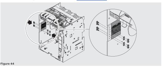
Mounting the fixed part of the Fix the fixed part to a horizontal surface using four M8 x 25 screws (see Figure 45). Tighten the screws withdrawable circuit-breaker with tightening torque = 21 Nm - 186 lb in.
