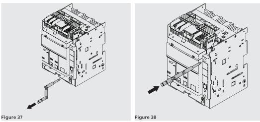
To extract the moving part from the fixed part, perform the same steps indicated for insertion in reverse order.
