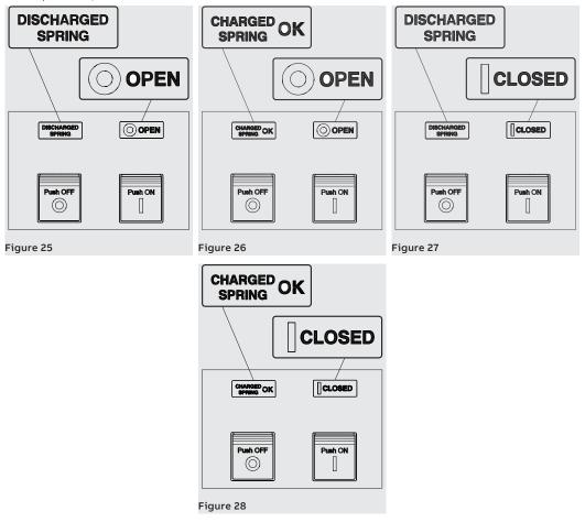
Circuit breaker racking-in/ racking-out operations
