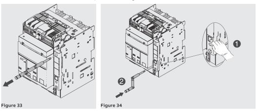
6. Keep breaker pushed. Turn the crank clockwise until the pushbutton comes out and the indicator shows that the circuit-breaker is in **TEST** position. See Figure 35.
