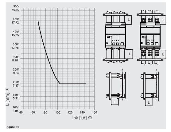
(1): distance of the first anchor plate from the circuit-breaker terminals (2): peak current
