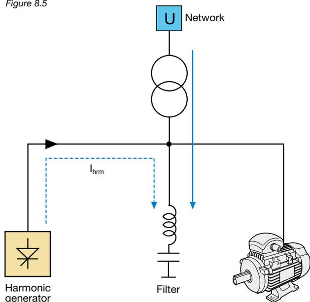
Therefore this filter, called *passive filter*, consists in a capacitor connected in series with an inductor so that the resonance frequency is altogether equal to the frequency of the harmonic to be eliminated.
