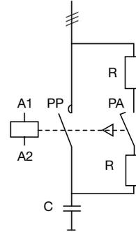
When the main poles PP are closed, the opening of the auxiliary poles is automatically carried out by switching off the resistors as shown in the following diagram.
