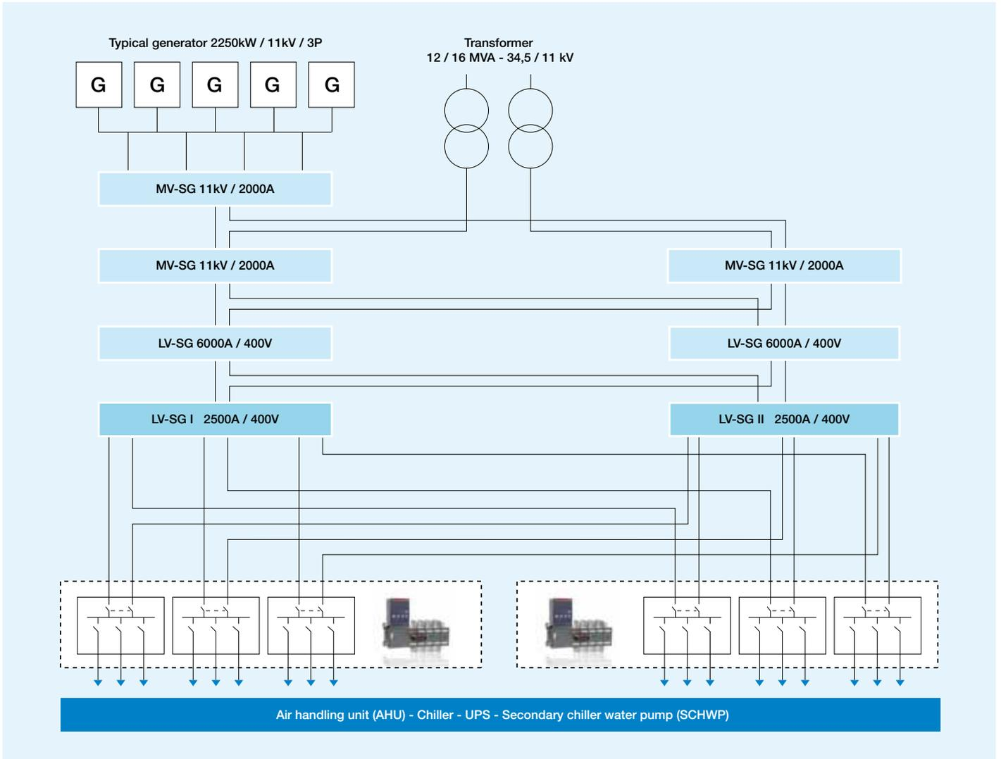
In Data centers automatic transfer switches are predominantly used to backup cooling facilities (air-handling units and chillers) on UPS (Uninterruptible Power Supply) that ensures short time power supply in case of emergency.
