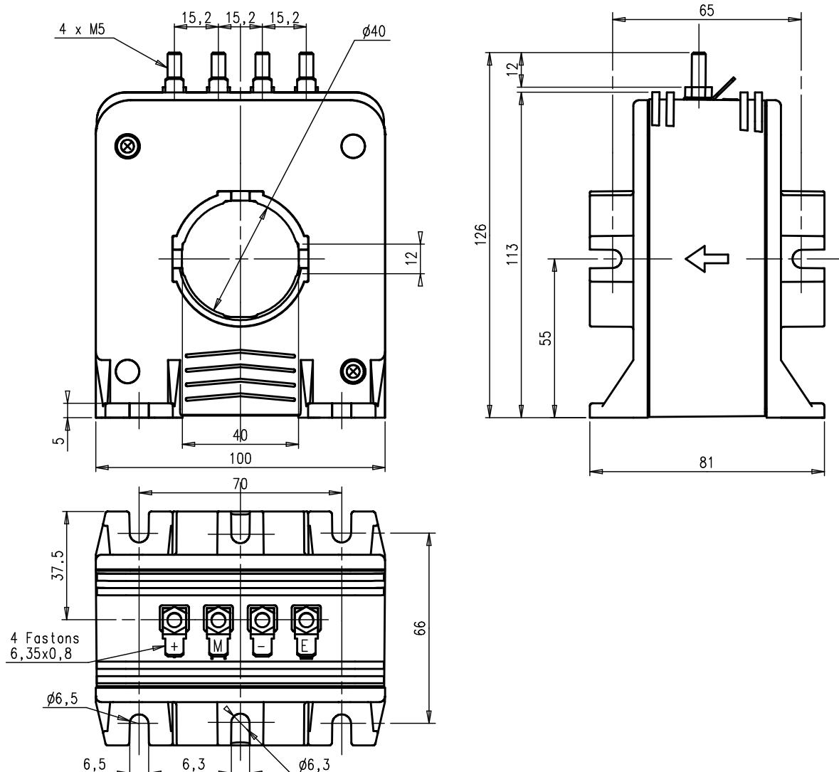
**Maximum M5 tightening torque: 2 N.m**
