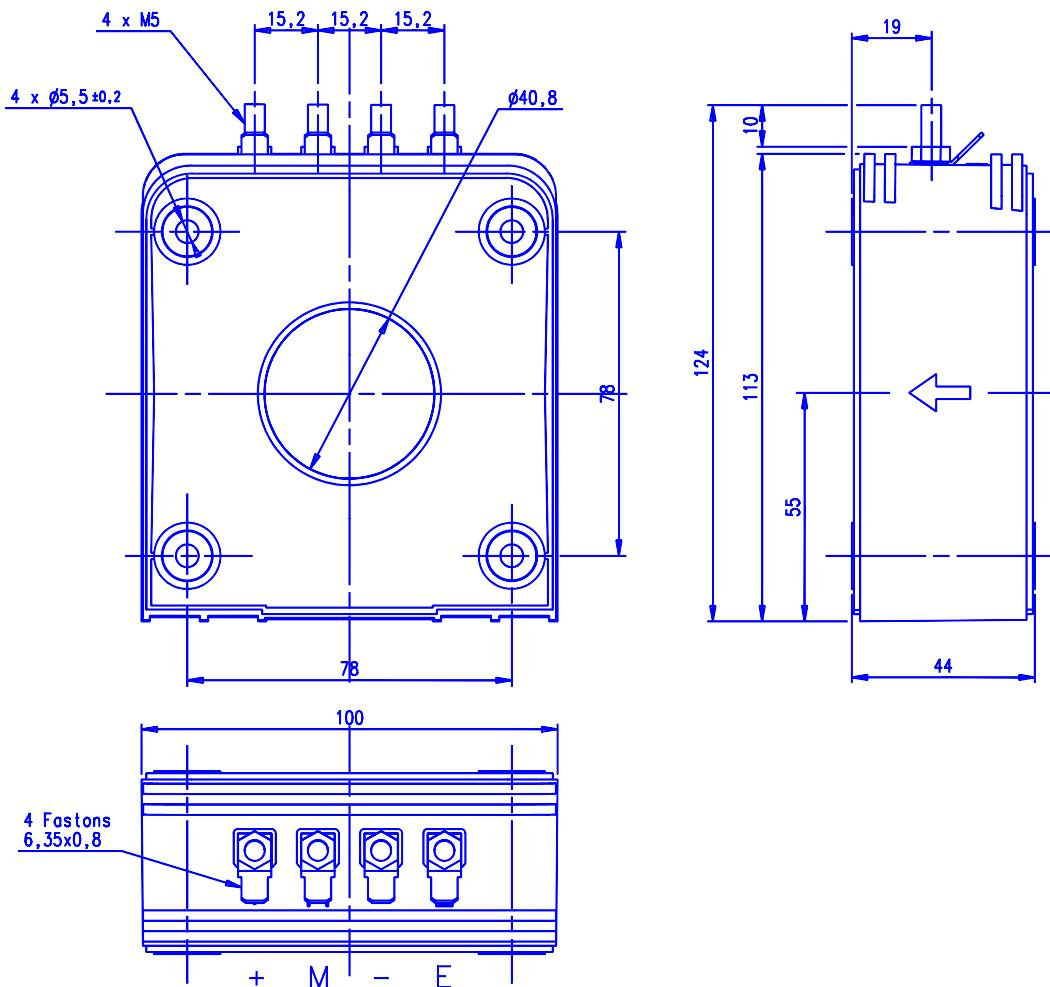
Maximum M5 tightening torque: 2 N.m
