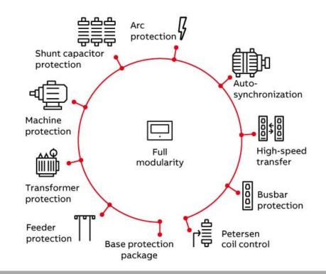
Innovative design – setting a new standard for what is possible with a single protection and control device
