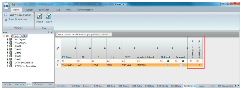
Figure 45: Connecting the SMV sender and receivers in IET600
