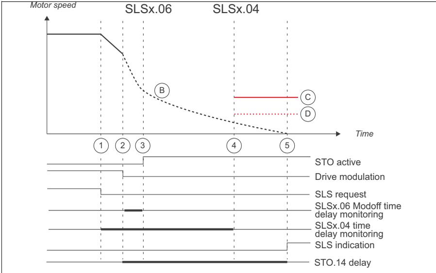
1. SLS request is activated (*SLSx.11 SLS1 input A* = DI X113:2 & X114:2). SLS time delay monitoring is started (*SLSx.04 SLS time delay* = 2000 ms). Deceleration to SLS limit speed is started (23.13 Deceleration time 1).
