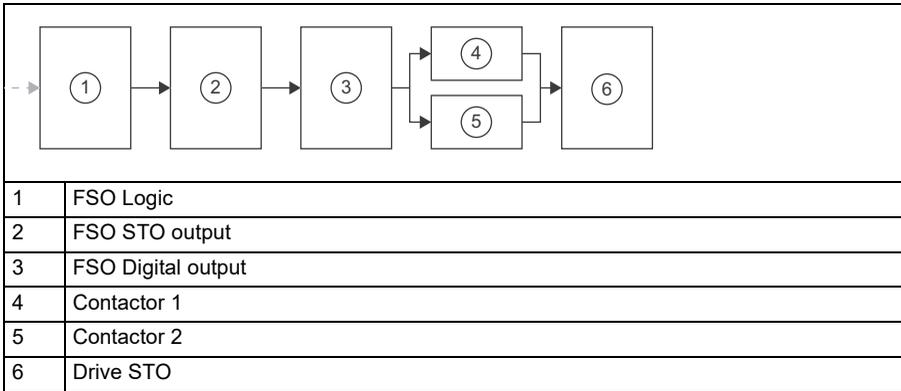
Safe brake control (SBC) includes the following subsystems: FSO Logic, FSO STO output, FSO Digital output, Contactor 1 and 2 (can be provided by ABB), and Drive STO.
