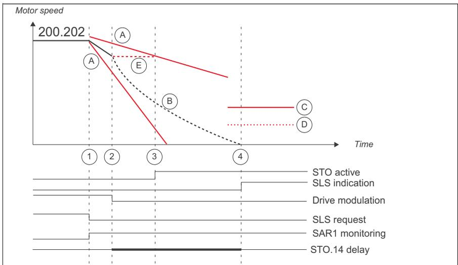
1. SLS request is activated (*SLSx.11 SLS1 input A* = DI X113:2 & X114:2). SLS ramp monitoring is activated (SAR1). Parameter *200.202 SAR speed scaling* (= 1500 rpm) is used as a reference point in ramp time calculations. Deceleration towards the SLS limit speed is started according to SAR1 parameters.
