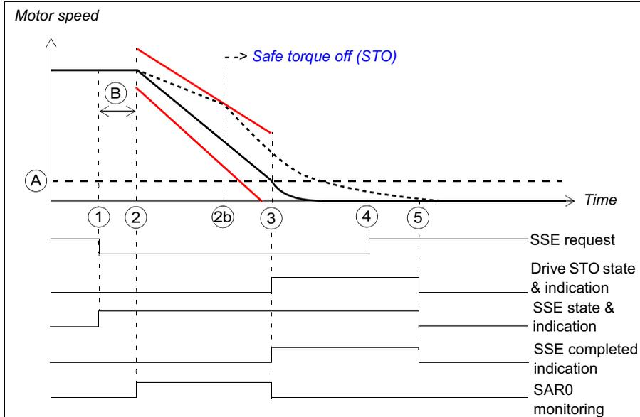
A Zero speed (parameter [FSOGEN.51](#)): Speed limit for activating the drive STO function. The safety function is completed, ramp monitoring is stopped and the SSE completed indication (parameter [SSE.22](#)) goes on. The acknowledgment becomes allowed.
