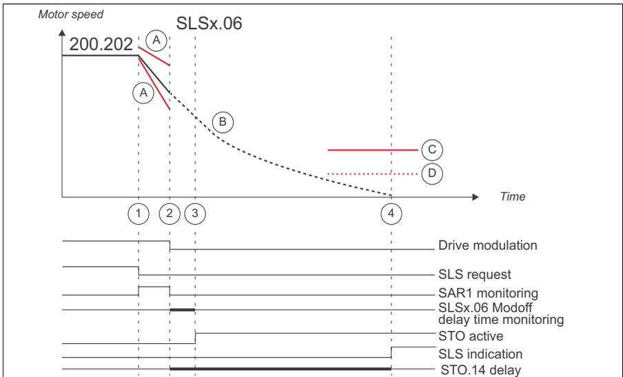
1. SLS request is activated (*SLSx.11 SLS1 input A* = DI X113:2 & X114:2). SLS ramp monitoring is activated (SAR1). Parameter *200.202 SAR speed scaling* (= 1500 rpm) is used as a reference point in ramp time calculations. Deceleration towards the SLS limit speed is started according to SAR1 parameters:
