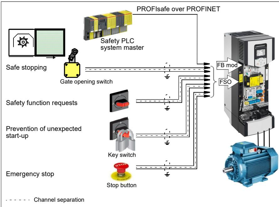
The FSO safety functions module is an option for the ACS880 drives. The Safe torque off (STO) function is a standard feature on the ACS880 drives.
