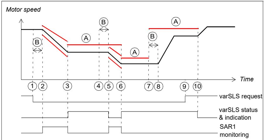
A Variable SLS trip limits (parameter [SL<sub>Sx</sub>.43](#) and the scaling values set in the safety PLC)
