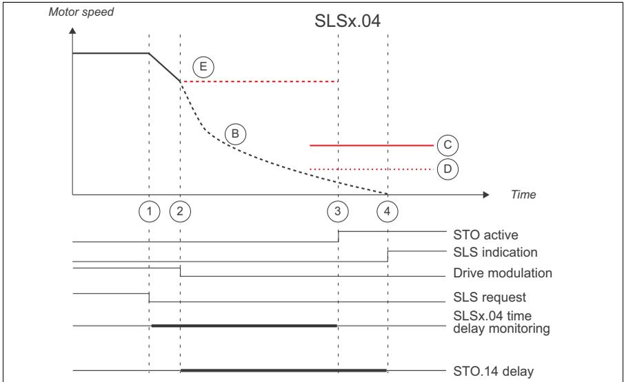
1. SLS request is activated (*SLSx.11 SLS1 input A* = DI X113:2 & X114:2). SLS time delay monitoring is started (*SLSx.04 SLS time delay* = 2000 ms). Deceleration to SLS limit speed is started (drive parameter 23.13 Deceleration time 1).
