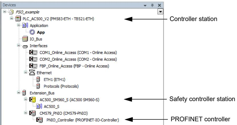
6. Right-click on the PROFINET controller **CM579-PNIO-Master** and add the FENA module to the PROFINET IO network.
