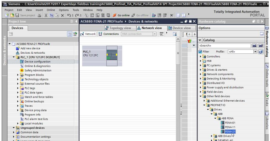
5. Open the FENA-21 device view and add (by dragging and dropping) the desired PPO and PS telegrams to slot 1 and 2. In this example, we use PPO7 and PS2 (Additional info in manuals).
