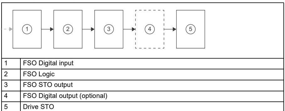
**Block diagram for dual channel solution:**
