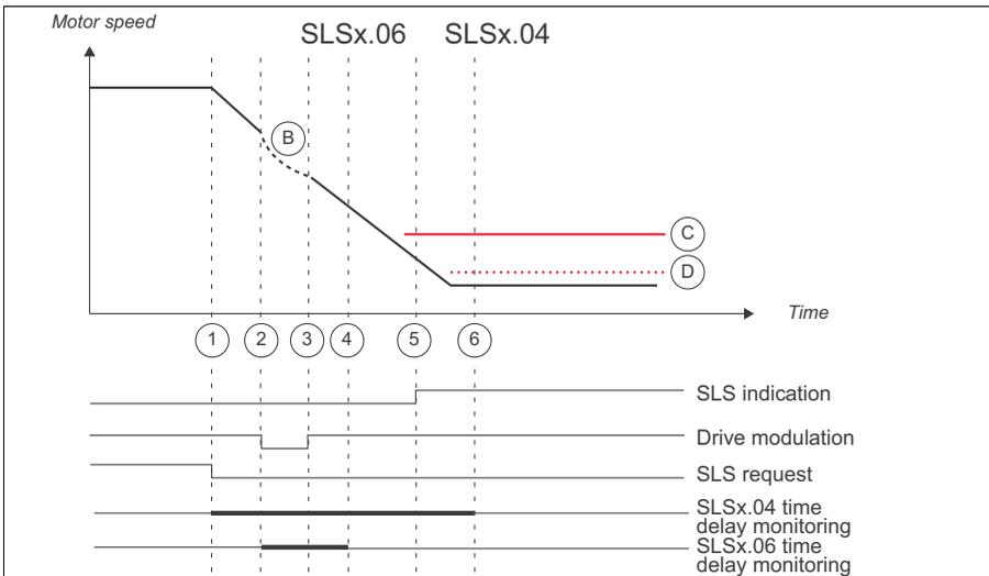
1. SLS request is activated (*SLSx.11 SLS1 input A* = DI X113:2 & X114:2). SLS time delay monitoring is started (*SLSx.04 SLS time delay* = 2000 ms). Deceleration to SLS limit speed is started (23.13 Deceleration time 1).
