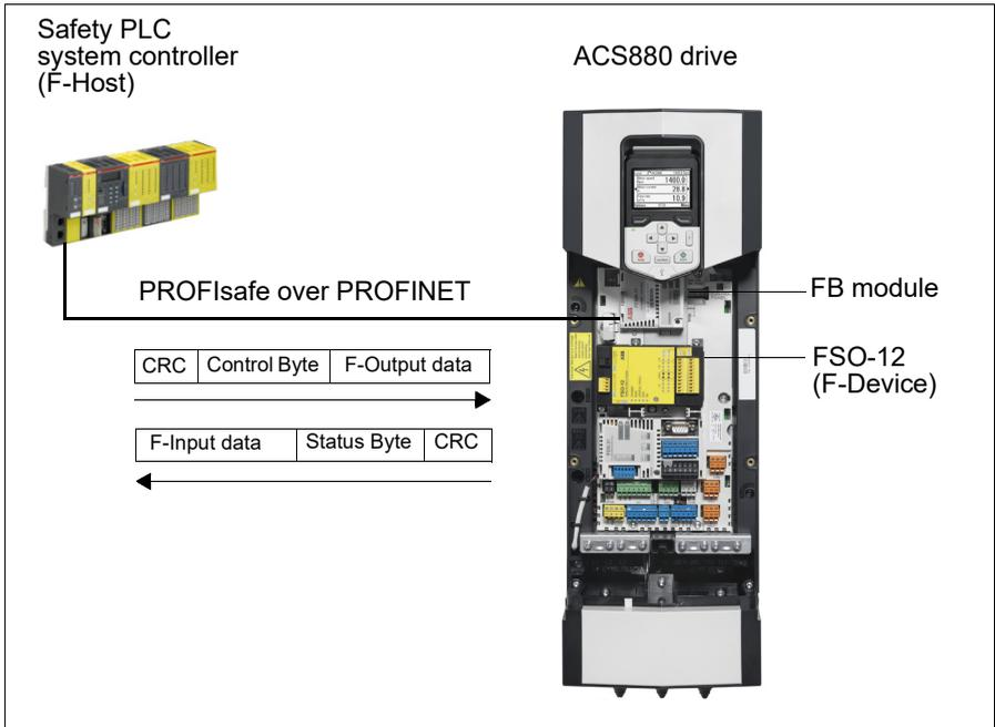
The FSO safety functions module and the FB module are installed on the ACS880 drive. The safety PLC is connected to the FB module, which communicates with the FSO module. The safety PLC activates safety functions via the PROFIsafe communication bus. The user can also activate safety functions from an I/O device (for example, an emergency stop button) which is connected to the FSO module.
