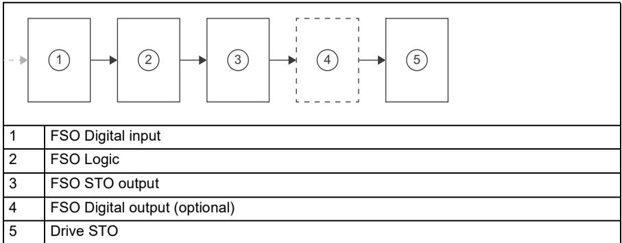
Prevention of unexpected start-up (POUS) includes the following subsystems: FSO Digital input, FSO Logic, FSO STO output, FSO Digital output (optional), and Drive STO.
