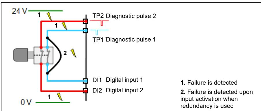
**Note:** If only one of the redundant inputs is activated upon a safety function request, the FSO module activates the safety function in which the input is configured but it cannot be acknowledged before the failure has been repaired. To acknowledge the safety function, you must set both input channels down and up at the same time or, switch the power off and on.
