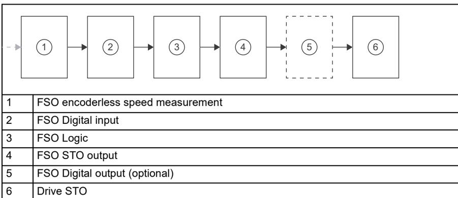
Safely-limited speed (SLS) without encoder includes the following subsystems: FSO encoderless speed measurement, FSO Digital input, FSO Logic, FSO STO output,
