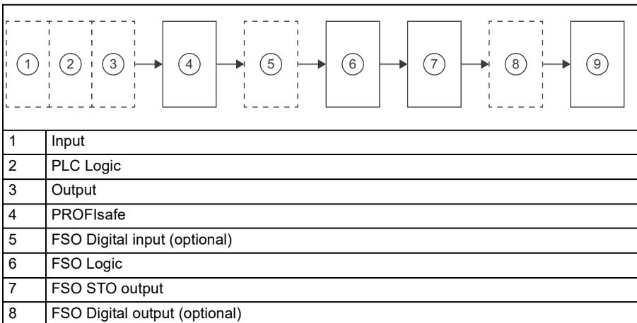
PROFIsafe can replace digital inputs and/or digital outputs of the FSO. For example, it is possible to use PROFIsafe input and FSO output in the same configuration.
