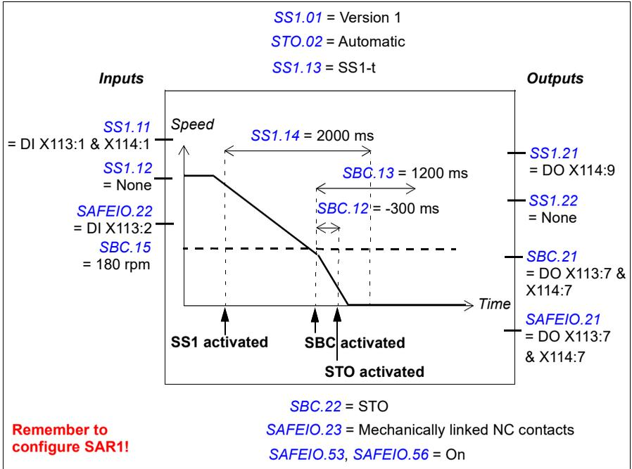
**Example 2:** The figure below shows an example of the SS1-r function with speed limit activated SBC, SBC before STO set-up:
