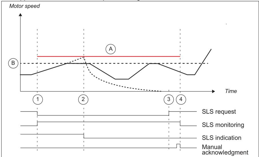
A SLS trip limit positive (parameter *SLSx.14*, *SLSx.23*, *SLSx.33* or *SLSx.43*)
