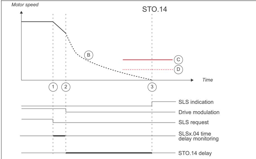
1. SLS request is activated (*SLSx.11 SLS1 input A* = DI X113:2 & X114:2). SLS time delay monitoring is started (*SLSx.04 SLS time delay* = 2000 ms). Deceleration to SLS limit speed is started (23.13 Deceleration time 1).
