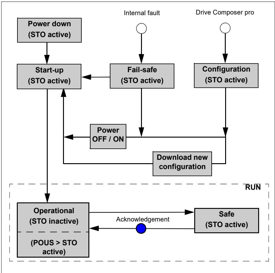
At power-up, the FSO goes into the Start-up mode. During the power-up process,
