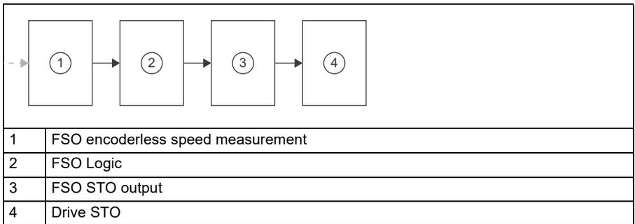
Safe maximum speed (SMS) includes the following subsystems: FSO encoderless speed measurement, FSO Logic, FSO STO output, and Drive STO.
