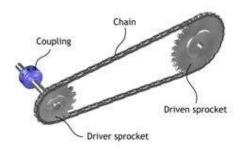
Figure 35 Chain and sprocket
