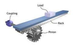
Figure 45 Rack and pinion mechanics
