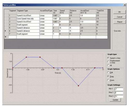
Figure 39 Motion profiles display
