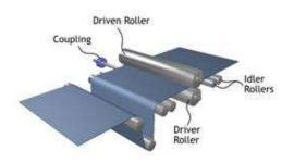
Figure 43 Feedroll mechanics
