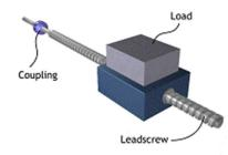
Figure 44 Lead screw mechanics
