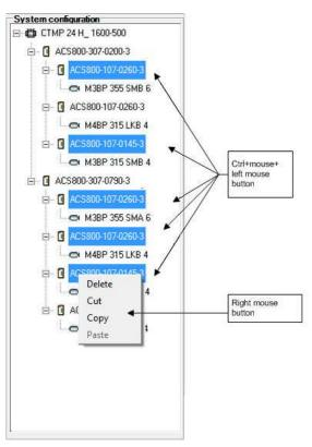
Figure 10: Highlighting several units at a time
