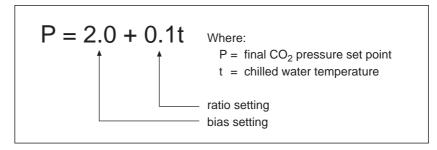
In the above example, with water chilled at  $10^{\circ}$ C, the design  $CO_2$  pressure is 3.0bar. If the water temperature changes by  $+1^{\circ}$ C, the  $CO_2$  pressure required would increase to 3.1bar.
