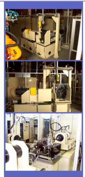
This machine automatically tests the axle for noise and vibration under a specified load. The machine is manually loaded and automatically positioned for the test sequence. An industrial PC with test software analyzes the gear through acceleration, full speed and deceleration modes.
