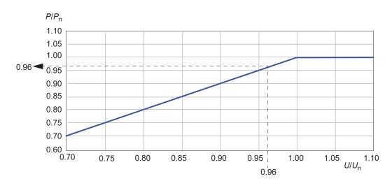
Example 1:  $P_n$  for ACS880-14-430A-7 is 400 kW. The supply voltage (U) is 660 V.
