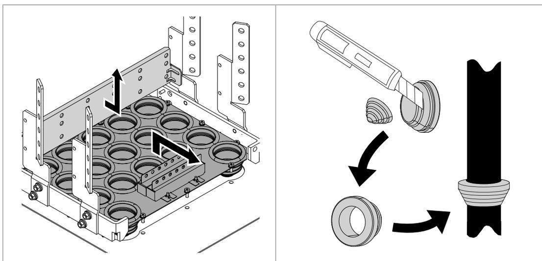
4. Lead the cables inside the cabinet through the cable entry plate. If there are several cables, use the rear 3 holes first. IP54 cabinet: Attach the the sealing grommets to the cable entry plate. Attach also the cable entry plate, and the cable support.
