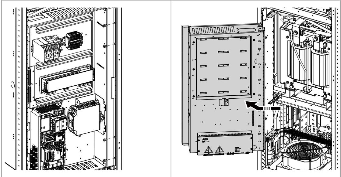
4. Loosen the two nuts on the studs attached to the fuse. Slide the fuse block out.
