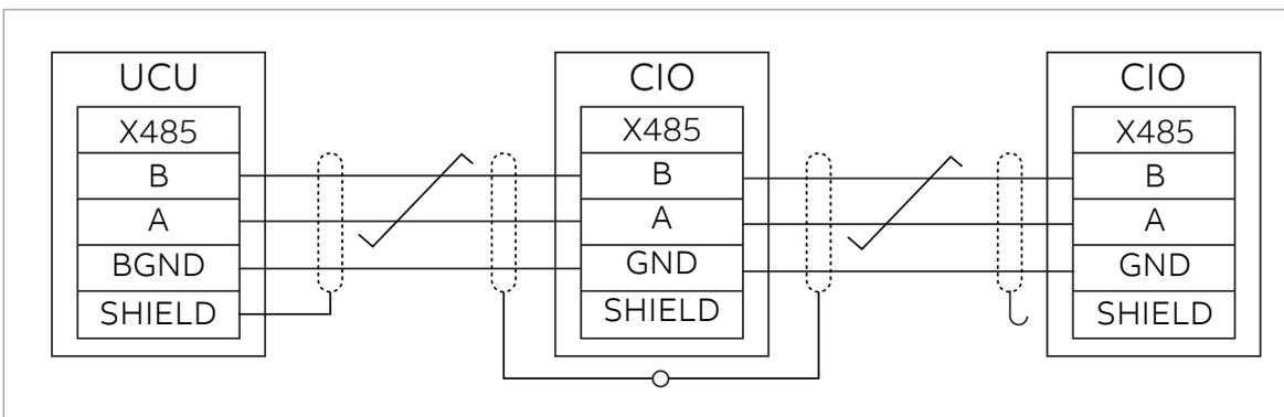
Terminate the I/O bus at its physical ends:
