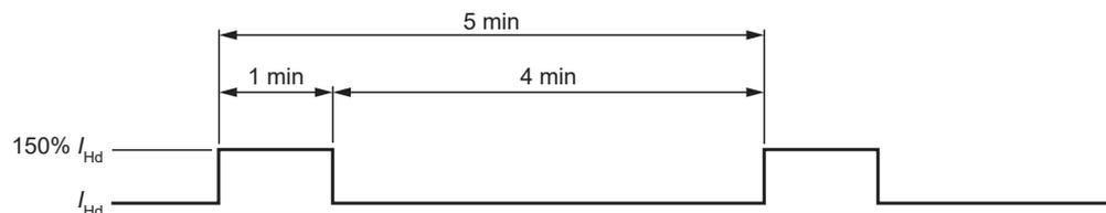
$P_{\text{Hd}}$  Continuous output power allowing 150%  $I_{\text{Hd}}$  for 1 min every 5 min
