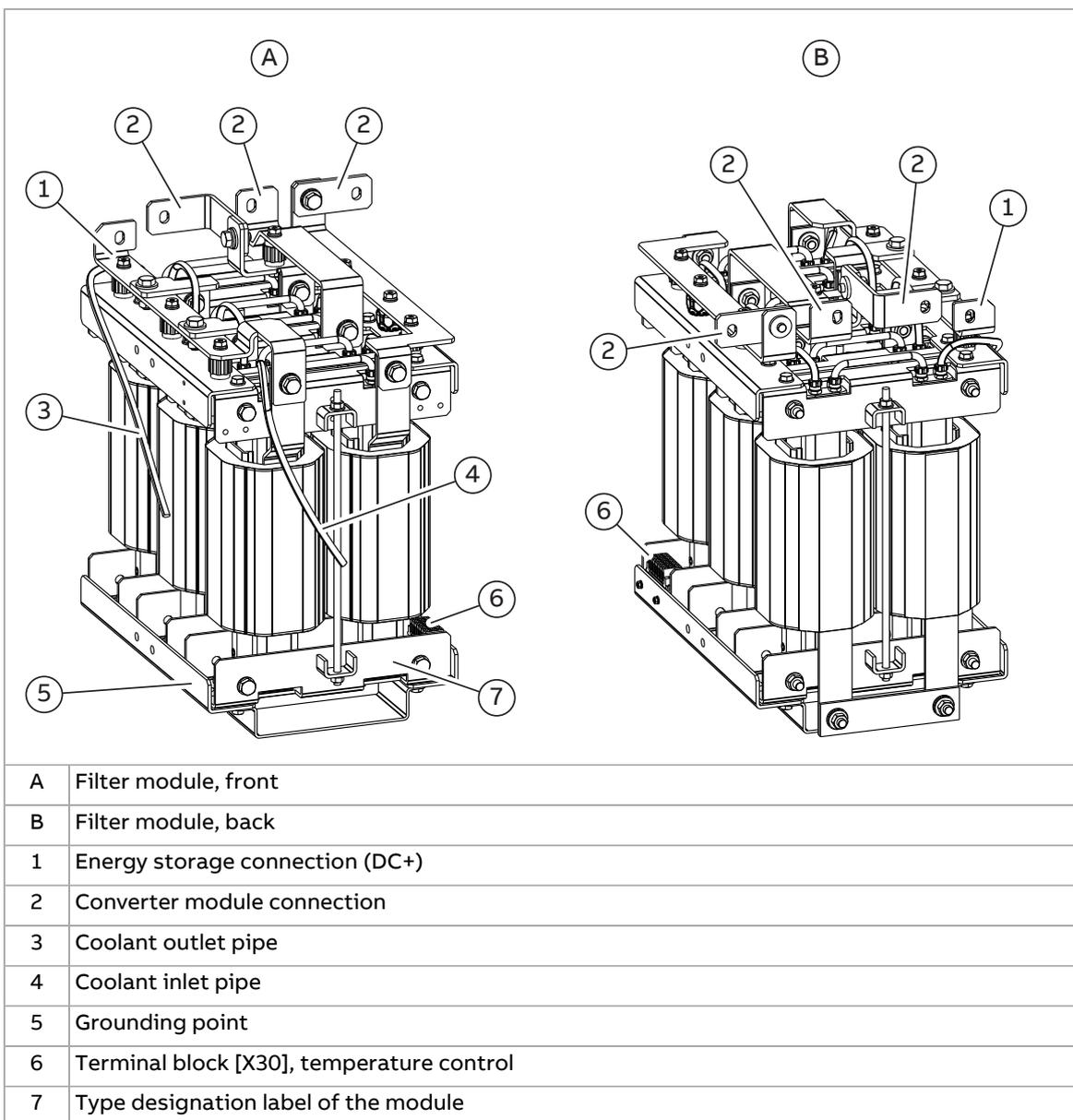
■ **BDCL filter module for frame R8i converter module**
