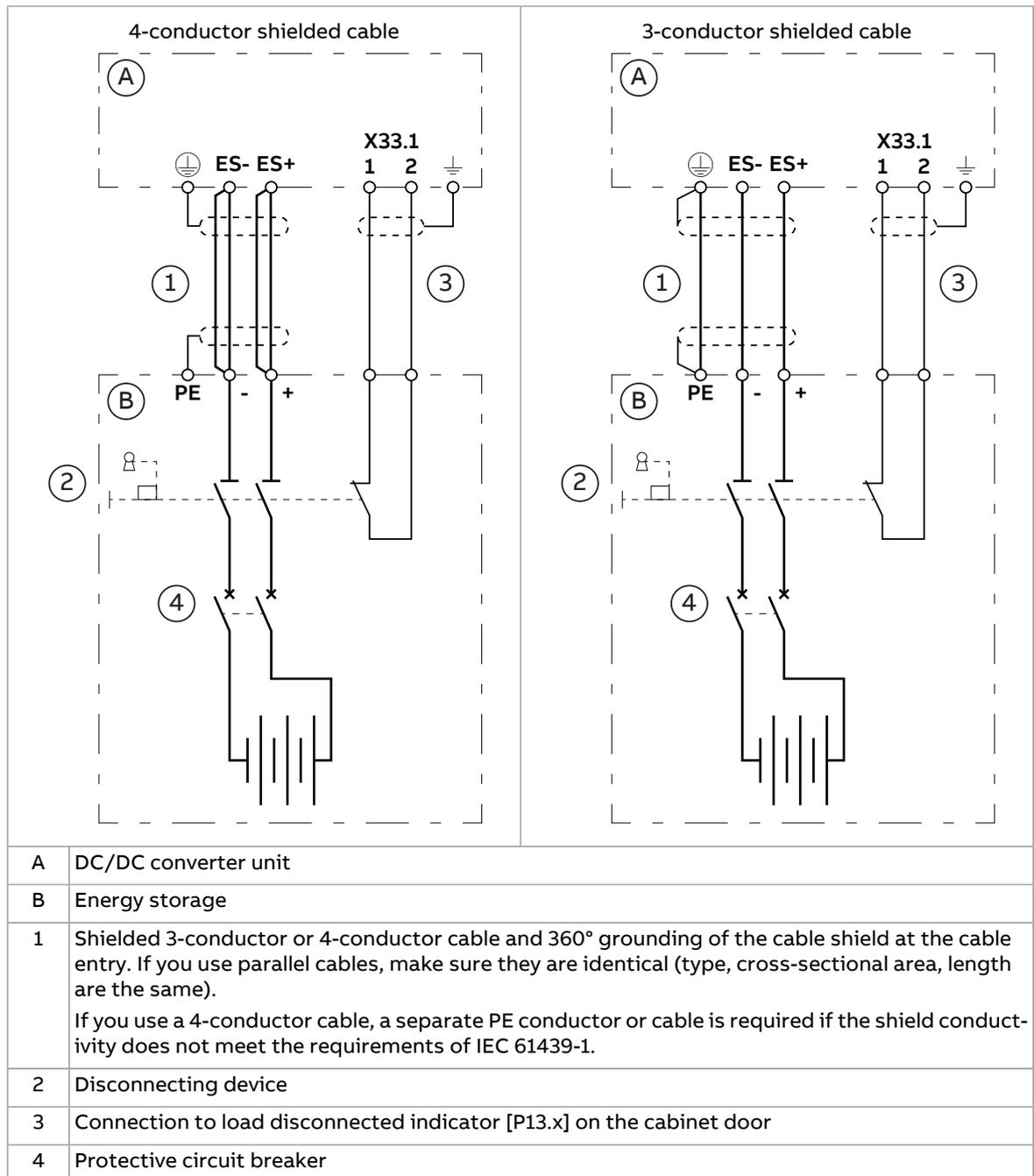
■ **Connection procedure of the energy storage cables**
