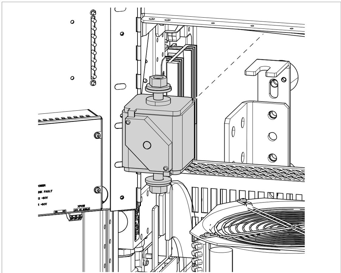
5. Remove the studs, nuts and washers from the fuse and install them to the new fuse. Make sure that you install the washers in the original order.
