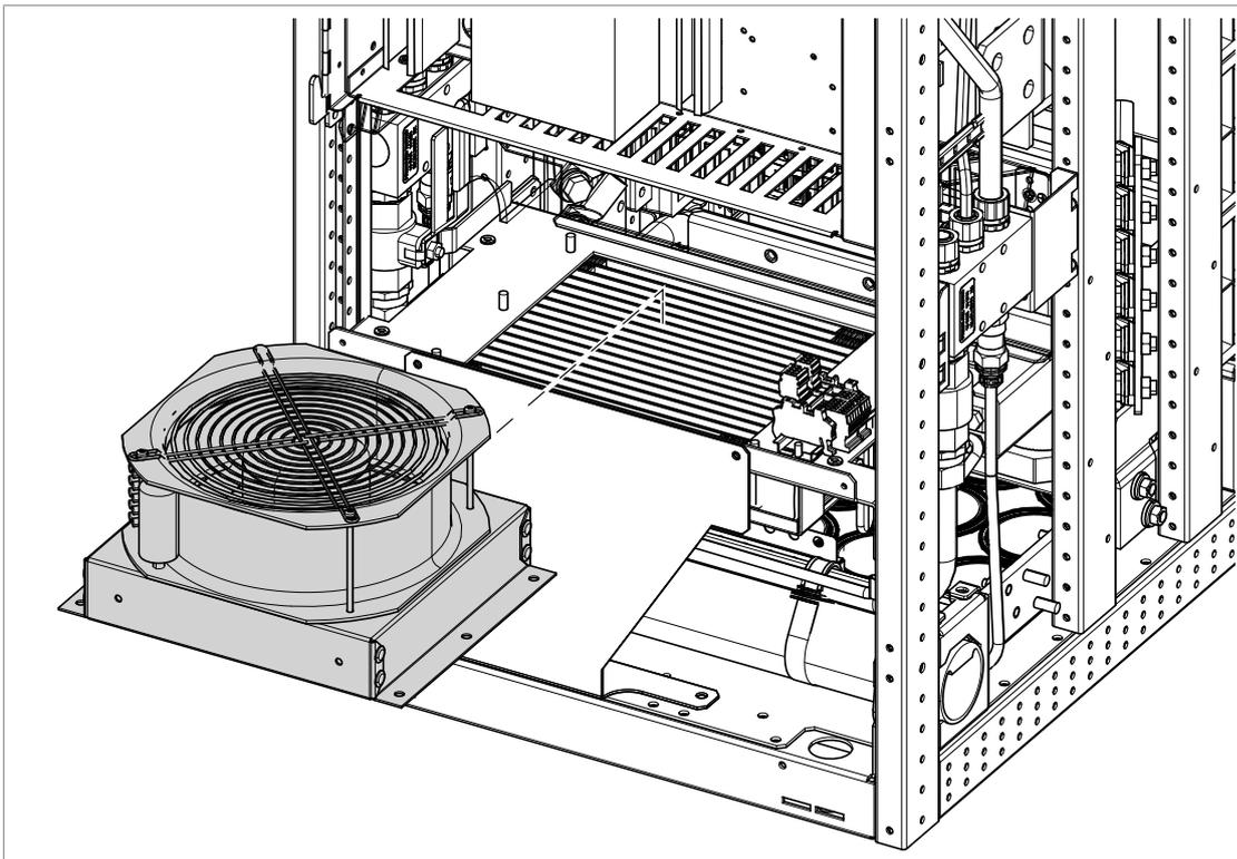
5. Remove the screws (a) that hold the finger guard (b) and fan (c) to the fan mounting plate (d).
