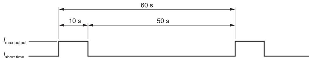
$P_{\text{short time}}$  Continuous output power allowing 10 s of  $I_{\text{max output}}$  every 60 s
