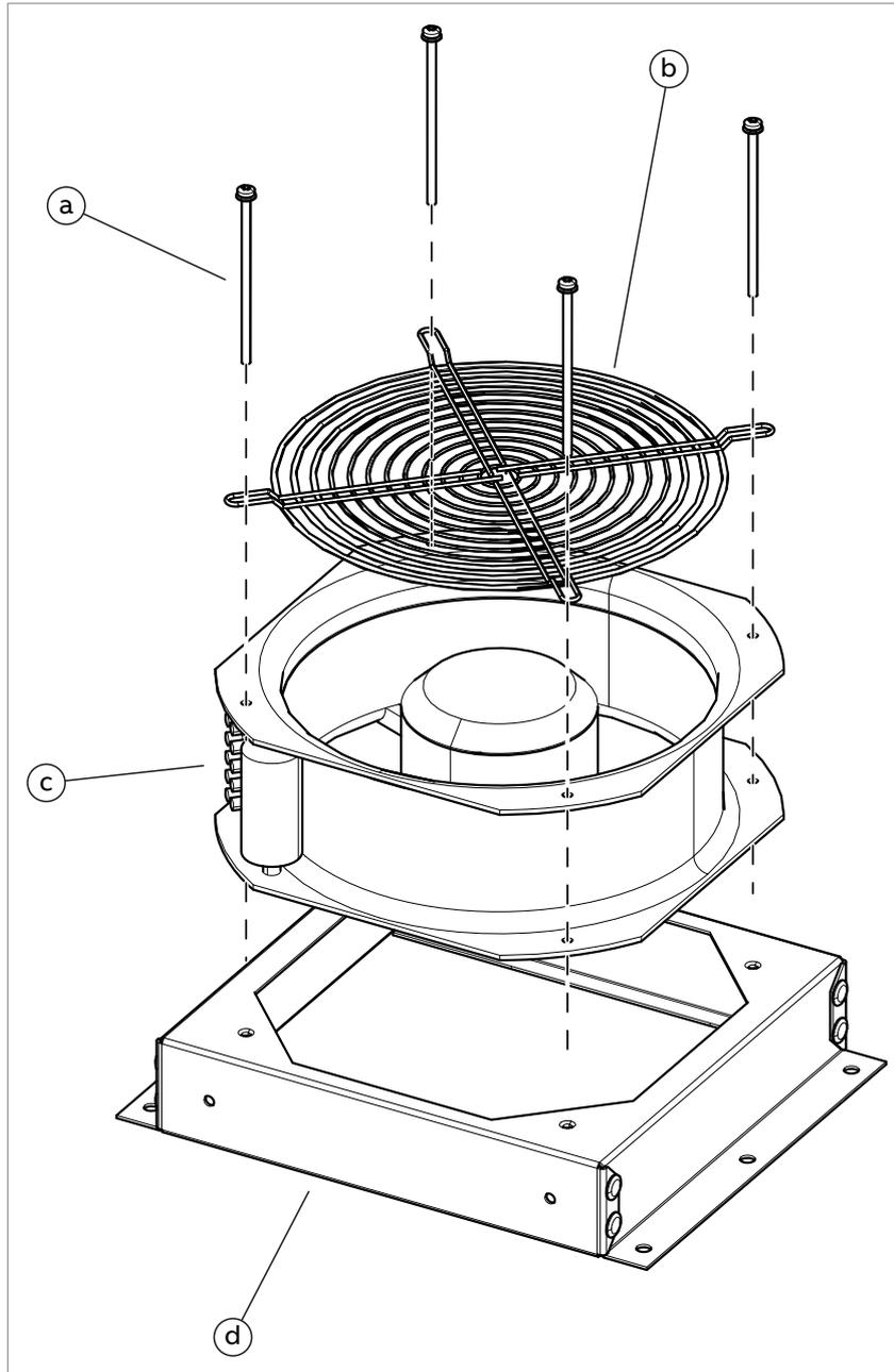
6. Assemble the fan assembly with a new fan. The airflow direction of the fan must be up.
