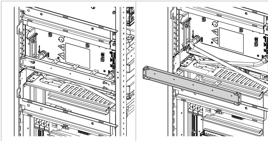
4. Disconnect the power and control cables from the module.
