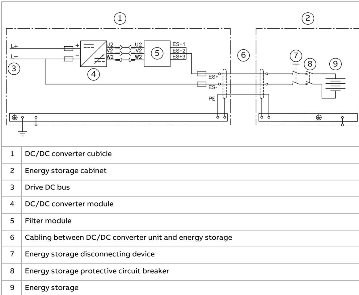
This figure shows a simplified main circuit diagram of a DC/DC converter with the DC switch-disconnector (option +F286) and charging circuit.
