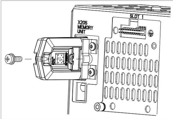
■ Replacing the memory unit (UCU-22...24)
