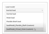
4. Select the uploaded custom FMU load model from the **Load model** drop-down and in the **Variables** section, map the FMU variables to the virtual drive variables. The available variables are listed in the table below:
