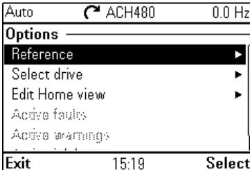
To go to the **Options** menu, press the **Options** softkey (
