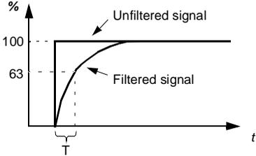
$O = I \times (1 - e^{-t/T})$ <p> <i>I</i> = filter input (step)<br/> <i>O</i> = filter output<br/> <i>t</i> = time<br/> <i>T</i> = filter time constant         </p> <p><b>Note:</b> The signal is also filtered due to the signal interface hardware (approximately 0.25 ms time constant). This cannot be changed by any parameter.</p> | 0.100 s               |
