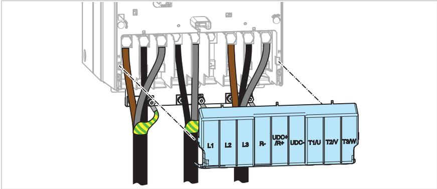
6. Secure the cables mechanically.
