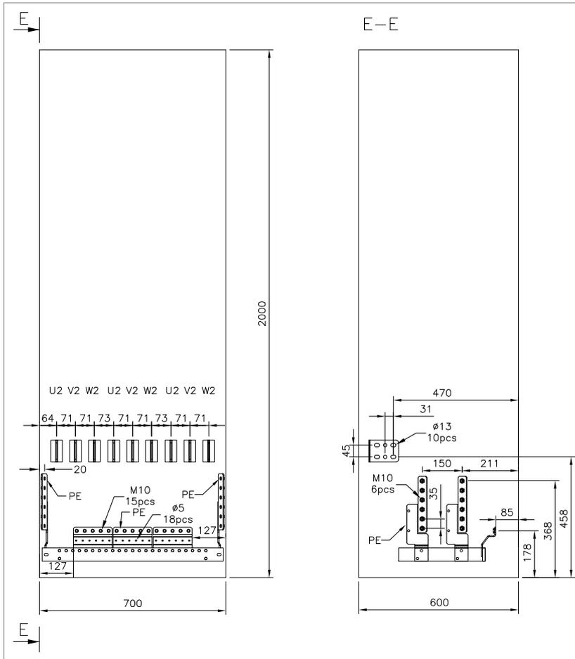
■ Units with common motor terminal cubicle (+H359)
