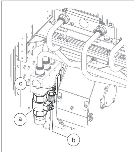
8. After the module has drained, disconnect the piping from the module.
