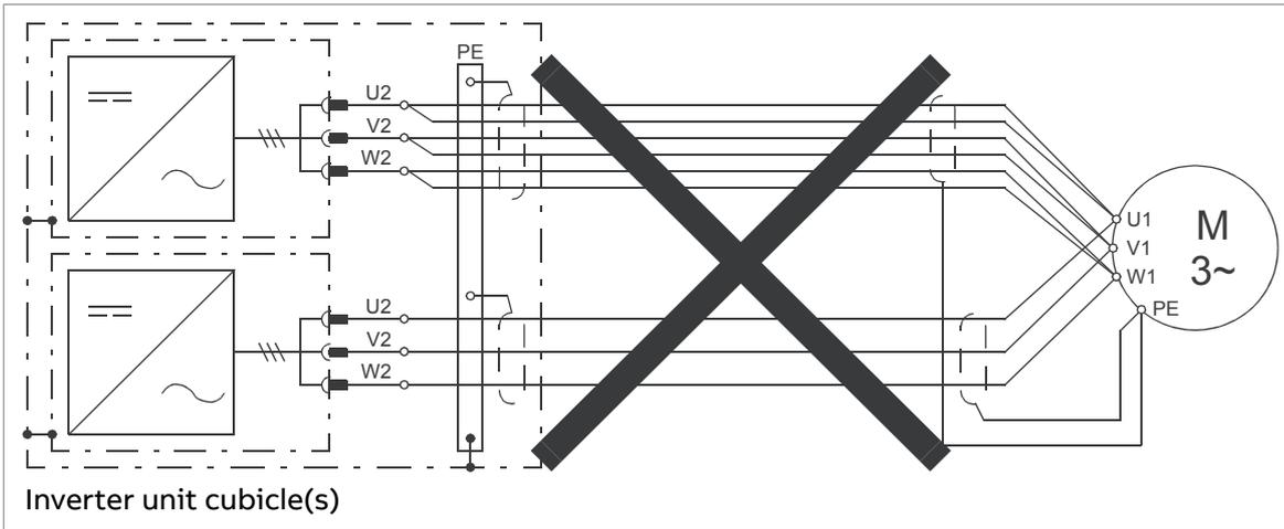
■ **Motor connection diagram (with option +H366)**
