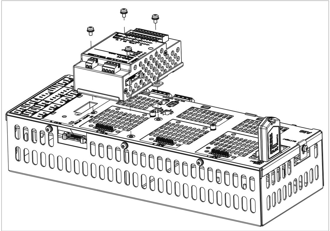
4. Tighten the FSO module electronics grounding screw.
