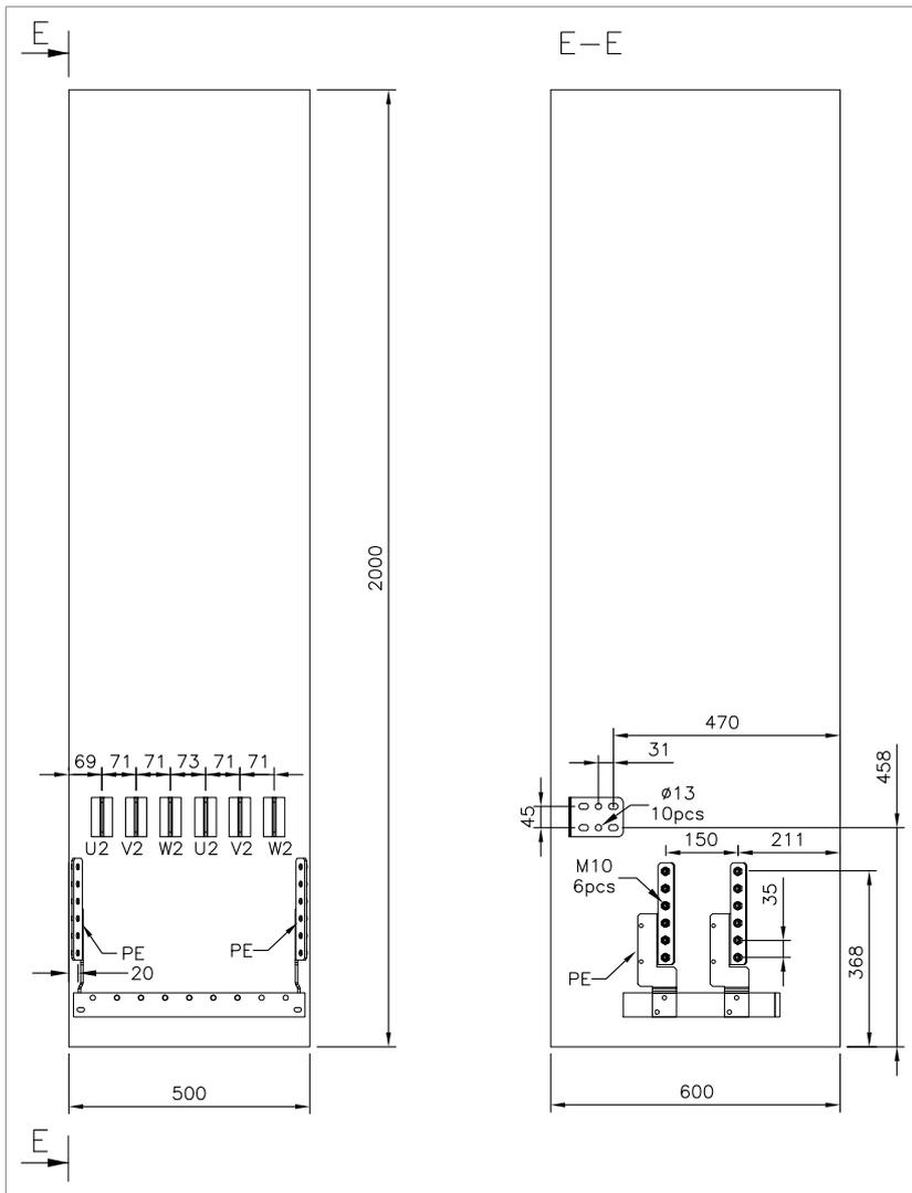
**Inverter module cubicle with three R8i modules, bottom cable exit**
