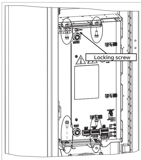
9. Pull the module carefully out onto the service platform.
