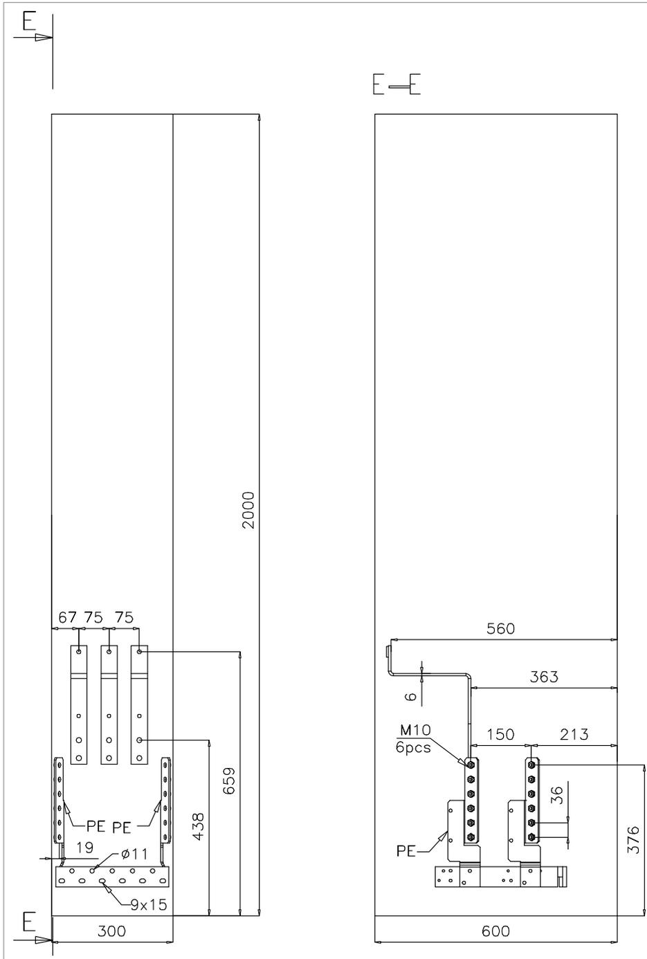
**Inverter module cubicle with two R7i modules, bottom cable exit**
