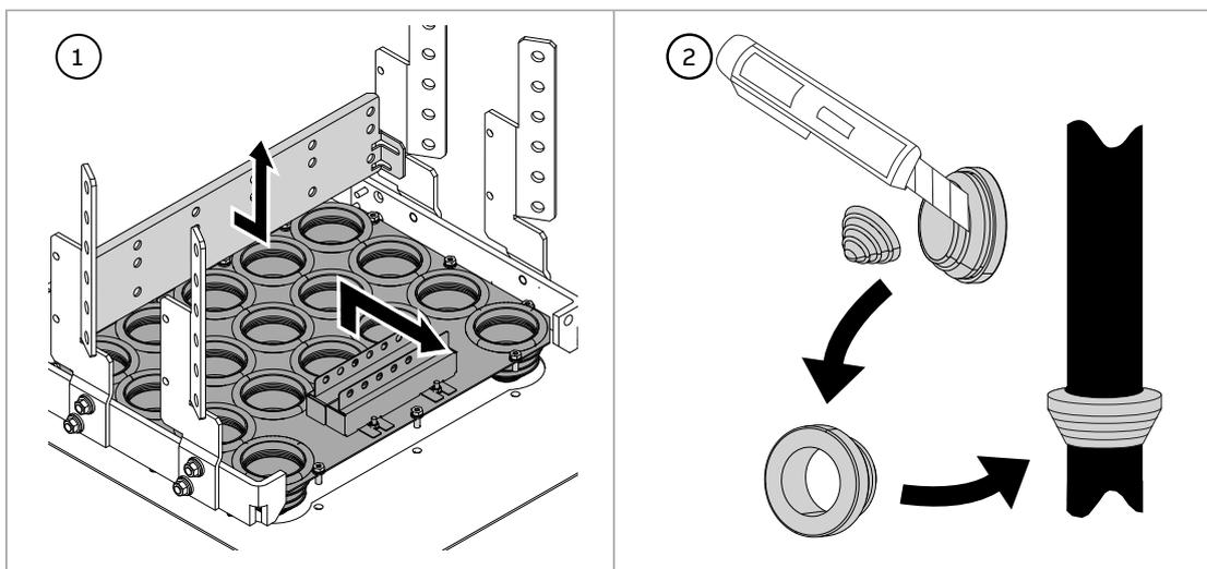
3. Lead the cables inside the cabinet through the cable entry plate. If there are several cables, use the rear 3 holes first.
