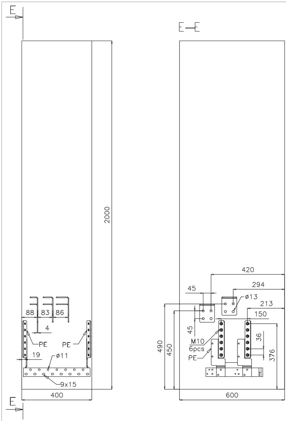
**Inverter module cubicle with one R8i module, bottom cable exit**
