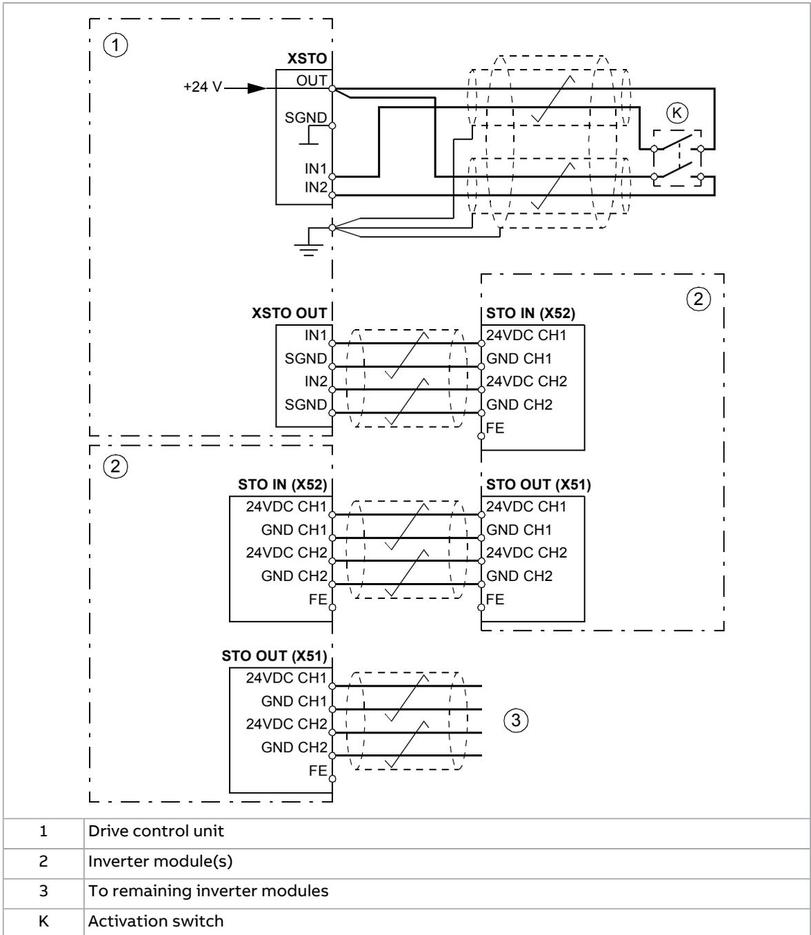
■ **Single-channel connection of activation switch**
