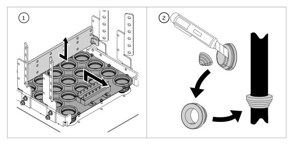
3. Lead the cables inside the cabinet through the cable entry plate. If there are several cables, use the rear 3 holes first.
