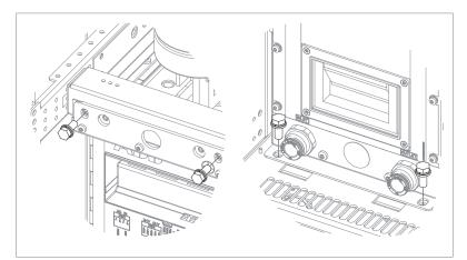
10. Pull the module carefully out onto the service platform. Keep the module secured to a hoist or equivalent to prevent the module from falling. For information on using the lifting device, see Converter module lifting device for drive cabinets hardware manual (3AXD50000210268 [English]).
