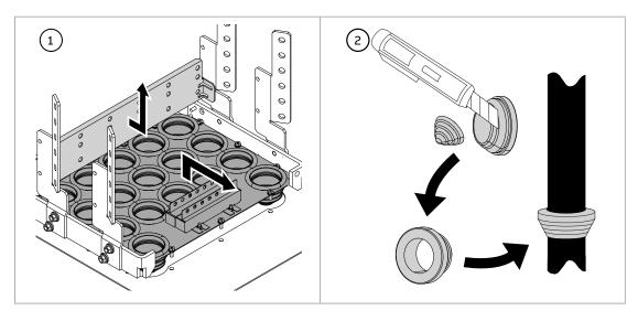
Lead the cables inside the cabinet through the cable entry plate. If there are several cables, use the rear 3 holes first.
