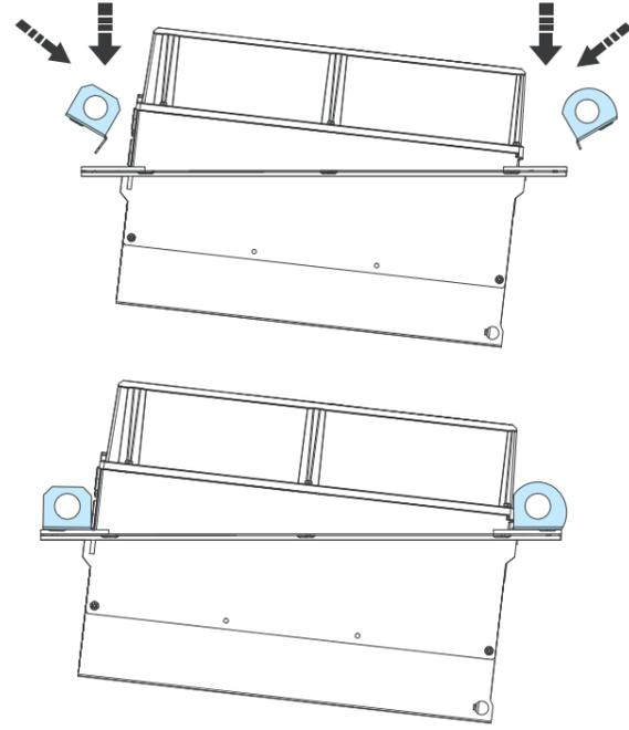
Drill holes for M6 Rivet or Kalei nuts. Consider the hole size for the nuts.
