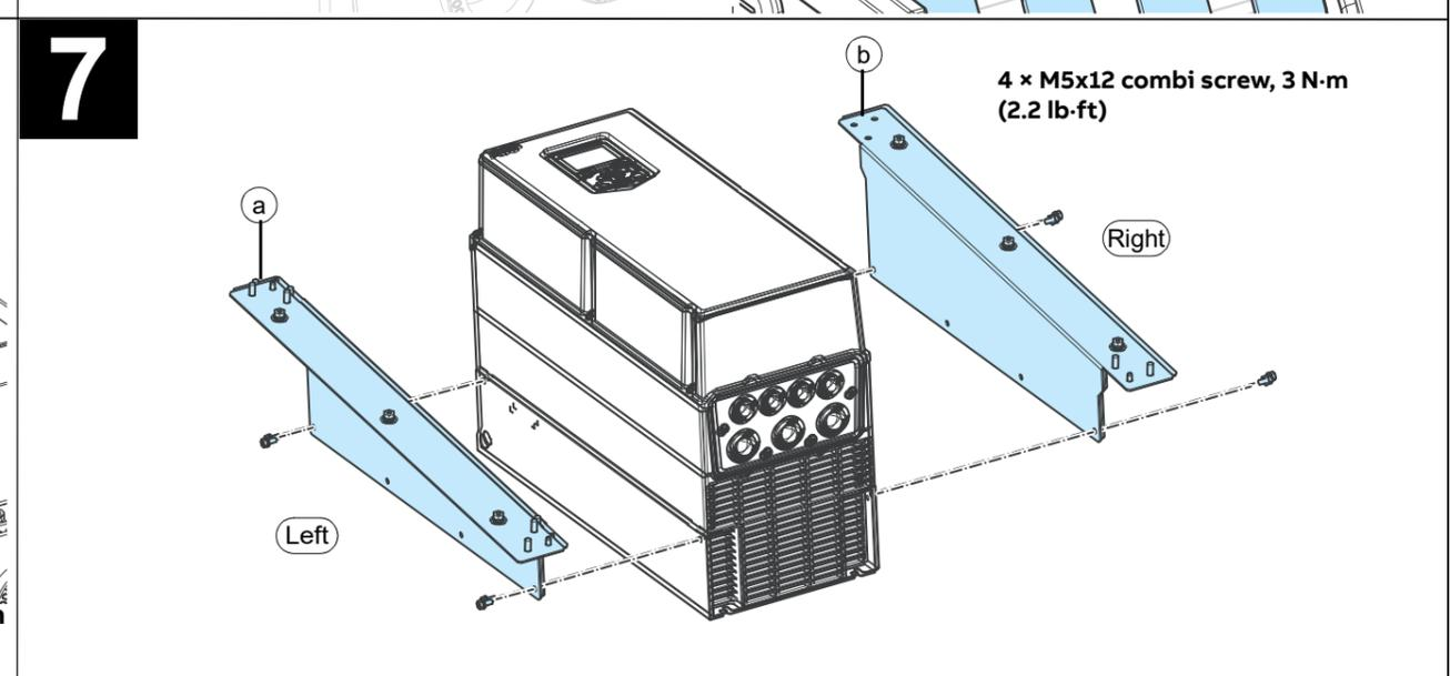
ACS880-11..., ACS880-31..., ACH580-31... and ACQ580-31...+C135 frame R3 flange mounting kit quick installation guide
