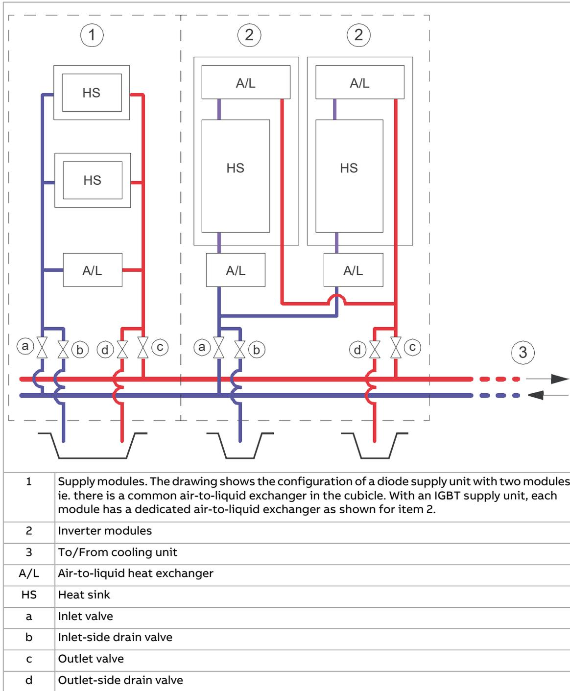
The coolant used with ACS880 liquid-cooled drive systems is Antifrogen® L 25% or 50% mixture. See [Coolant specification \(page 172\)](#).
