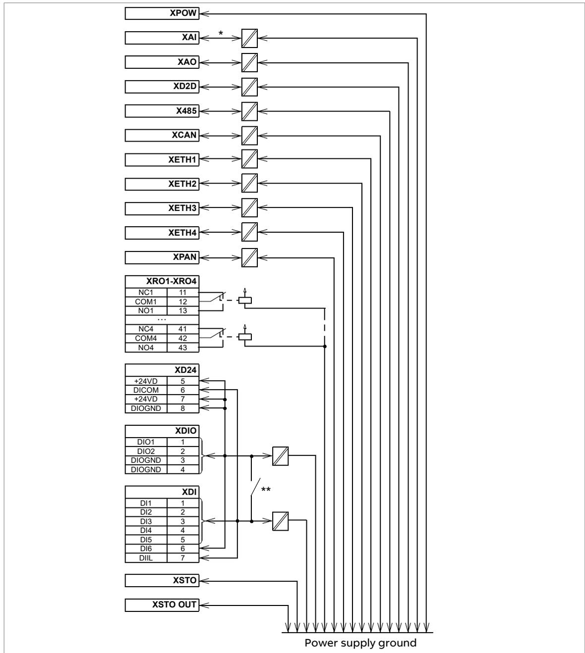
\*The maximum common mode voltage between each AI input and AGND is  $\pm 30$  V
