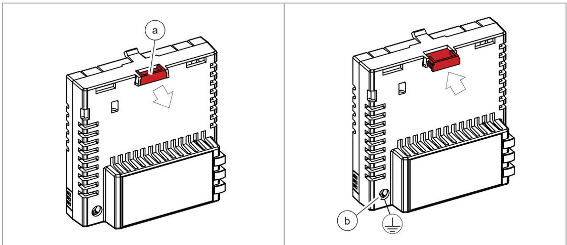
6. Connect the wiring to the module. Obey the instructions given in the documentation of the module.
