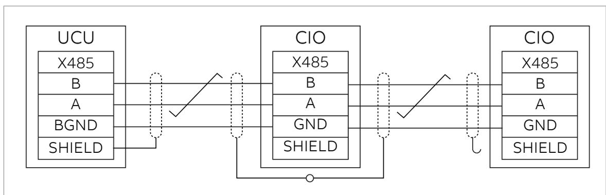
Terminate the I/O bus at its physical ends:
