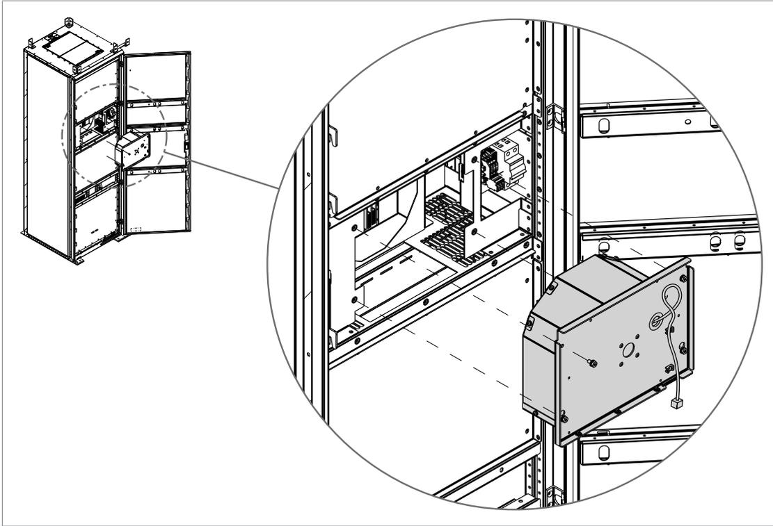
7. Disassemble the fan assembly as follows:
