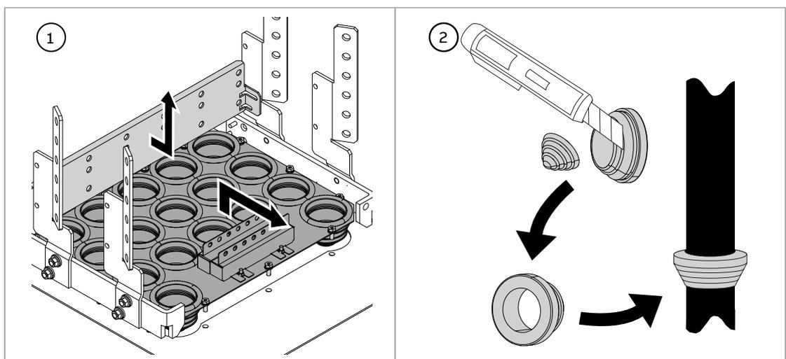
3. Put the cables inside the cabinet through the cable entry plate. If there are several cables, use the rear 3 holes first.
