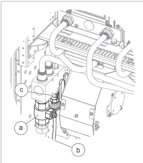
8. After the module has drained, disconnect the piping from the module.
