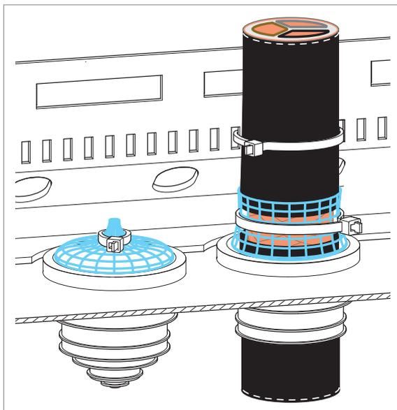
8. Connect the twisted shields of the cables to the PE busbar of the cabinet.
