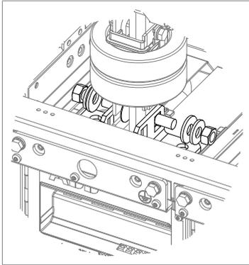
7. Close the inlet valve (a) and outlet valve (located on the right-hand side of the cubicle). Lead the drain hoses (b, on both sides of the cubicle) into a suitable container. Open the drain valves (c, on both sides of the cubicle). This will drain all modules in the cubicle.
