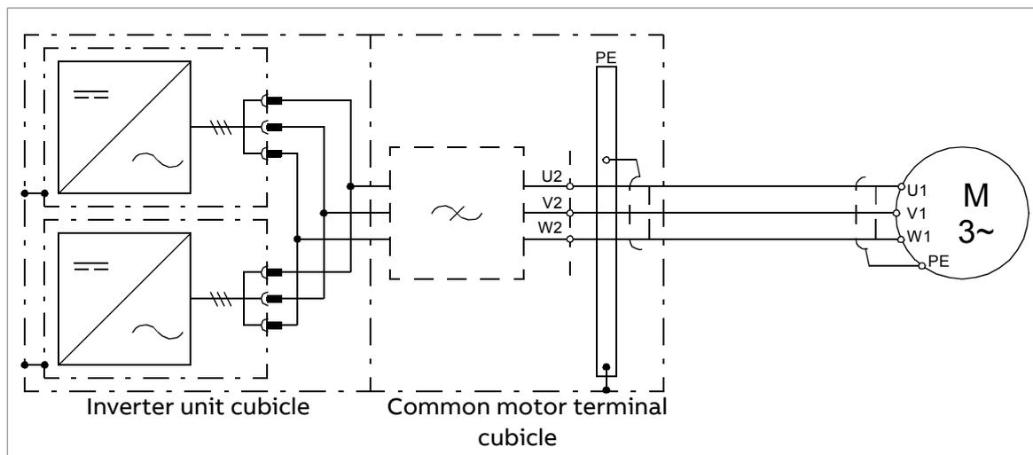
The recommended cable types are given in the technical data.
