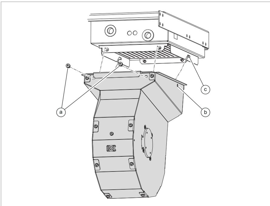
17. Install the lower front mounting plate. Connect the wiring to the components on the mounting plate.
