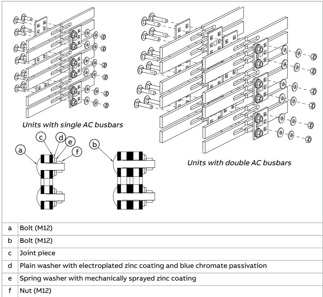
**WARNING!** Make sure that you install the washers in the correct order, as shown in the illustration. For example, placing an unpassivated zinc-coated spring washer directly against the joint piece will cause corrosion.
