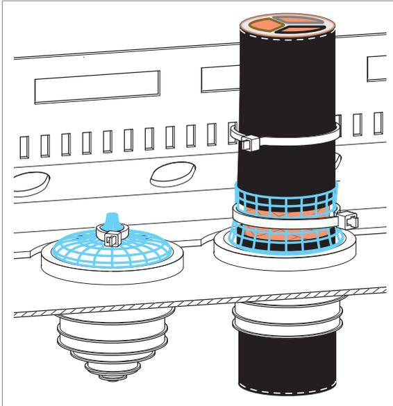
13. Connect the twisted shields of the cables to the PE busbar of the cabinet.
