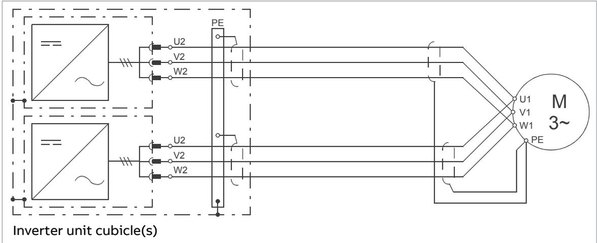
The recommended cable types are given in the technical data.
