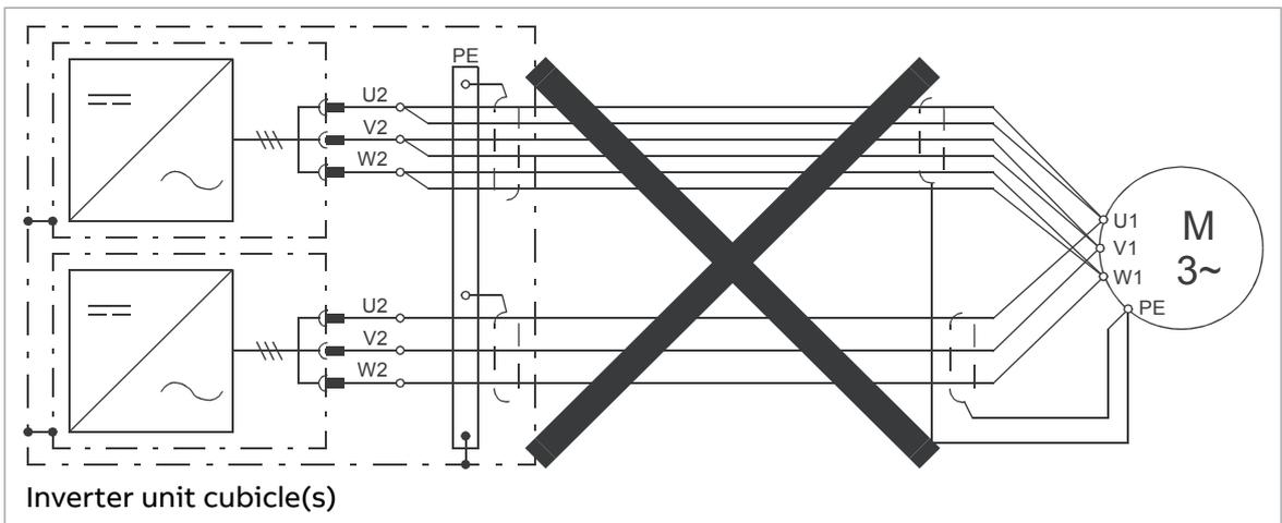
■ **Motor connection diagram (with option +H366)**
