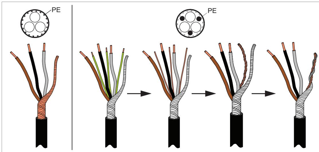
6. Remove rubber grommets from the cable entries for the cables to be connected. Cut adequate holes into the rubber grommets. Slide the grommets onto the cables. Slide the cables into the cubicle through the conductive sleeves and attach the grommets to the holes.
