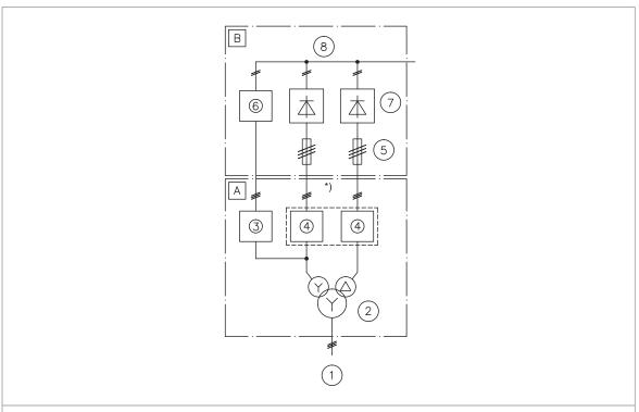
**Note:** \*) Each module must have its own input AC cable with the minimum length of 5 meters. Use symmetrical supply cabling to ensure equal current sharing between parallel diode bridges.
