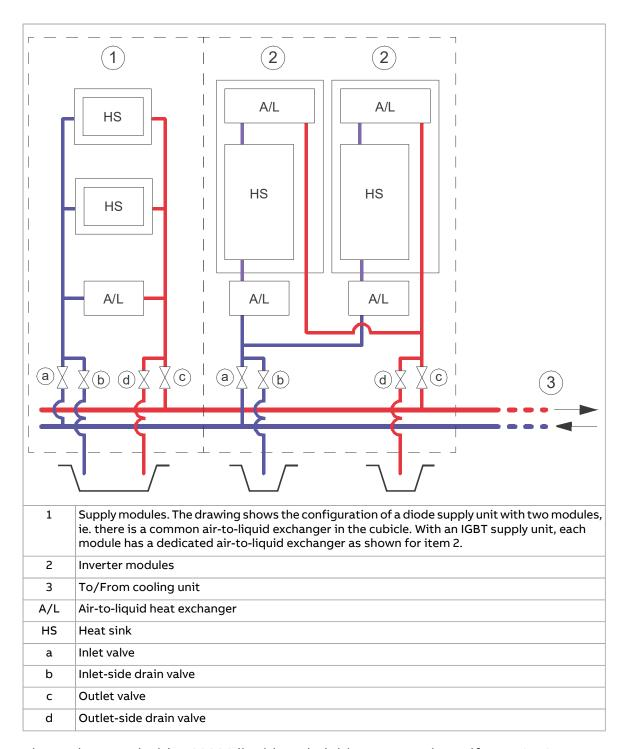
The coolant used with ACS880 liquid-cooled drive systems is Antifrogen® L 25% or 50% mixture. See Coolant specification (page 114).
