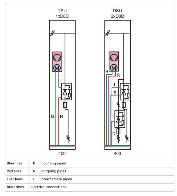
In diode supply unit cabinets, flow restrictors are used in both manifolds.
