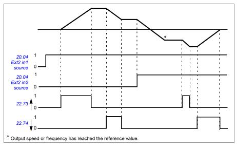
The running direction can be changed with parameter 20.04 Ext1 in2 source. See the following example.
