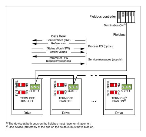
The AC500 PLC has a free version library called 'PS553 drives' which help user to communicate and control between PLC and drives easily.
