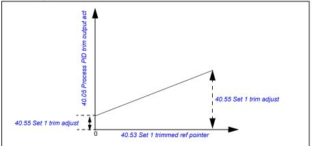
**Note:** In the above graph, it is assumed that the PID output is limited/stable at 100. This is for understanding purpose only. In real case scenario, PID output can vary based on the setpoint and actual.
