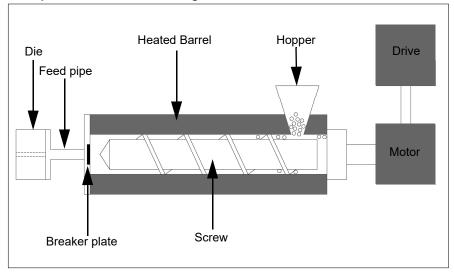
Basic plastic extrusion block diagram
