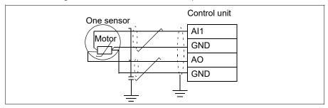
Leave the sensor end of the cable shield unconnected.
