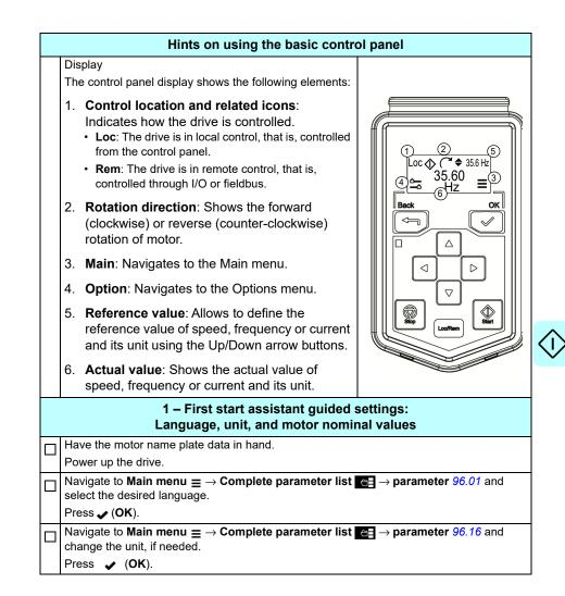
Refer to the motor nameplate for the following nominal value settings of the motor. Enter the values <u>exactly</u> as shown on the motor nameplate.
