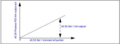
**Note:** In the above graph, it is assumed that the PID output is limited/stable at 100. This is for understanding purpose only. In real case scenario, PID output can vary based on the setpoint and actual.
