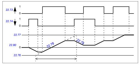
The following example shows the behavior of the motor potentiometer value.
