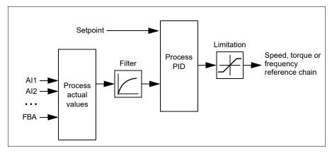
**Note:** Process PID control is available only in external control location EXT2. See section *Local control vs. external control* (page 33).
