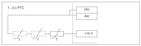
**Note:** RIIO-01 or BIO-01 is required for the analog input. By default, RIIO-01 is provided with the ACS560 drives.
