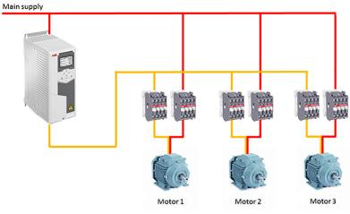
Example of a 3-pump constant pressure water supply application:
