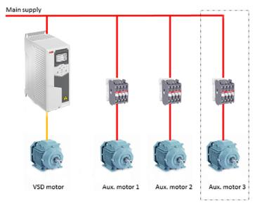
Example of a 3-pump constant pressure water supply application:
