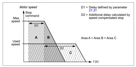
Speed compensation can be restricted to forward or reverse rotating direction.
