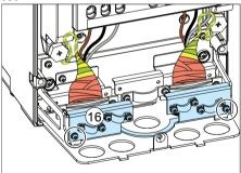
17. Put the (so far) unused rubber grommets to the holes in the lead-through plate, unless you will continue with installing the control cables.
