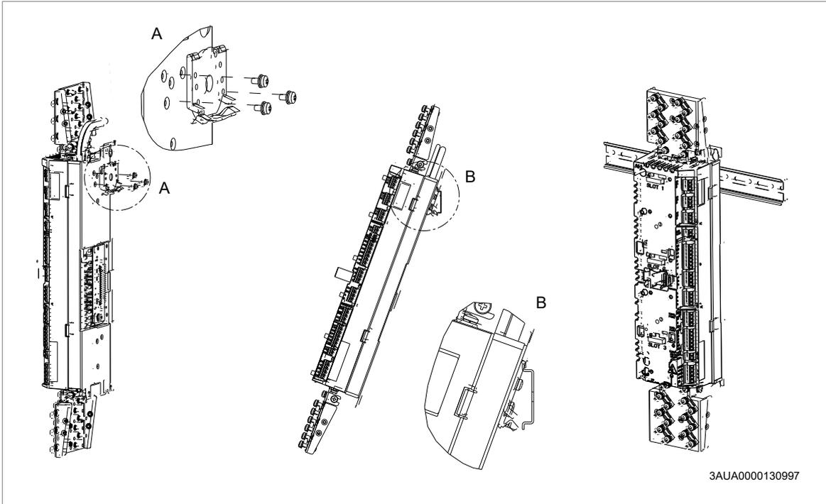
■ **Attaching the external control unit horizontally on a DIN rail**
