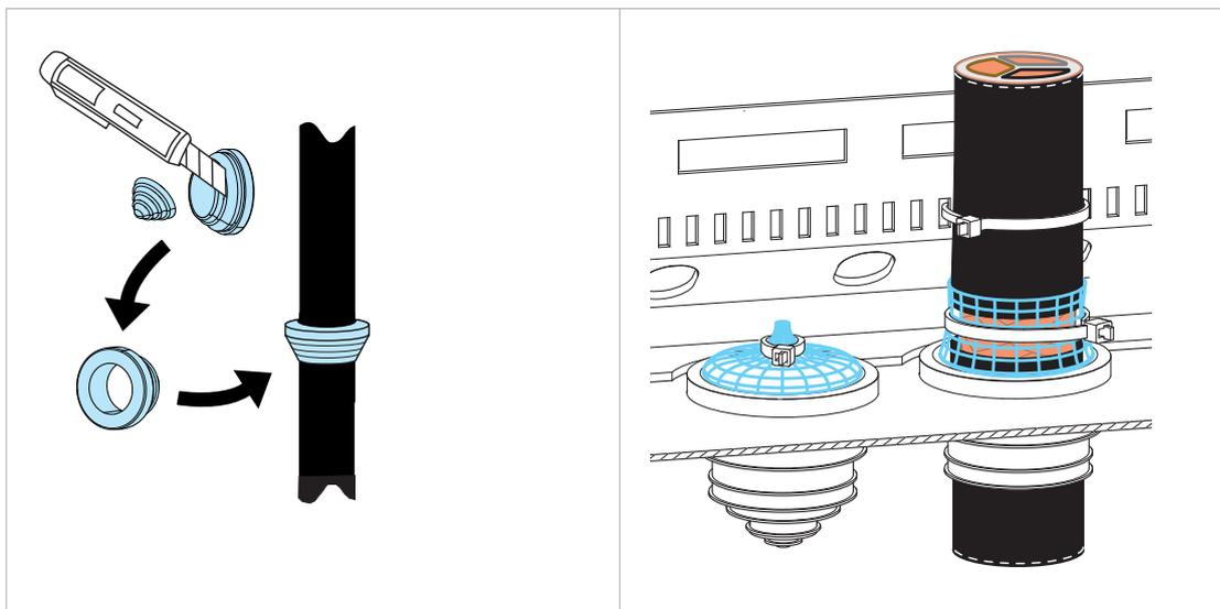
■ **Power cable connection procedure**
