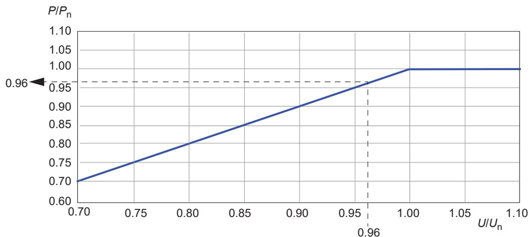
**Example 1:**  $P_n$  for ACS880-34-430A-7 is 400 kW. The input voltage ( $U$ ) is 660 V.  $\rightarrow U/U_n = 660 \text{ V} / 690 \text{ V} = 0.96$   $\rightarrow P/P_n = 0.96$   $\rightarrow$  The derated power  $P = 0.96 \times 400 \text{ kW} = 384 \text{ kW}$ .
