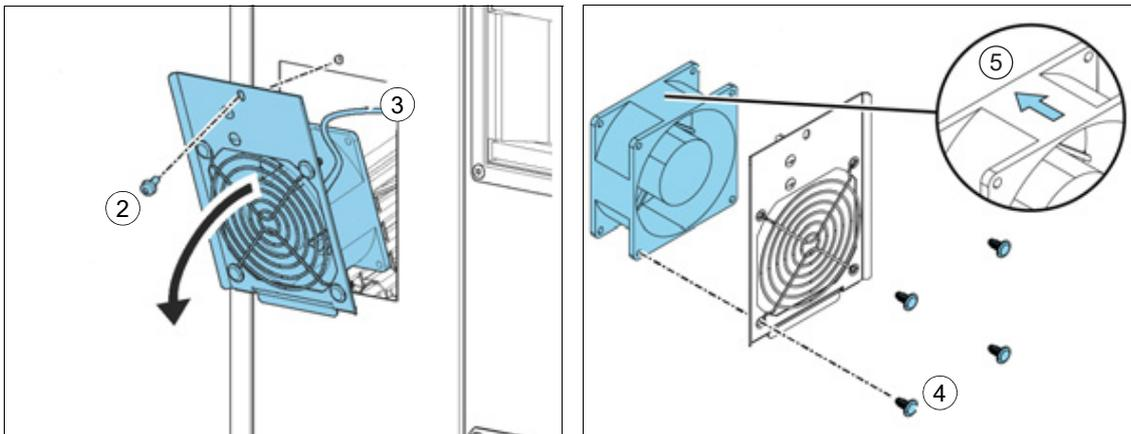
**Fan at the bottom of the circuit board compartment:**
