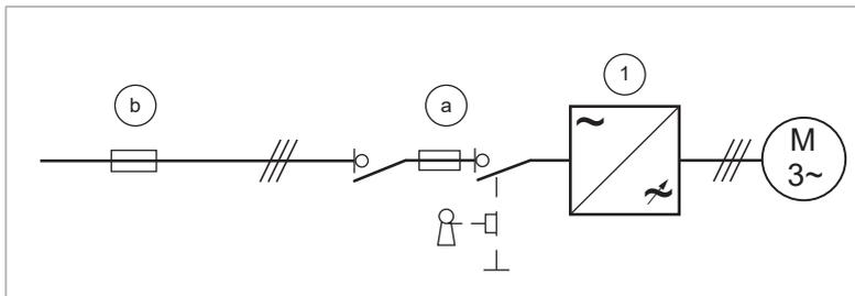
Select the fuses or the circuit breaker according to local regulations for the input cable protection. Select the fuses for the drive according to the instructions given in the technical data. The fuses for the drive protection will restrict drive damage and prevent damage to adjoining equipment in case of a short-circuit inside the drive.
