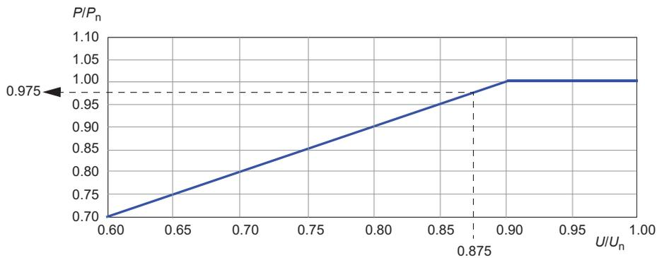
**Example 1:**  $P_n$  for ACS880-34-650A-3 is 355 kW. The input voltage ( $U$ ) is 350 V.  $\rightarrow U/U_n = 350 \text{ V} / 400 \text{ V} = 0.875$ .  $\rightarrow P/P_n = 0.975$   $\rightarrow$  The derated power  $P = 0.975 \times 355 \text{ kW} = 346 \text{ kW}$ .
