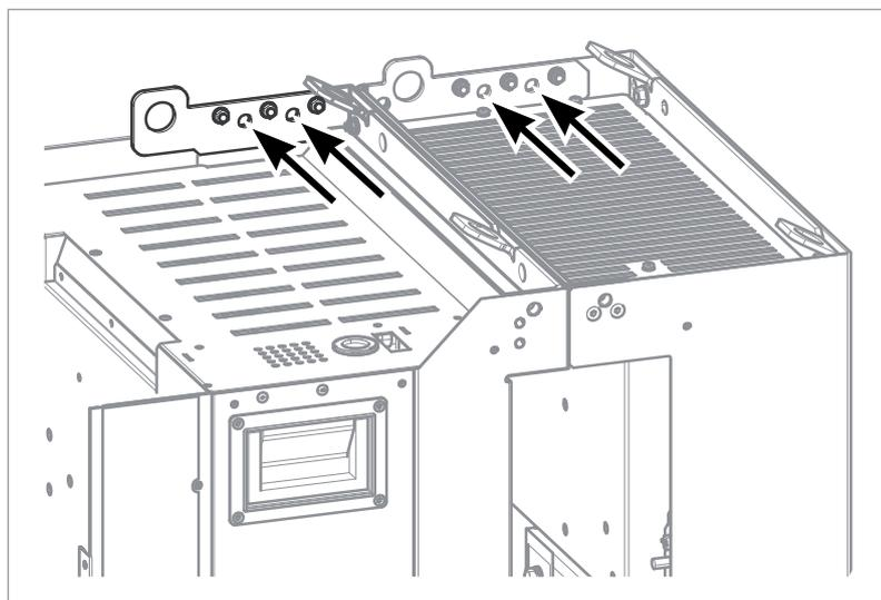
You can attach the modules to Rittal VX25 enclosure with the mounting brackets delivered with the drive, see *Step-by-step drawings* for an installation example of standard drive configuration in Rittal VX25 800 mm wide enclosure (Page 257).
