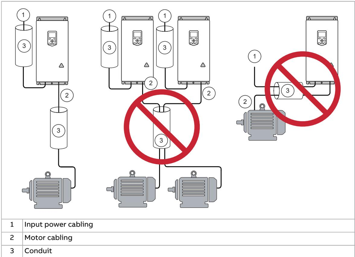
■ **Continuous motor cable shield/conduit or enclosure for equipment on the motor cable**
