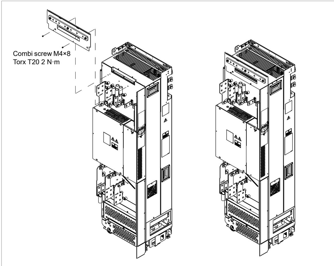
Connect the input power cable connection terminals as shown in Step-by-step drawings for an installation example of standard drive configuration in Rittal VX25 800 mm wide enclosure (Page 257).
