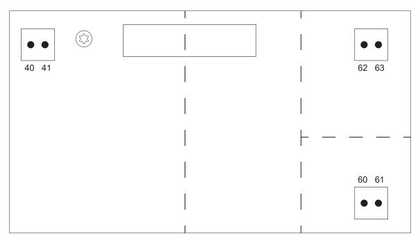
Dashed line: reinforced insulation (IEC 61800-5-1).
