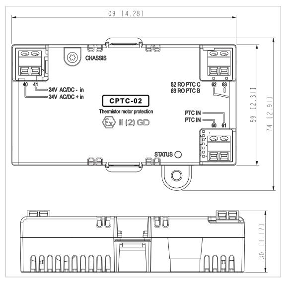
Installation: Into Option slot 2 on the drive control unit
