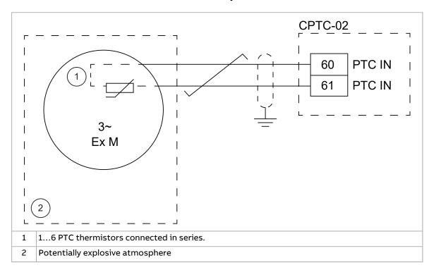
The PTC input is reinforced/double insulated. If the motor part of the PTC thermistor and wiring are reinforced/double insulated, voltages on the PTC wiring are within SELV limits.
