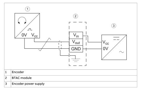
When using a 24 V encoder, it is possible to supply power to the encoder and BTAC module from the 24 V DC auxiliary power output of the drive. If you supply power from the auxiliary power output, make sure that you do not exceed the maximum load capacity.
