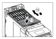
Replacing the cooling fan, frame R4
