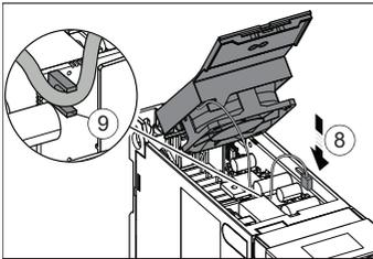
10. Carefully put the fan cover into position in the drive. Make sure that the fan power cable is routed correctly.
