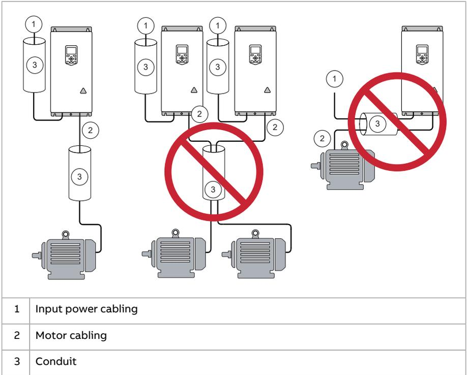
■ **Continuous motor cable shield/conduit and metal enclosure for equipment on the motor cable**
