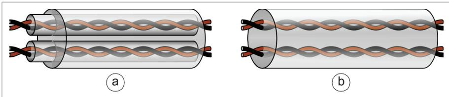
■ **Signals in separate cables**
