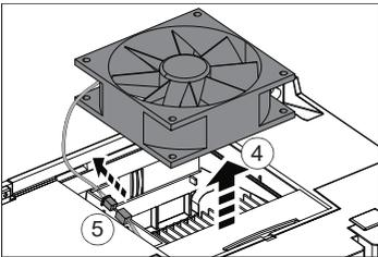
6. Replace the fan. The arrow indicating the air flow direction must point up.
