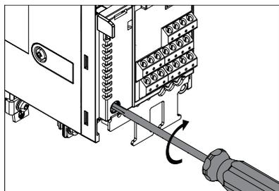
6. If the option module has a locking tab, push it down until it locks.
