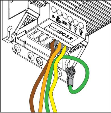
9. If you use a brake resistor, connect the brake resistor conductors to terminals R- and UDC+.
