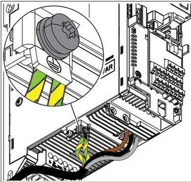
12. Connect the protective earth (ground) conductor(s) of the input power cable to the grounding terminal.
