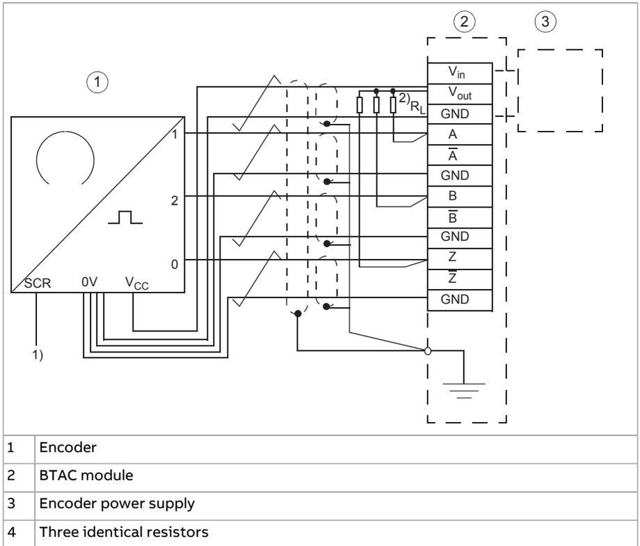
The resistor size depends on the encoder power supply  $V_{in} = V_{OUT}$ :
