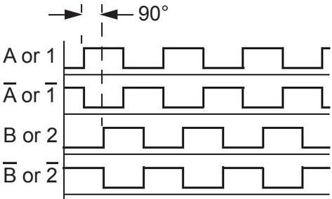
The diagram shows normal phasing: Pulse A leads (rises earlier than) pulse B.
