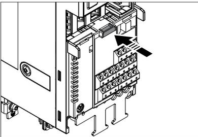
7. Connect the control cables. See the control cable connection instructions.
