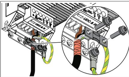
6. Twist the motor cable shield into a bundle, mark it with yellow-green insulation tape, install a cable lug, and connect it to the grounding terminal.
