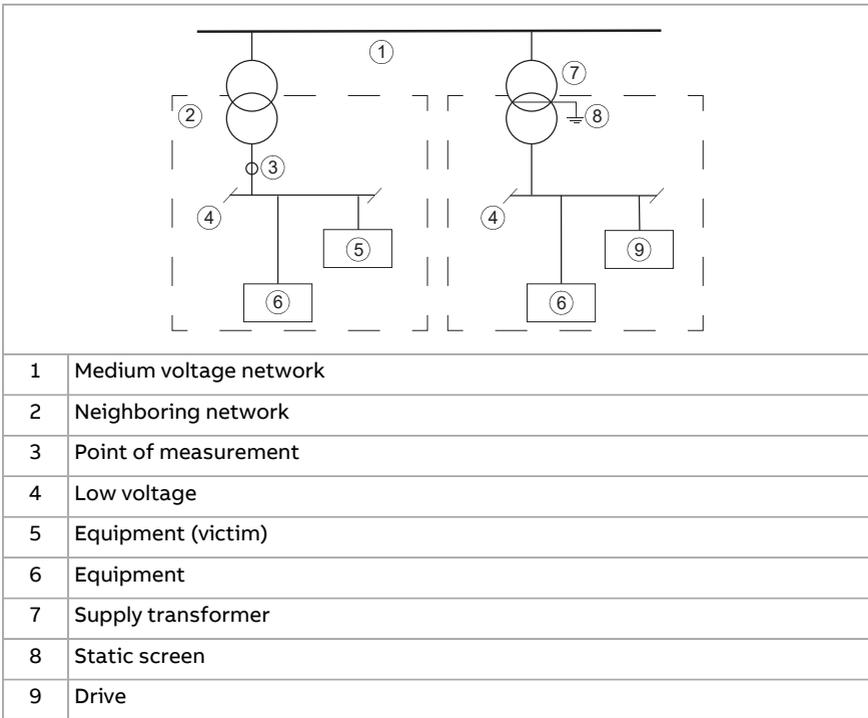
2. An EMC plan for preventing disturbances is drawn up for the installation. A template is available in [Technical guide No. 3 EMC compliant installation and configuration for a power drive system \(3AFE61348280 \[English\]\)](#).
