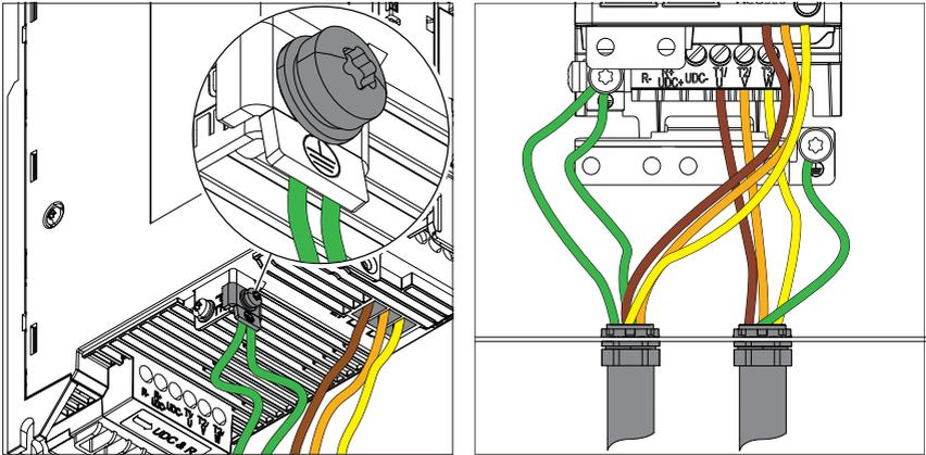
13. Connect the other ends of the conductors.
