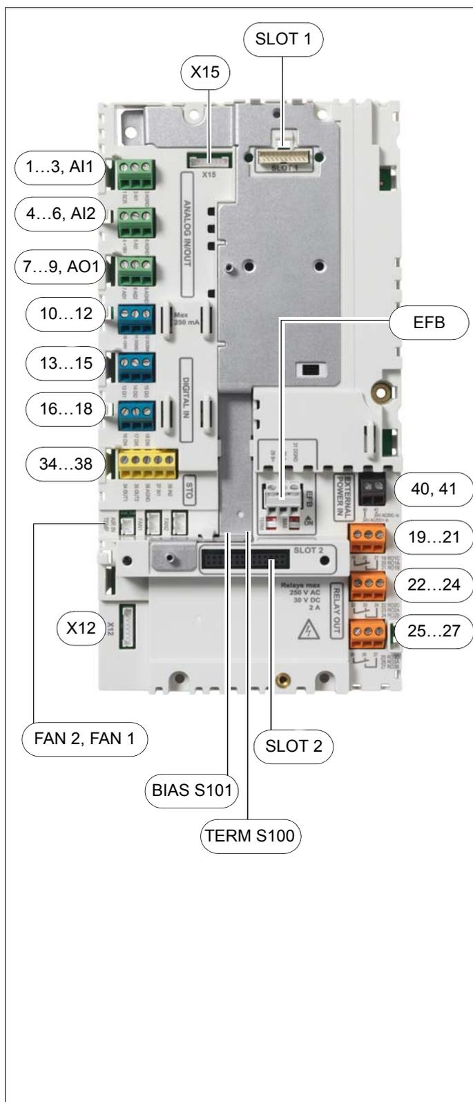
The diagram shows the physical terminal block of the converter. Labels on the left side include: 1...3, AI1; 4...6, AI2; 7...9, AO1; 10...12; 13...15; 16...18; 34...38; X12; FAN 2, FAN 1; BIAS S101; and TERM S100. Labels on the right side include: X15; EFB; 40, 41; 19...21; 22...24; 25...27; and SLOT 2. The terminal block itself has sections for ANALOG IN/OUT, DIGITAL IN, STO, EXTERNAL POWER IN, and RELAY OUT.
