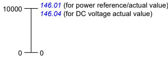
The scaled references are shown by parameters [103.05 FB A reference 1](#) and [103.06 FB A reference 2](#).
