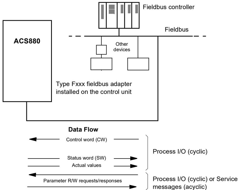
The brake unit can be set to receive its control information through the fieldbus interface, or the control can be distributed between the fieldbus interface and other available sources such as digital and analog inputs.
