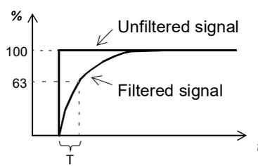
$O = I \times (1 - e^{-t/T})$ <p>I = filter input (step)<br/> O = filter output<br/> t = time<br/> T = filter time constant</p> <p><b>Note:</b> The signal is also filtered due to the signal interface hardware. See parameter <i>114.31 AI1 filter gain</i>.</p> | 0.040 s              |
