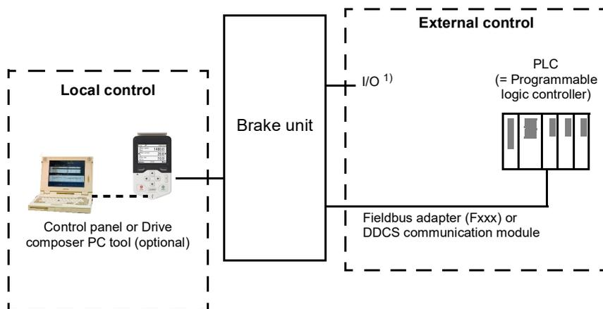
1) Extra inputs/outputs can be added by installing optional I/O extension modules (FIO-xx) in the option slots of the control unit.
