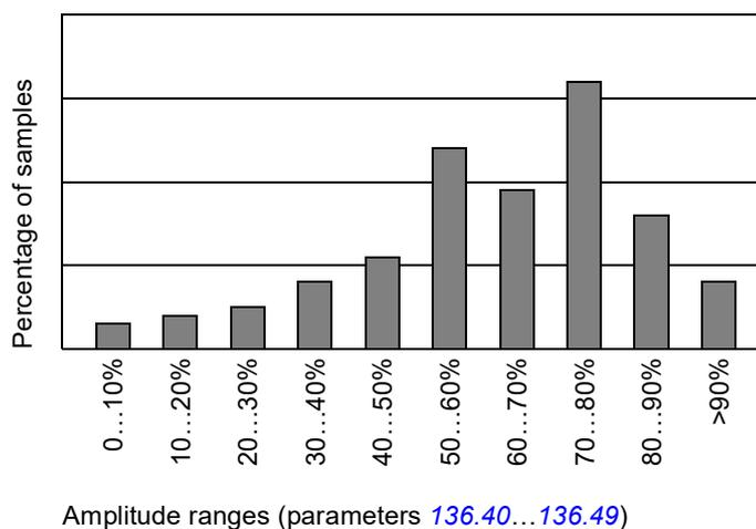
Amplitude logger 1 is fixed to AC current ([101.21 Converter current %](#)), and cannot be reset. With amplitude logger 1, 100% corresponds to the maximum current of the converter. The measured current is logged continuously. The distribution of samples is shown by parameters [136.20...136.29](#).
