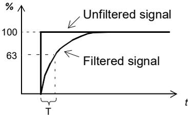
$O = I \times (1 - e^{-t/T})$ <p>I = filter input (step)<br/>O = filter output<br/>t = time<br/>T = filter time constant</p> <p><b>Note:</b> The signal is also filtered due to the signal interface hardware. See parameter <i>114.61 AI3 filter gain</i>.</p> | 0.100 s          |
