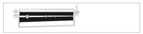
6. If more than one cable go through a grommet, seal the grommet by applying Loctite 5221 (catalogue number 25551) inside the grommet.
