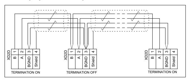
The following diagram shows the wiring of the drive-to-drive link.
