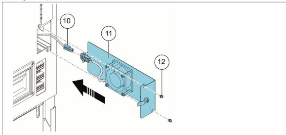
12. Install and tighten the two screws.
