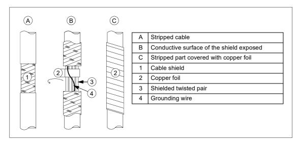
**Note for top entry of cables:** When each cable has its own rubber grommet, sufficient IP and EMC protection can be achieved. However, if very many control cables come to one cabinet, plan the installation beforehand as follows:
